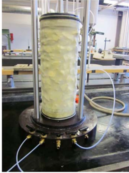
Figure 3.2. Specimen once the mold is removed
