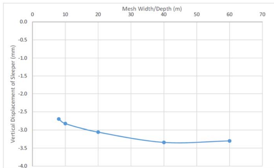
Figure 4.8. Mesh Size's Influence on Vertical Displacement of Sleeper
