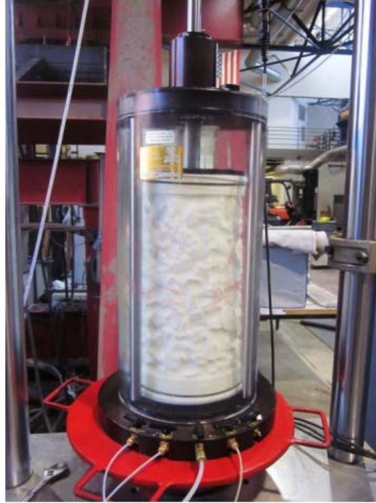
Figure 3.3. Specimen fully set up with de-aired water
