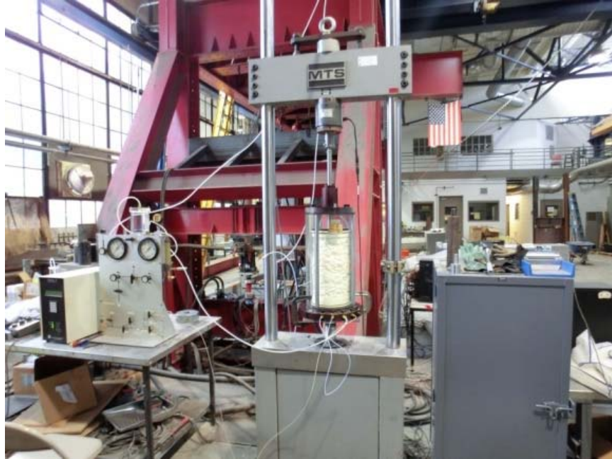
Figure 3.4. Triaxial set up with console and FlowTrac controller in MTS Machine
