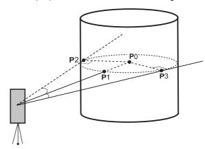
• The azimuth angle of the center of the column is 1/2 of total azimuth angle of circumscription points (P2) and (P3).
