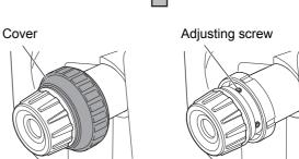
5. Turn the 4 adjusting screws of the optical plummet to adjust the remaining half of the deviation using hexagonal wrench (1.3 mm) as shown below. When the survey point is on the lower (upper) part of the illustration:
