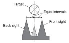
**Vertical direction**: a position where you can see the tops of the front sight and back sight at the same height of the target's center.
