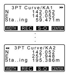
9. In the screens for the KA1 point, KE1 point, KE2 point, and KA point that have been found, press **[CENTER]** to move to centerline peg settings.
