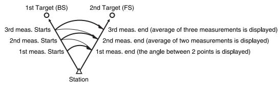
• The maximum number of angle measurements that can be made is 10.
