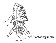
Looking through the optical plummet eyepiece, turn the optical plummet eyepiece to focus on the reticle.
