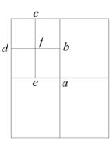
**22.18** The quarter-section corner between Secs. 15 and 16 is found to be 39.86 ch from the corner common to Secs. 9, 10, 15, and 16. Where should the quarter-quarter-section corner be set along this line in subdividing Sec. 15?
