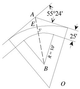
Tabulate all data required to lay out by deflection angles and incremental chords, at the indicated stationing, for the circular curves of Problems 24.20 and 24.21.
