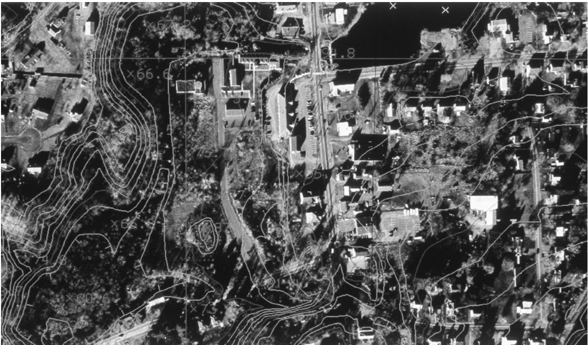
Figure 28.5 Vector data overlaid on a raster image background. (Courtesy Tom Pantages.)
