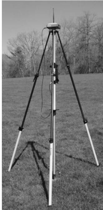
Figure 15.1 A GNSS receiver mounted on a fixed height tripod.
