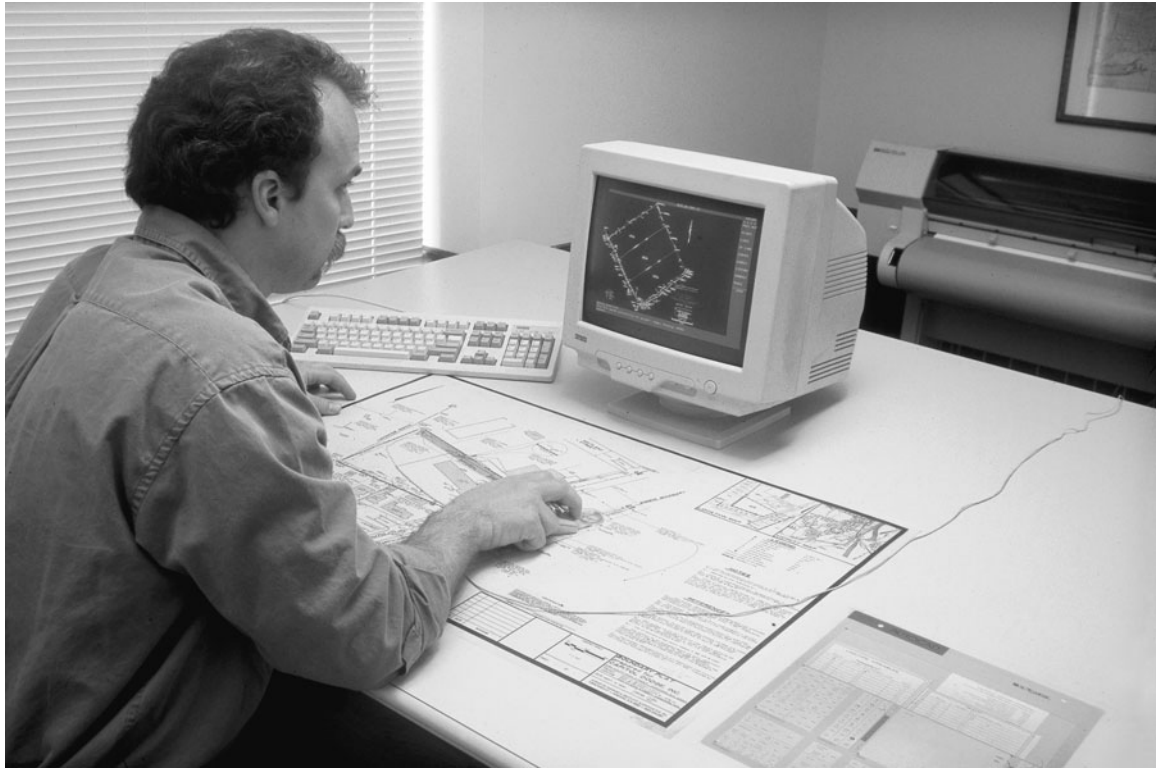
Figure 28.8 Tablet digitizer interfaced with personal computer. (Courtesy Tom Pantages.)
