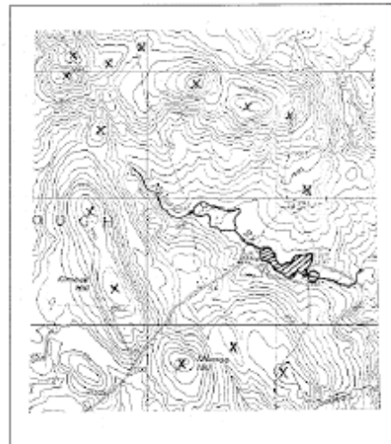
Figure E-4: Delineating a Watershed Boundary - Step 1
