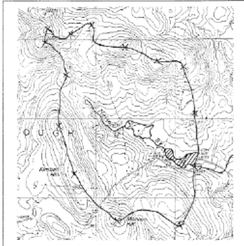
Figure E-5: Delineating a Watershed Boundary - Step 2
