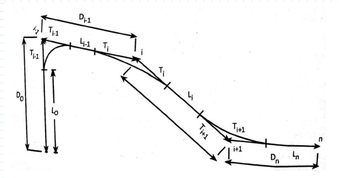
Tangents may be defined as the straight lines obtained by joining two successive points of intersections of the two straight traverse lines along the road route. Net length of tangents in between two curves is obtained by deducing tangents to the curves at adjacent deviation points or intersection points.
