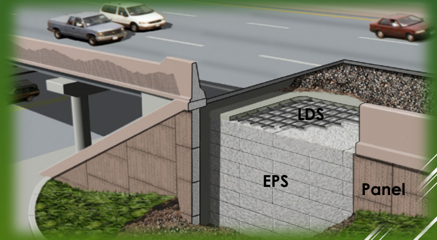
Method 2 – Vertical embankment capped with concrete load distribution slab (LDS) and precast concrete panels
