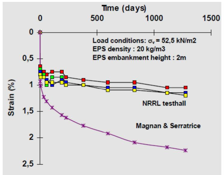
Figure 10. Deformation and creep results from calculated values and full scale laboratory test
