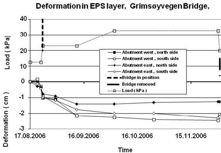
Figure 22. Deformation in EPS embankment at Gimsøyvegen Bridge
