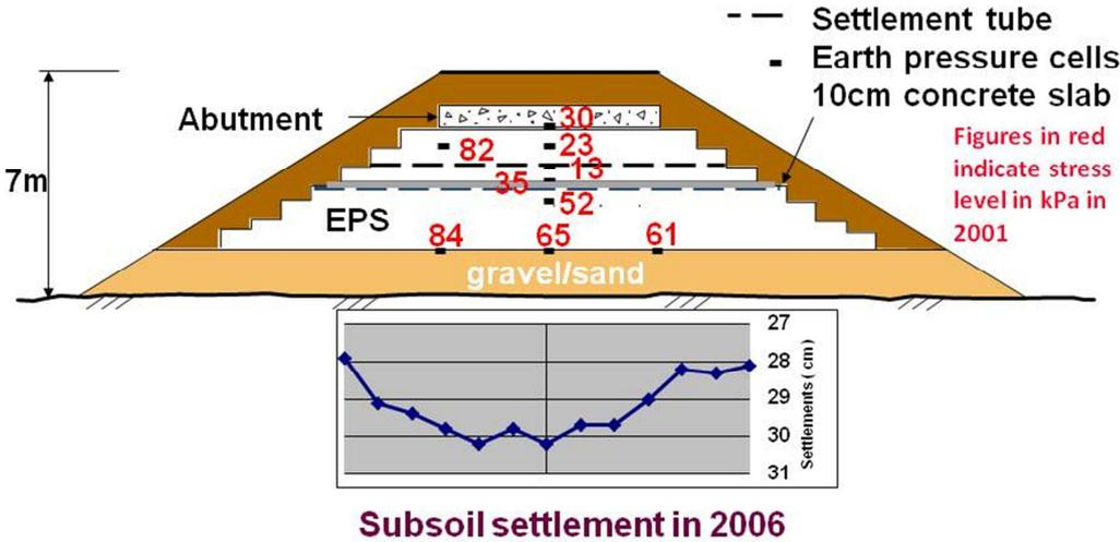
Figure 15. Løkkeberg Bridge. Observed stress distribution and settlements in the cross section.
