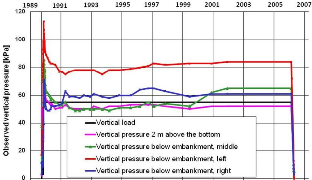
Figure 16. Long term measurements of vertical pressures at Løkkeberg Bridge
