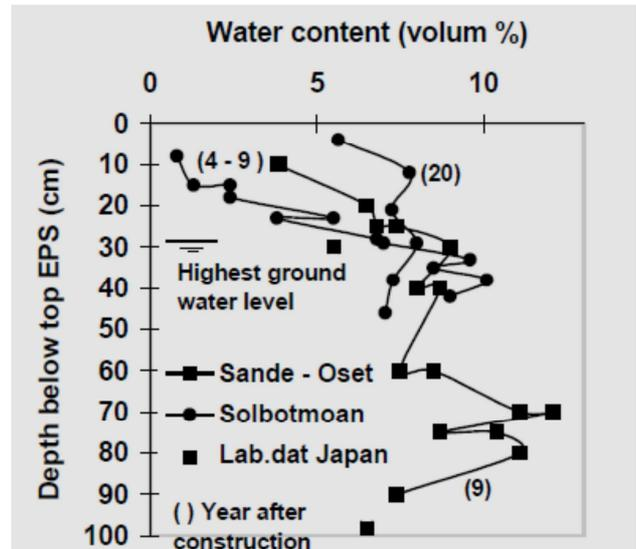
Figure 8. Typical water content in submerged EPS blocks
