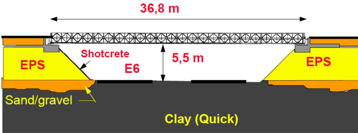
Figure 12. Løkkeberg bridge. Longitudinal profile
