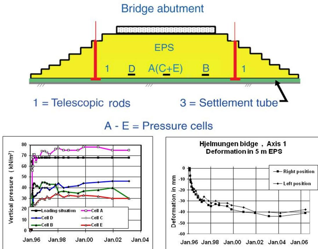
Figure 20. Measured stress and settlements at Hjelmungen
