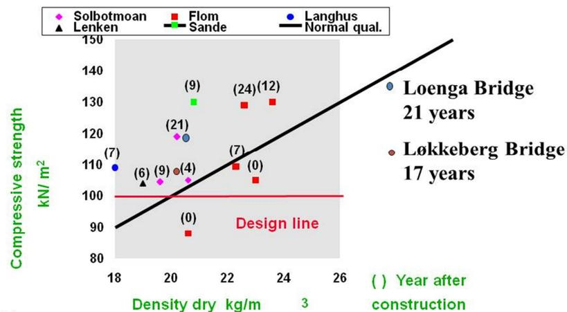
Figure 5. Compressive strength on retrieved samples from EPS embankments
