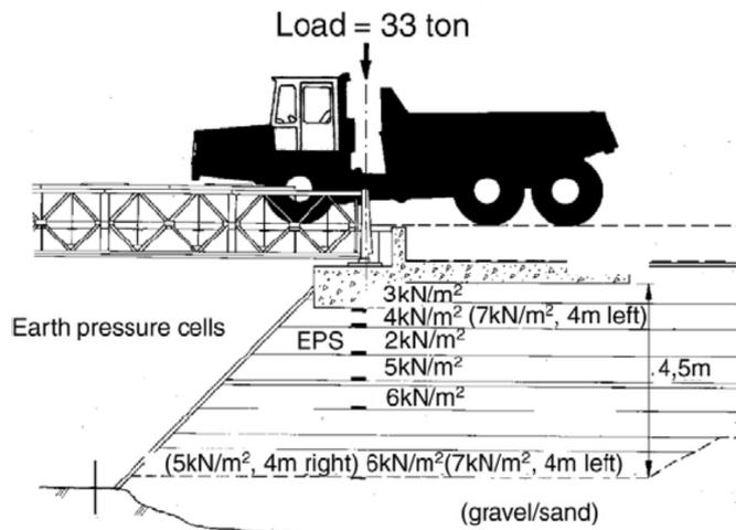
Figure 17. Stress levels in EPS fill at Løkkeberg
