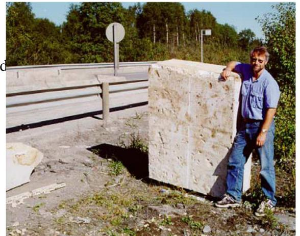
Figure 4. Excavation of a 24 years old EPS block from the first EPS embankment at Flom bridge.
