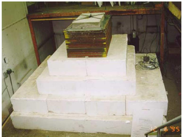
Figure 9. EPS test embankment at the Norwegian Road Research Laboratory.
