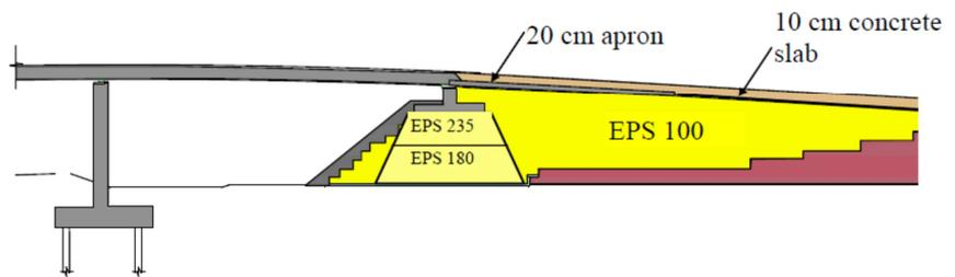
Figure 18. Supporting bridge abutments directly on EPS
