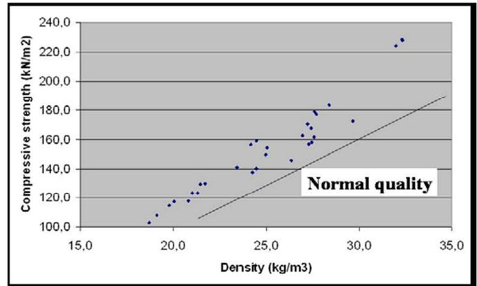
Figure 6 Loenga bridge 1983 Compressive strength after 21 years in the ground
