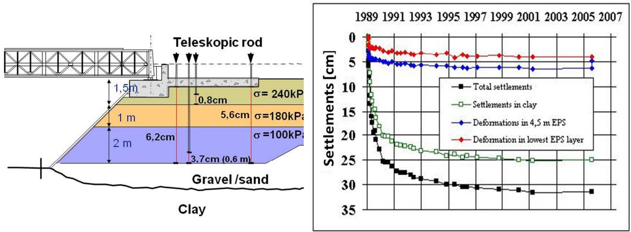
Figure 13. EPS types and deformations in EPS embankment at Løkkeberg.
