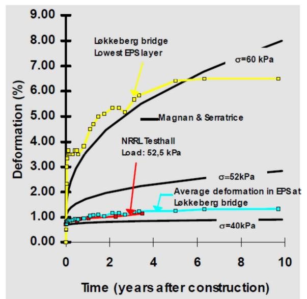
Figure 14. Creep deformations in EPS.
