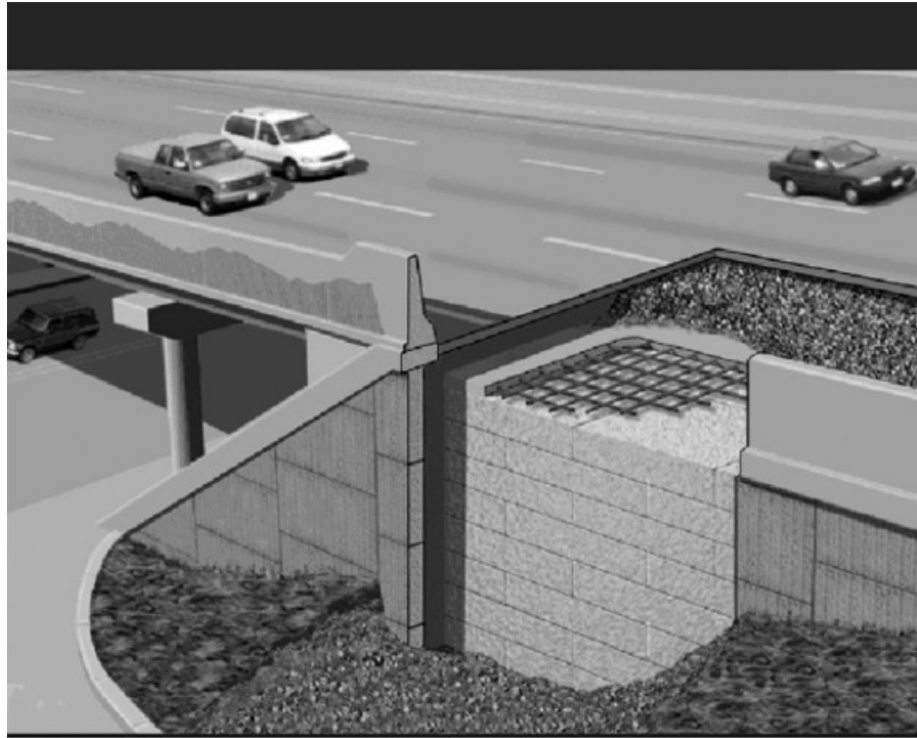
Figure 3: Typical Bridge Abutment with Geofoam Backfill.
