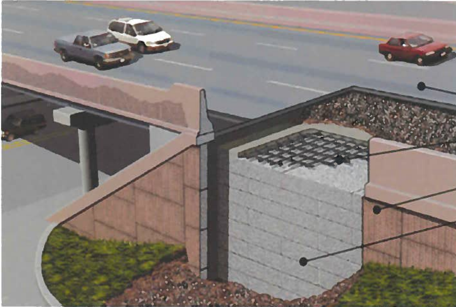
桥梁交叉路口上典型的地基泡沫装置 Typical geofabric installation at a bridge crossing
