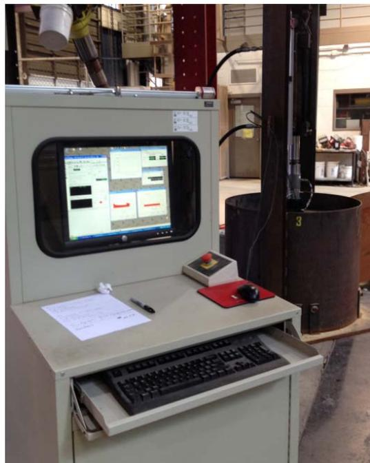
Figure 3.4 Axial Displacement and Force Measurement System
