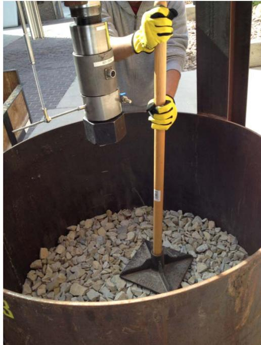
Figure 3.1 Compaction of Specimen
