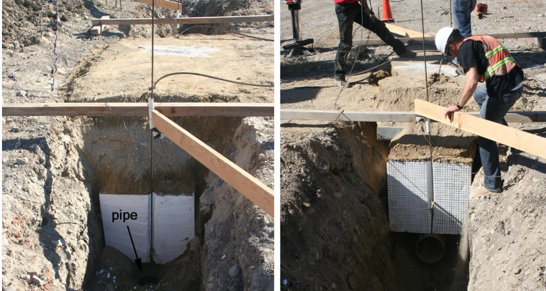
Fig. 3. Pre-test (left) and post-test (right) of pipe uplift test of EPS cover system.
