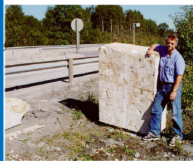
Figure 4. Excavation of a 24 years old EPS block from the first EPS embankment at Flom bridge.
