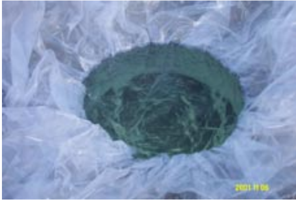
Figure 10: Water used to measure excavated volume.
