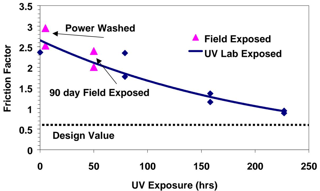
**Figure 8. Interface Coefficients for Geofoam – Cast in Place Concrete with UV Exposure Duration.**
