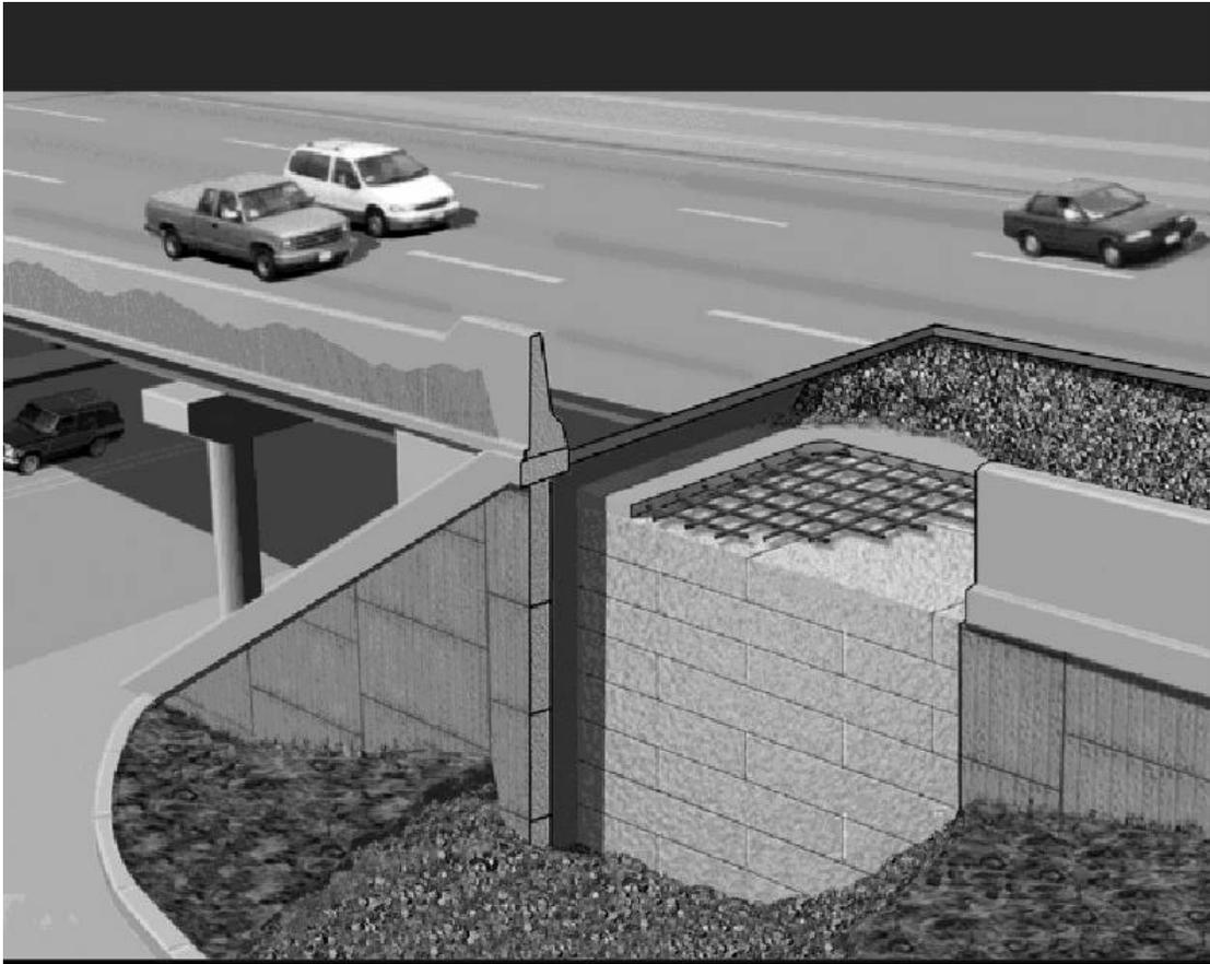
**Figure 3. Typical Bridge Abutment with Geofoam Backfill.**
