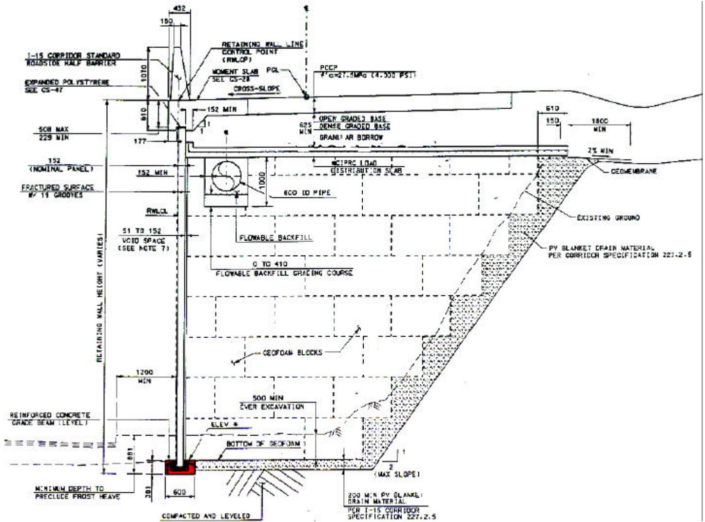
Figure 4. Details of a Typical I-15 Project Geofill.
