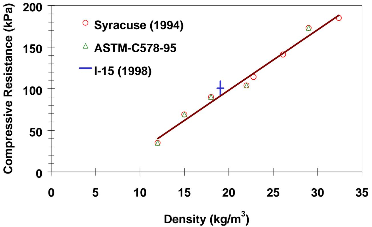
Figure 6. Compressive Resistance versus Geof foam Density.
