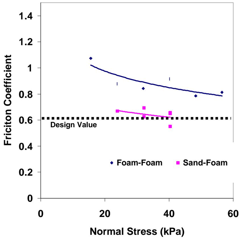
Figure 7. Interface Coefficients for Type VIII Geofoam.
