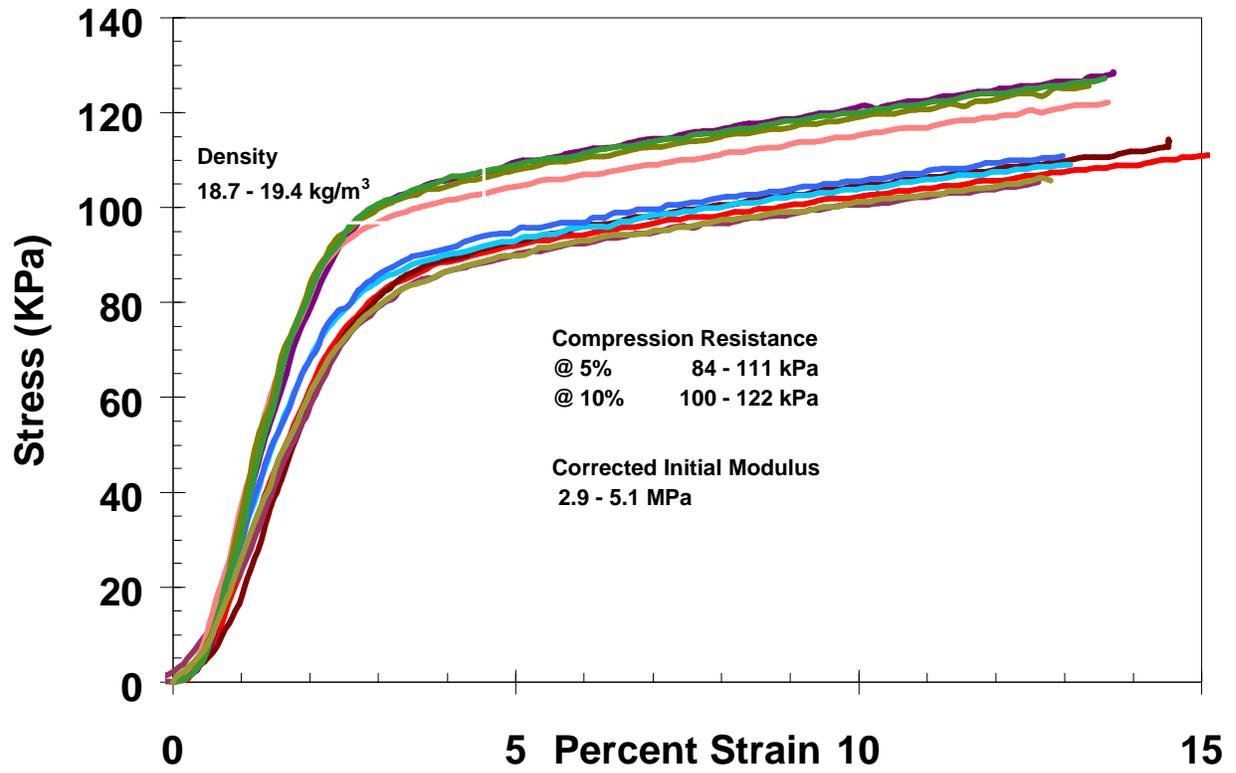
**Figure 5. Stress-Strain Curves for Type VIII Geofoam, 50-mm Samples at 10% Strain Rate.**
