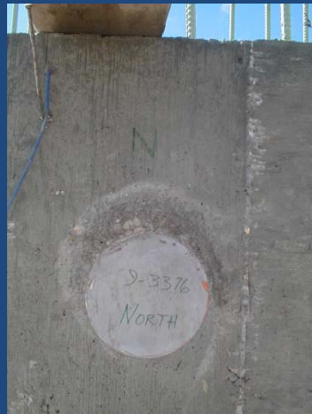
Pressure Cell Cast in Bridge Abutment
