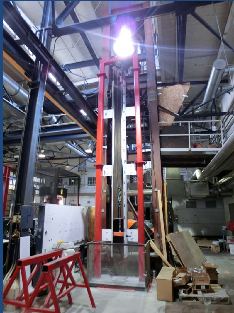
Impact Hammer and Test Frame
