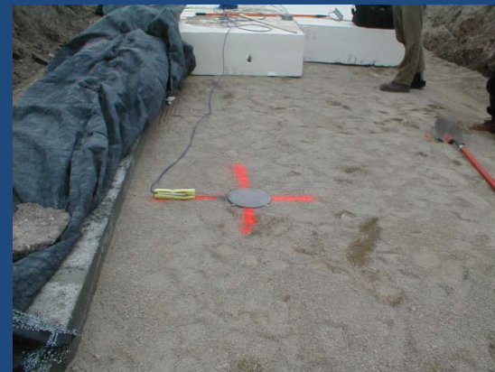
Pressure Cell in Base Sand
