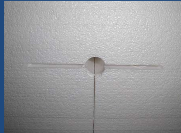
Hotwire Cut Slot for Pressure Cell
