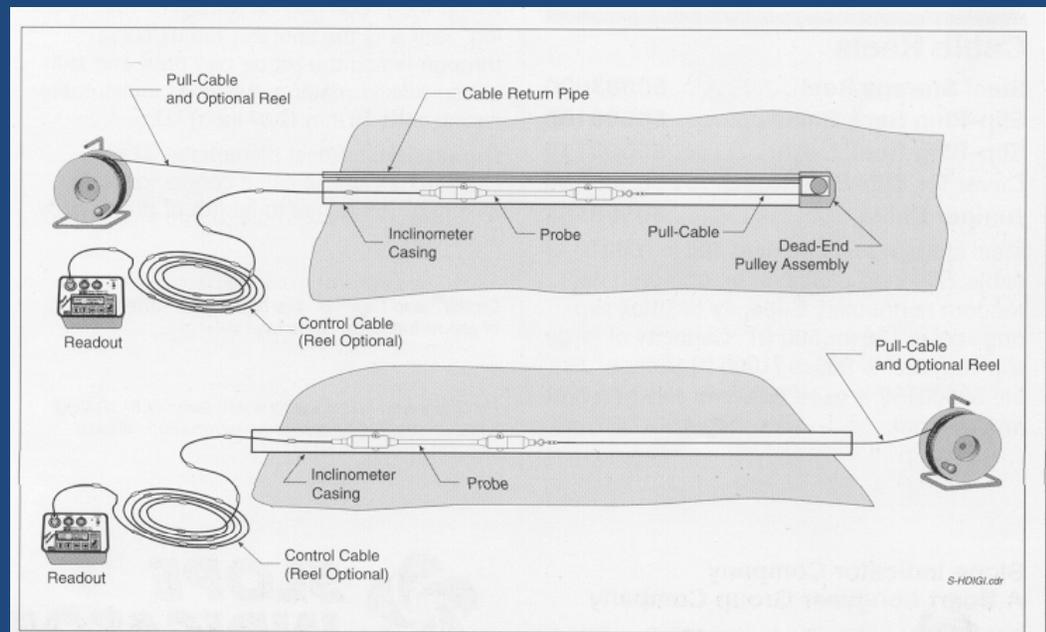
Horizontal Inclinometer Systems, with and without dead-end pulley assembly
