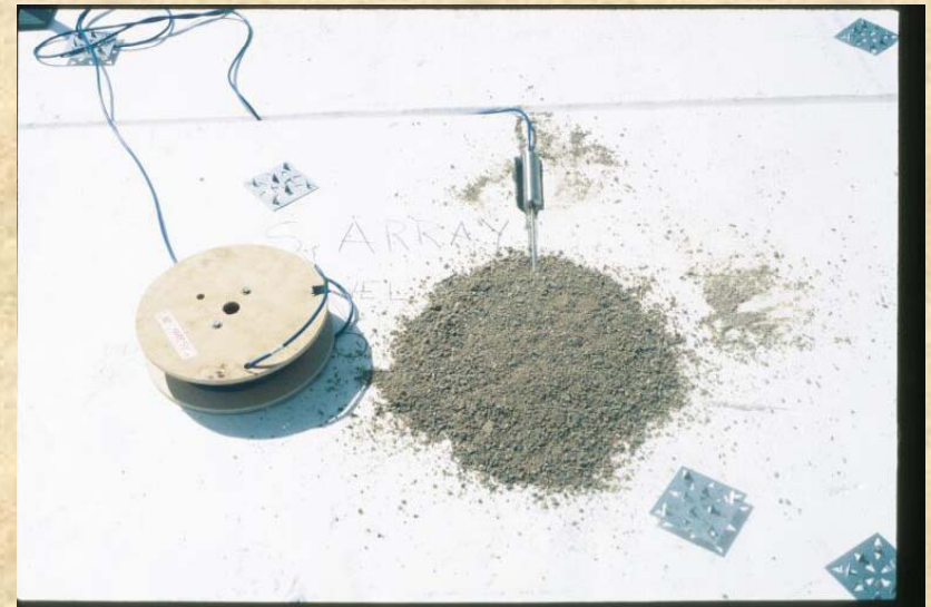
First Method of Placing Pressure Cell
