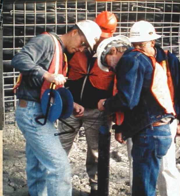
Reading of Sondex Extensometer
