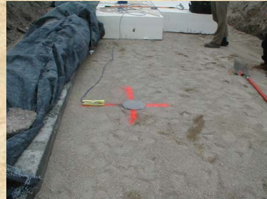
Pressure Cell in Base Sand
