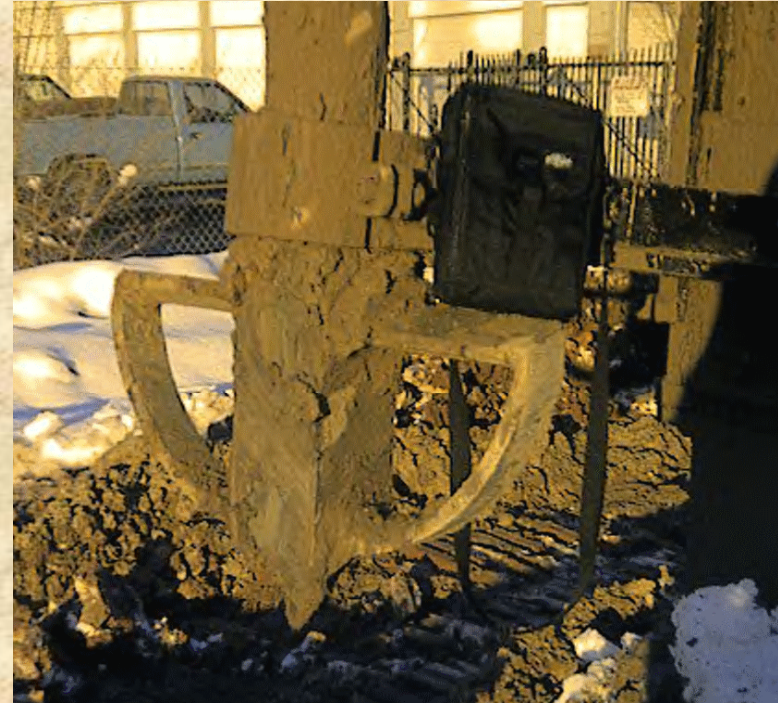
Auger / Mixer for Lime and Cement
