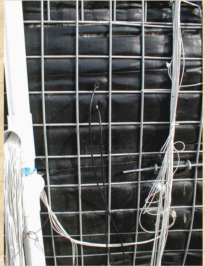
Strain gage wiring at face of MSE wall
