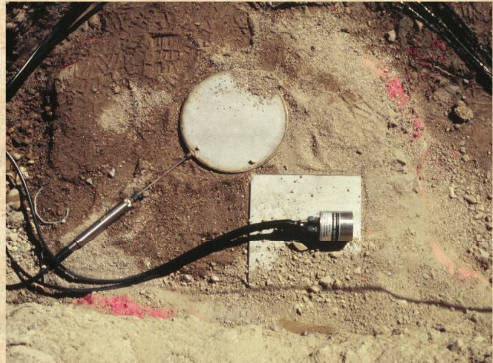
Pressure and Settlement Cells Atop Column
