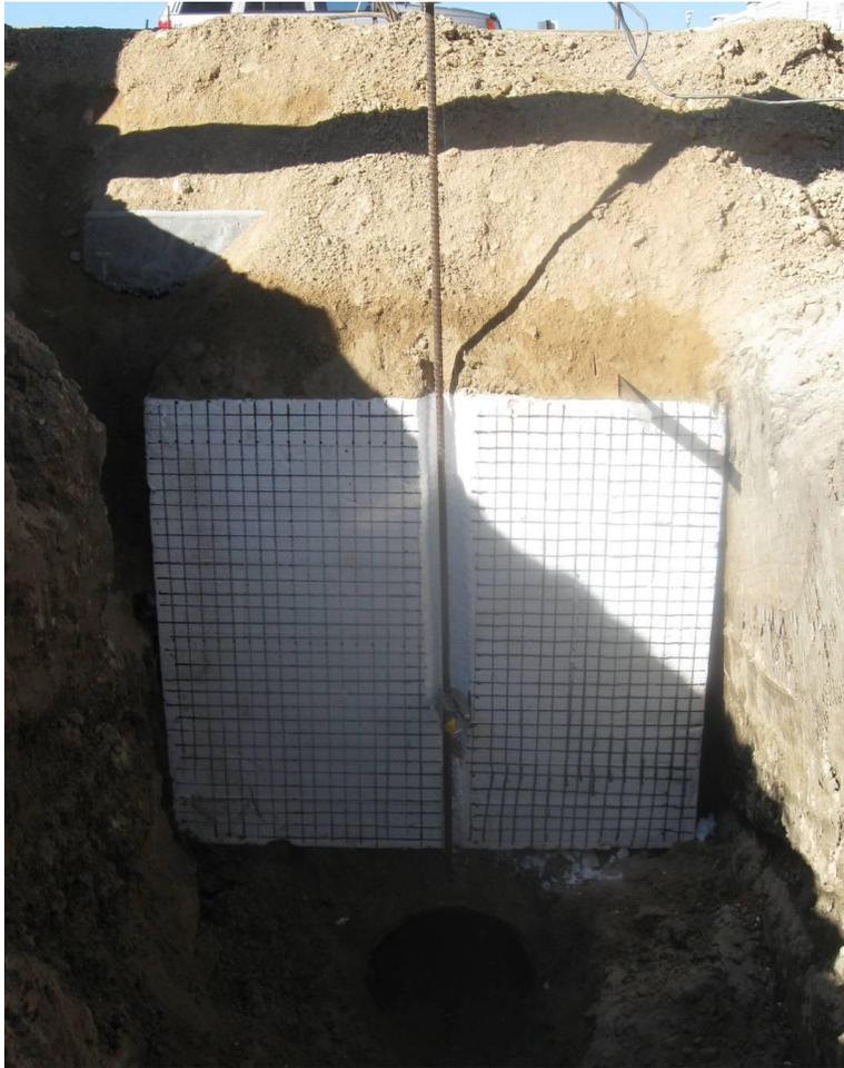
**Figure 13. Photograph of the end of trench, pipe, EPS block prior to uplift test.**
