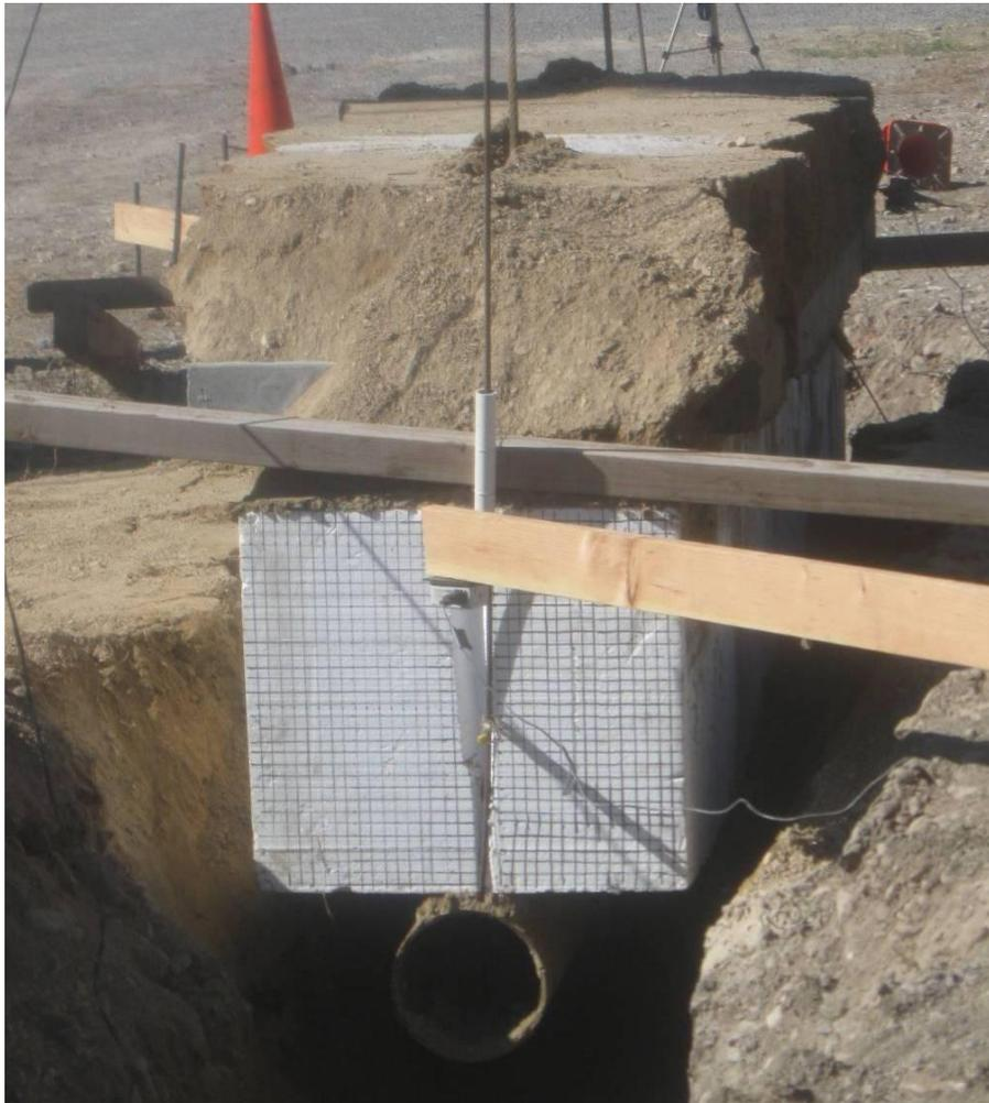
**Figure 14. Photograph of the end of the trench, pipe, EPS block after uplift test.**
