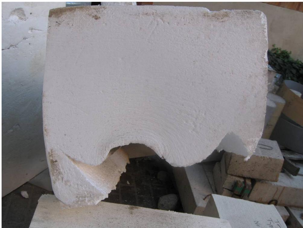
Figure 52. Localized deformation of an EPS block loaded by pipe in the trench box
