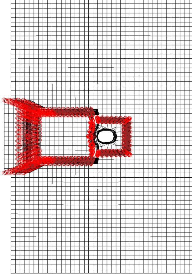
Figure 116. Interface contact at end of uplift for EPS Geofoam model with interfaces
