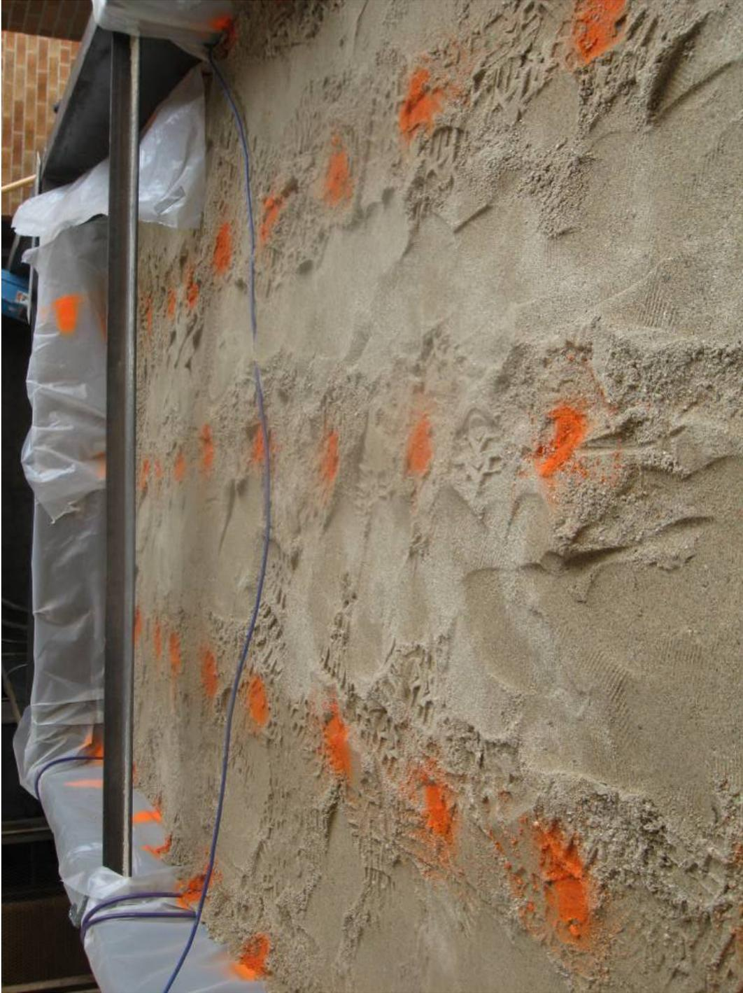
Figure 42. Completely filled trench box with survey grid ready for testing
