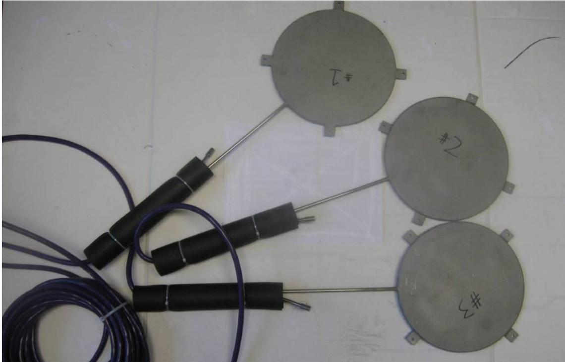
Figure 192. Geokon total earth pressure cells
