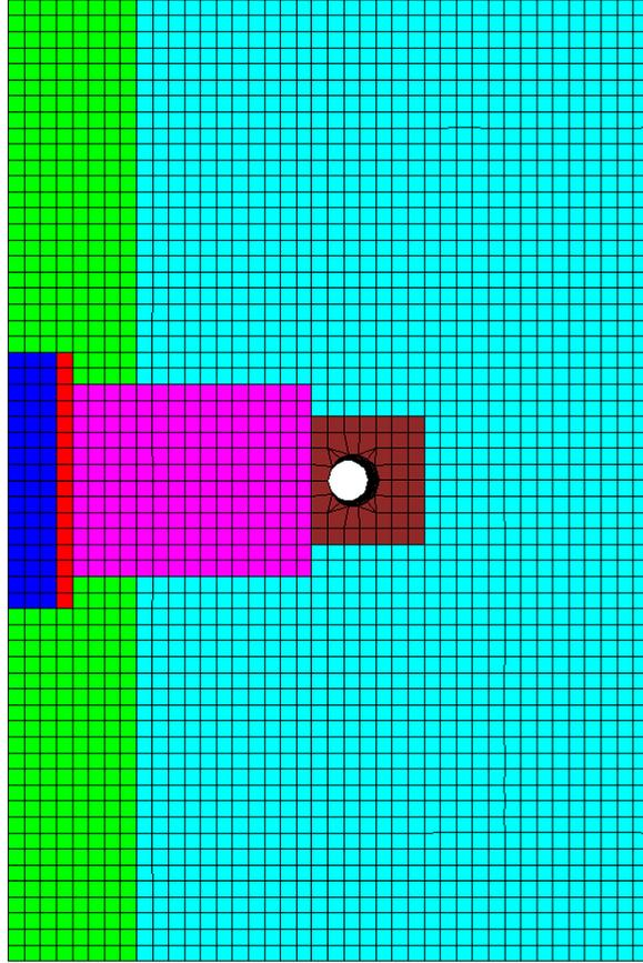
Figure 113. FLAC3D Geofoam model geometry with interfaces
