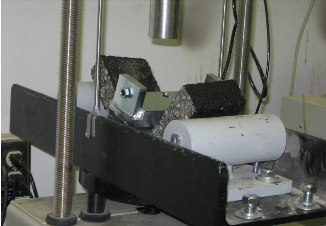
Figure 126. Cracked asphalt beam after 3-Point beam test
