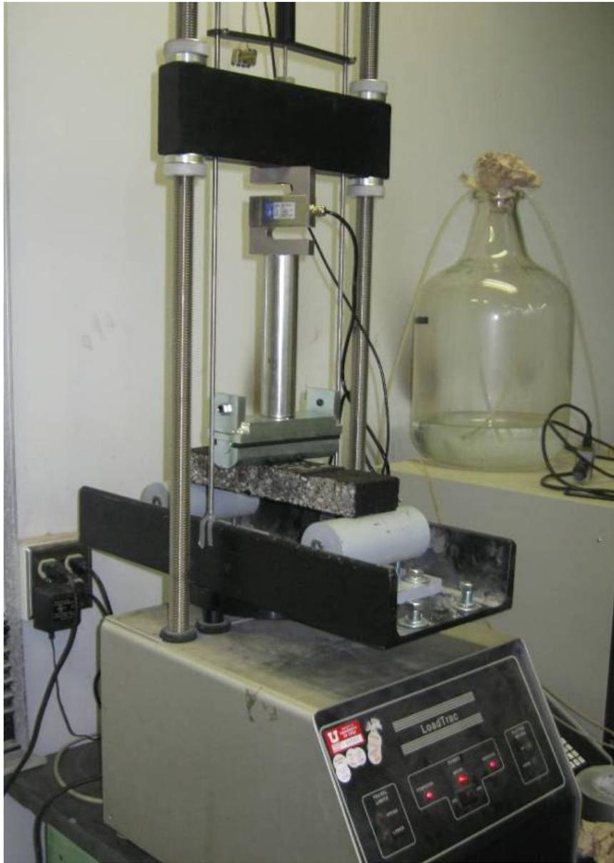
Figure 125. LOADTRACK and asphalt beam
