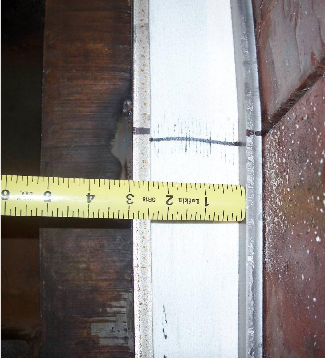
Figure 18. EPS block height at end of compression in the large load frame
