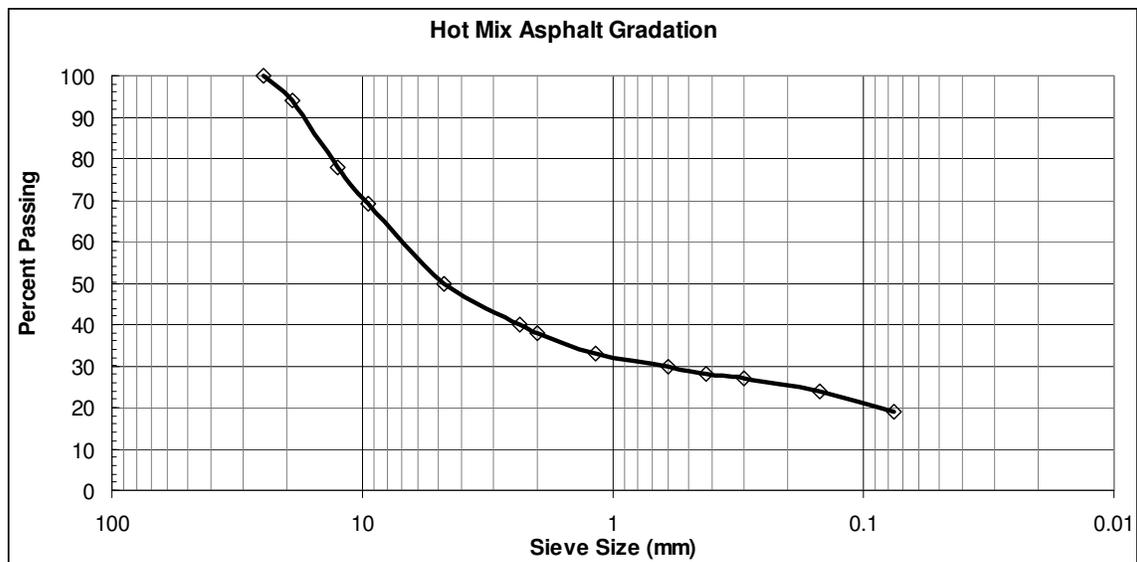
Figure 123. Gradation of HMA used in beam tests
