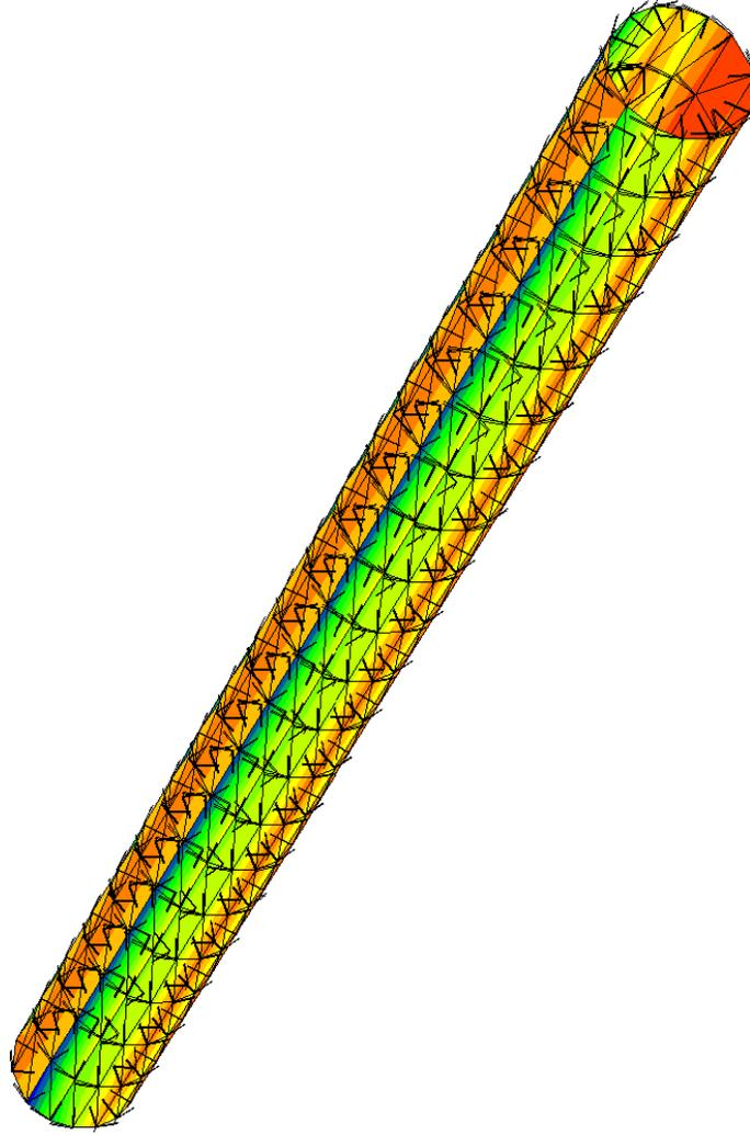
Figure 119. Vertical stress on pipe at end of uplift for Geofoam model with interfaces
