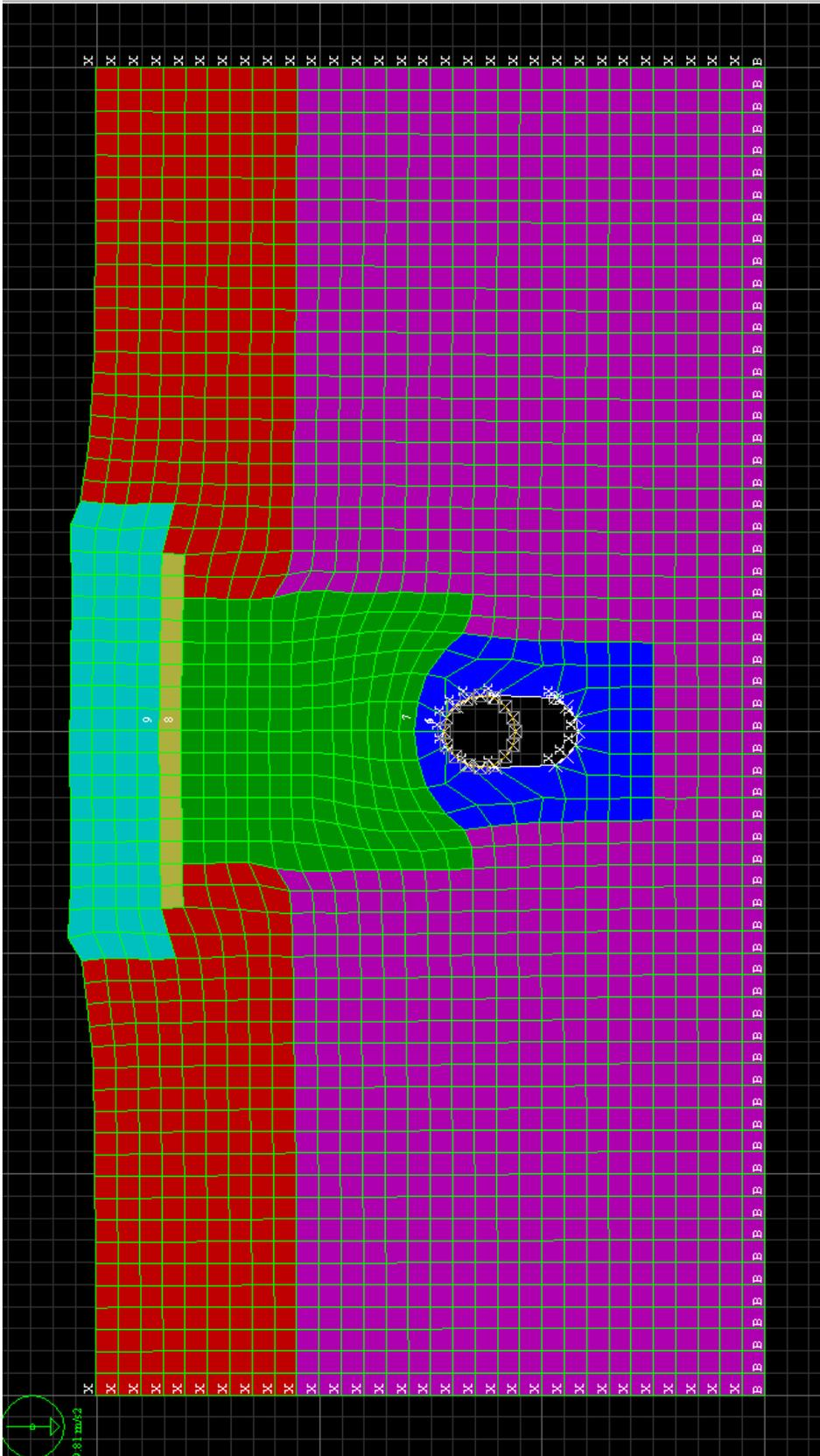
Figure 92. EPS section deformed mesh, no interfaces
