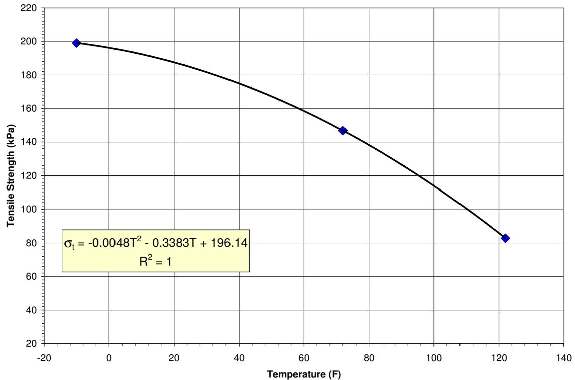
Figure 127. Relationship of tensile strength and temperature
