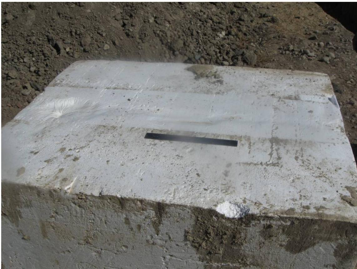
Figure 71. Deformations along bottom of Geofoam block
