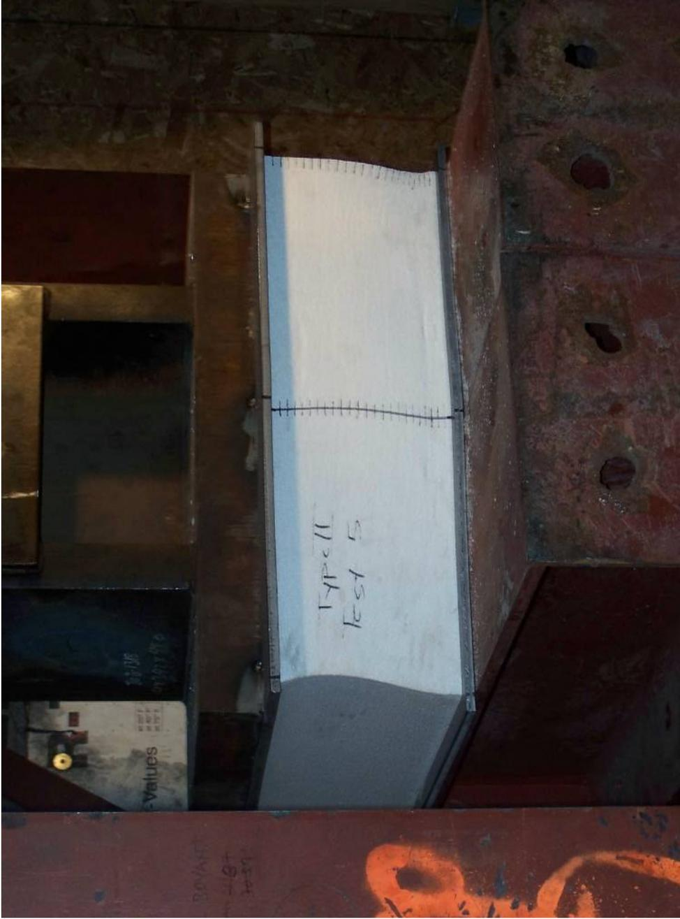
Figure 14. EPS block during compression in the large load frame
