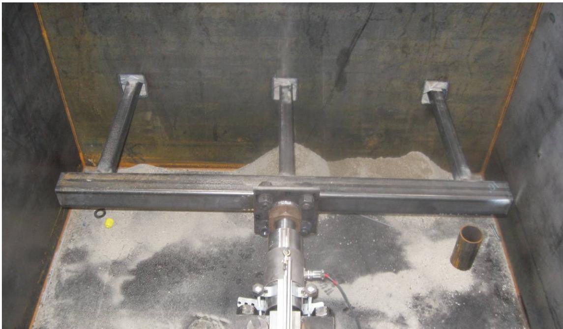
Figure 190. Load cell connecting to push rods
