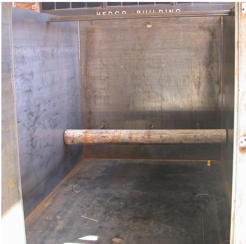
Figure 41. Initial position of pipe in trench box before sand placement
