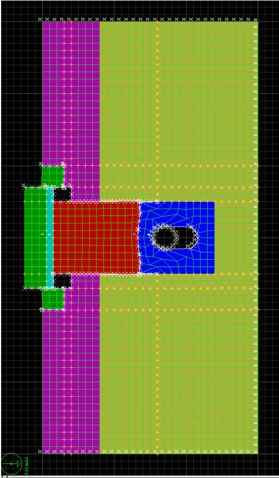
Figure 96. EPS Geofam model with interfaces deformed mesh
