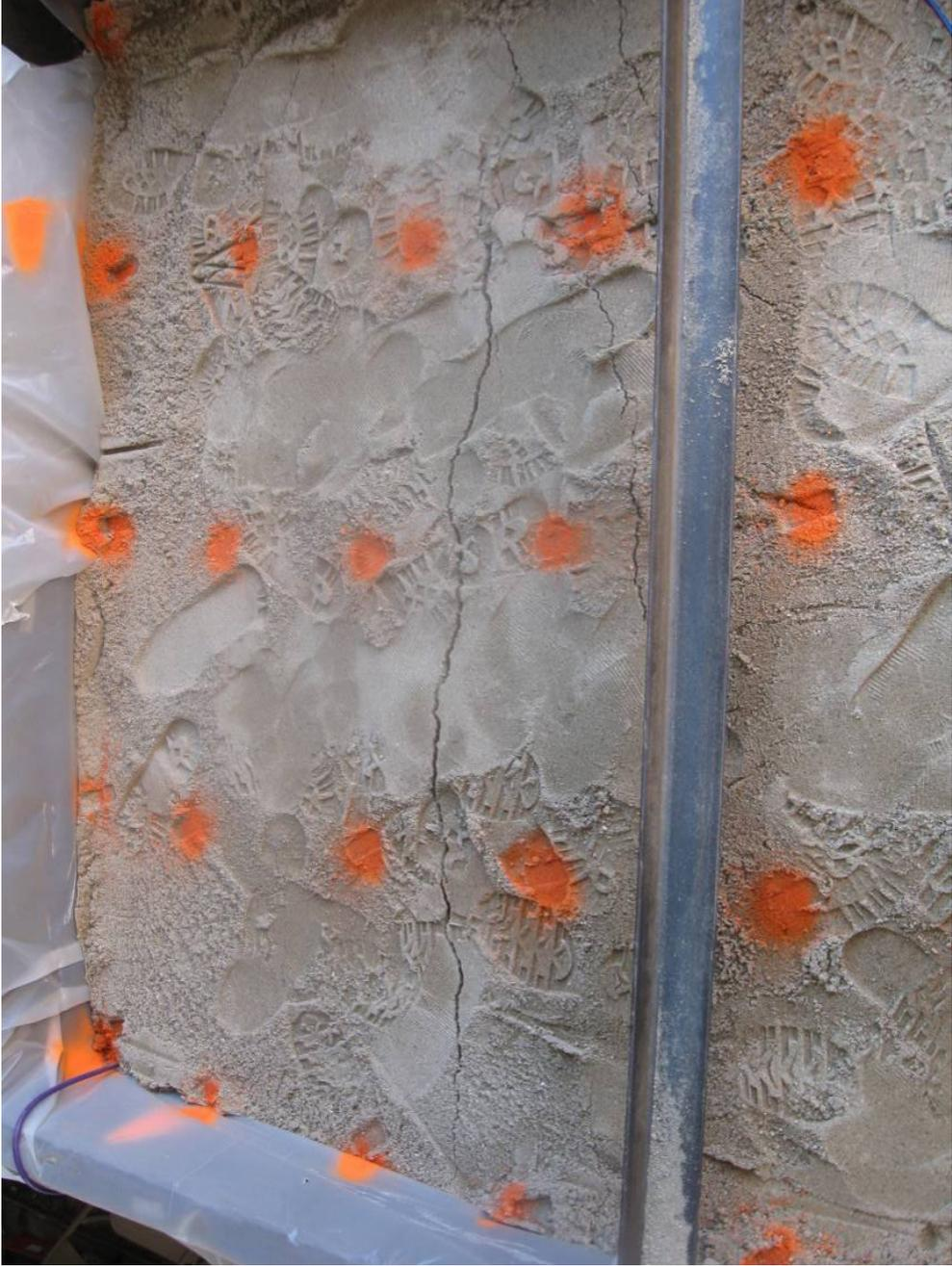
Figure 43. Posttest photograph of top of box and developed cracking pattern fissured sand after testing
