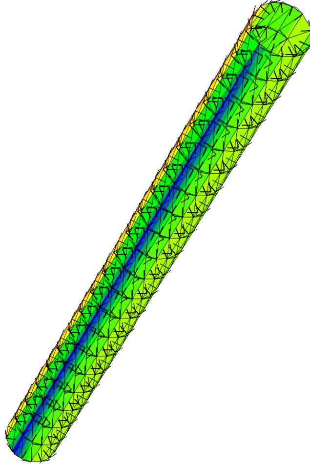
Figure 120. Shear stress on pipe in Geofomo model with interfaces
