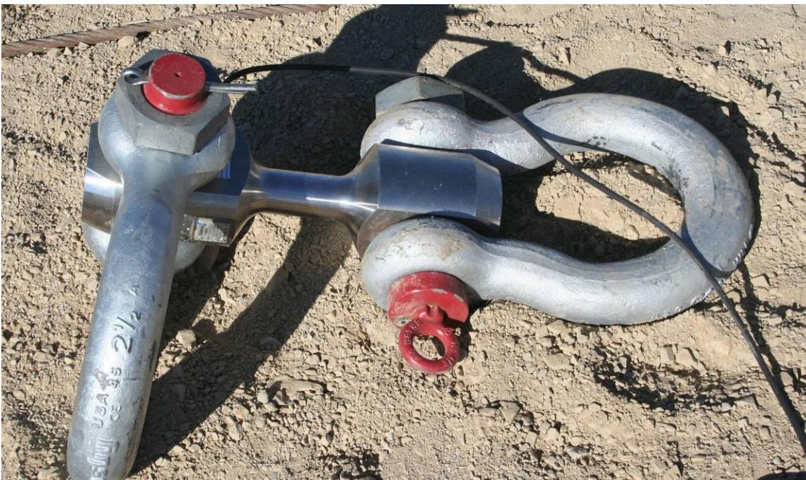
Figure 195. Strainertension load cell and shackles
