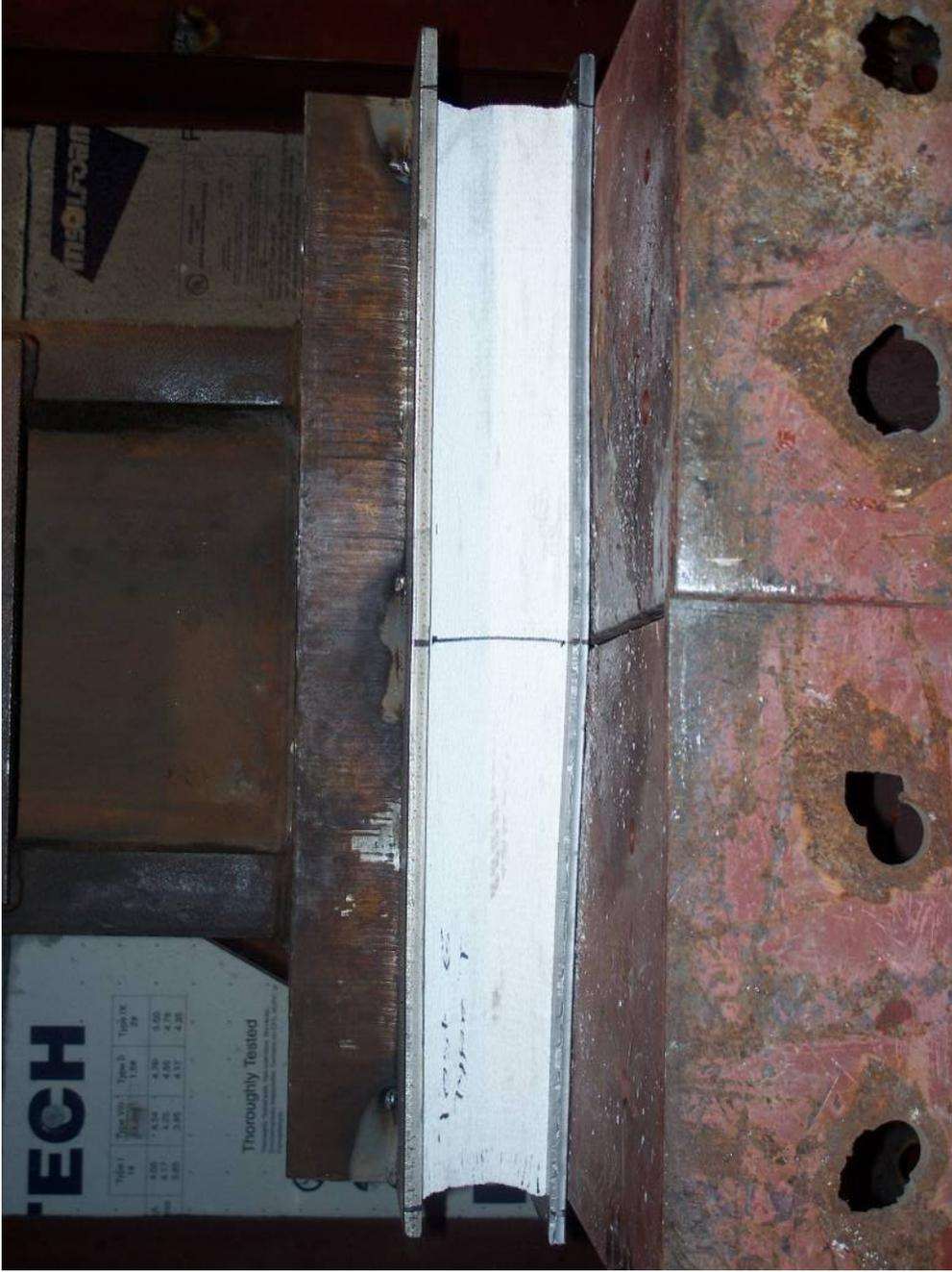
Figure 15. EPS block at end of compression in the large load frame
