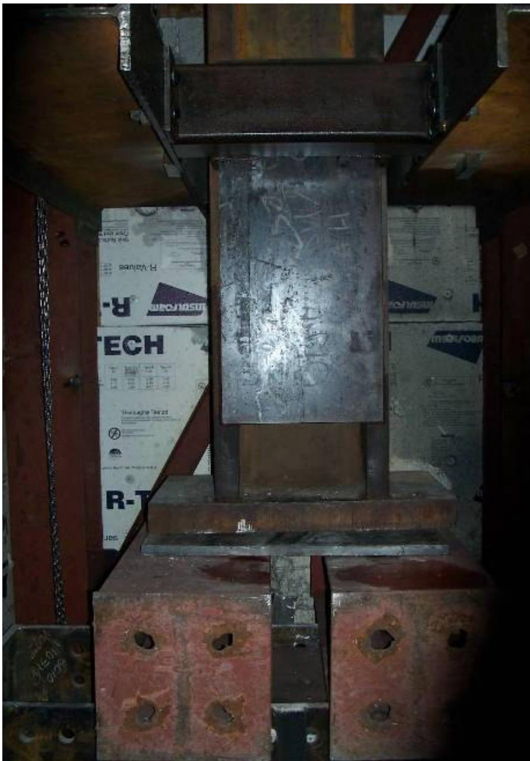
Figure 12. Large load frame for EPS block tests at full stroke
