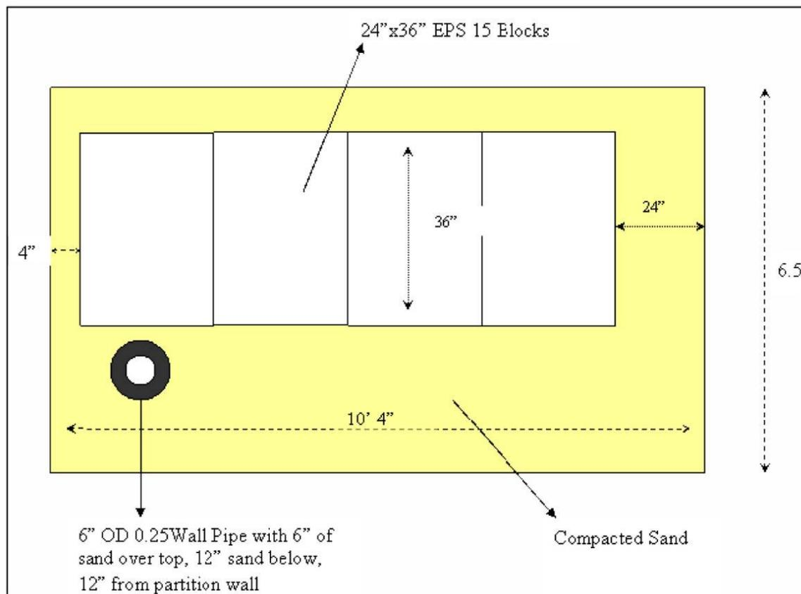
Figure 44. EPS block layout for test 4
