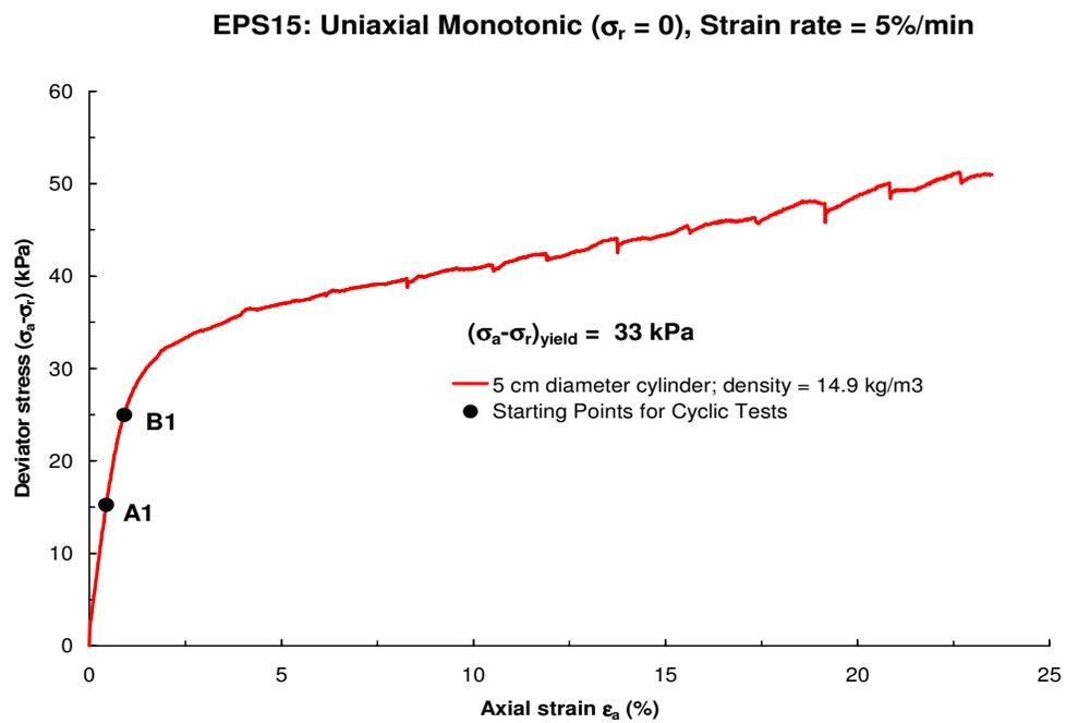
Figure 168. Uniaxial monotonic test result on EPS15
