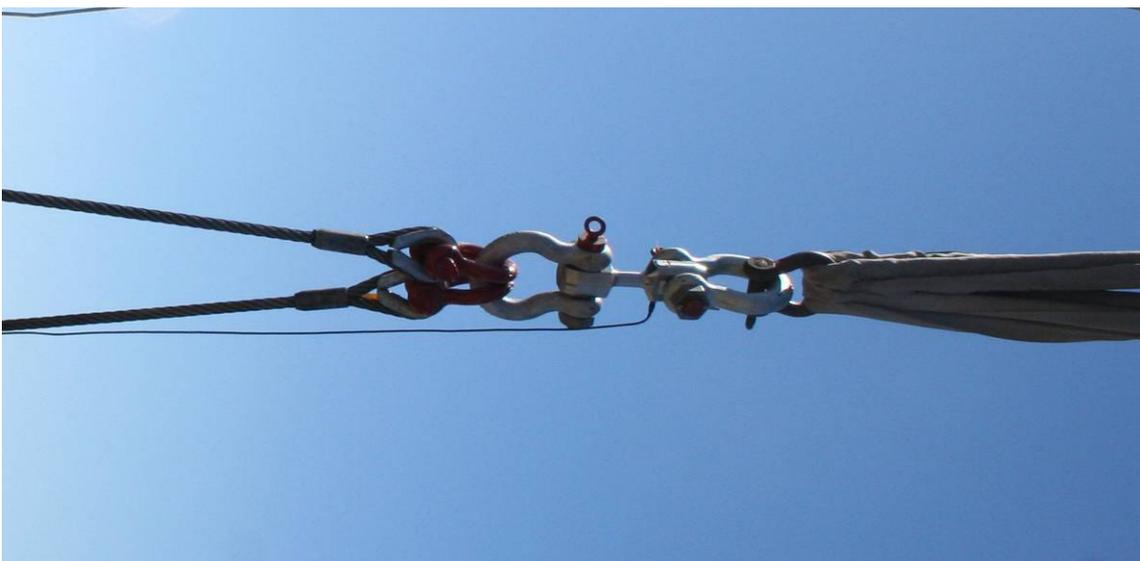
Figure 196. Strainertension load cell and crane cables
