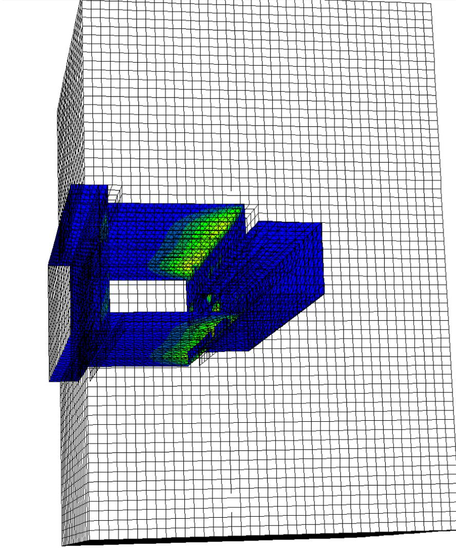
Figure 115. FLAC3D Geofem model with interfaces, interface normal stress
