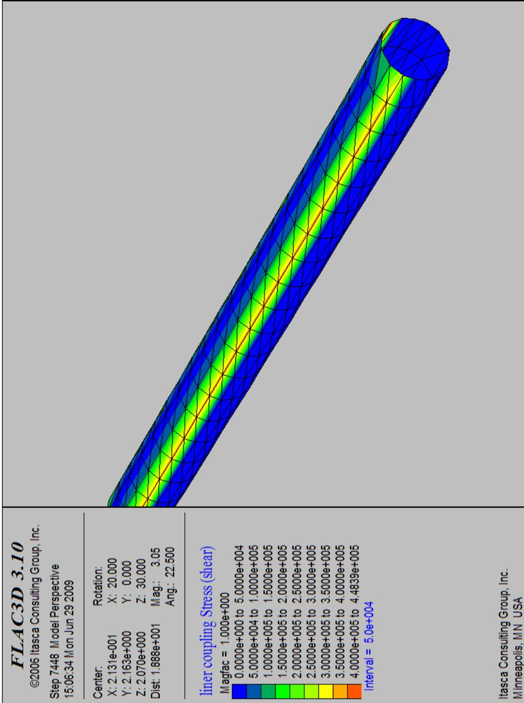
Figure 111. Pipe shear coupling stresses from soil backfill model
