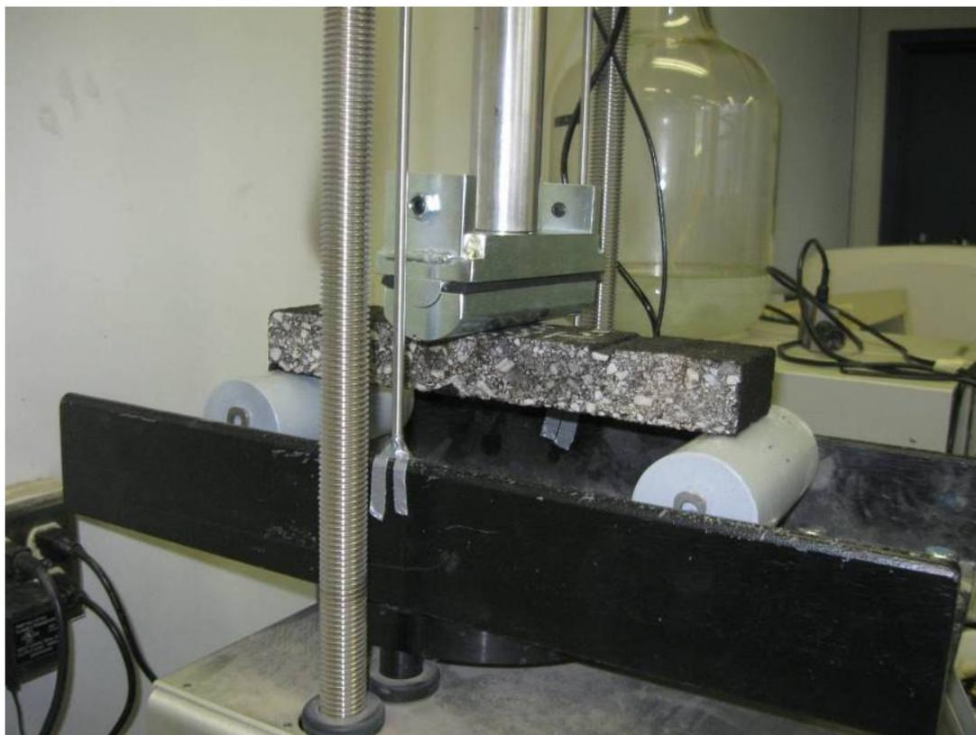
Figure 124. Asphalt beam on rollers
