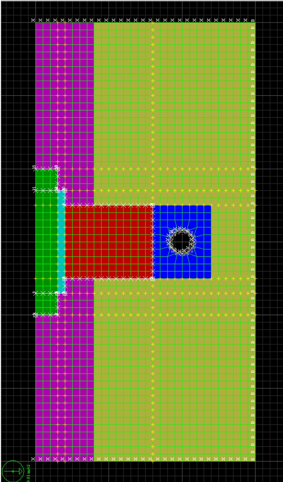
Figure 86. Geofram section model with interfaces
