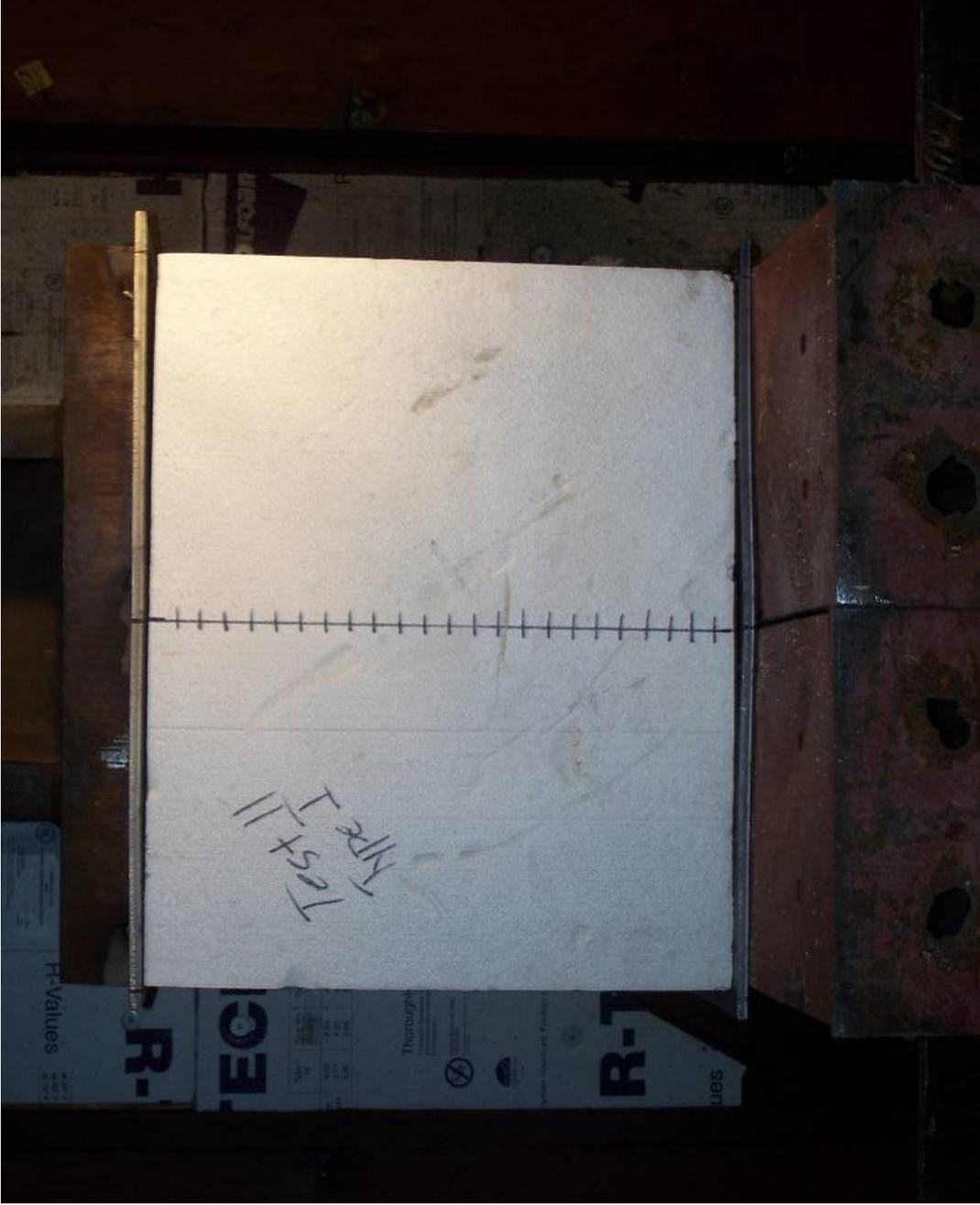
Figure 13. EPS block positioned in large load frame prior to testing
