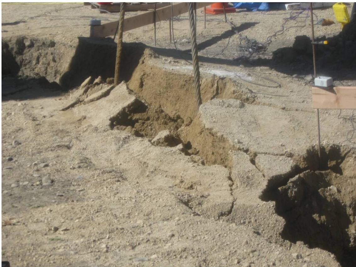
Figure 69. Uplifted soil backfill system
