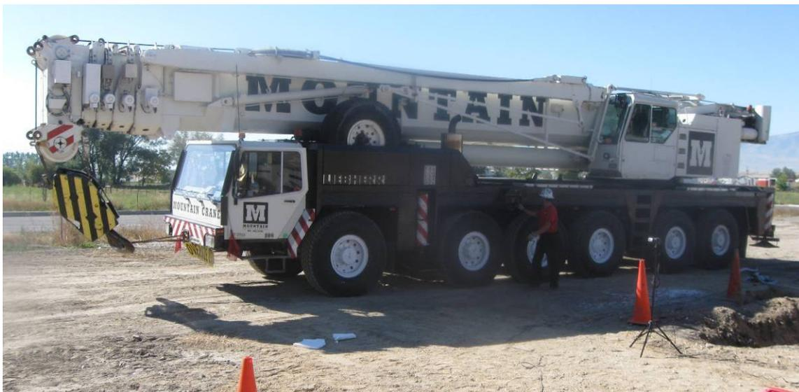
Figure 68. Tire mounted crane used for uplift tests
