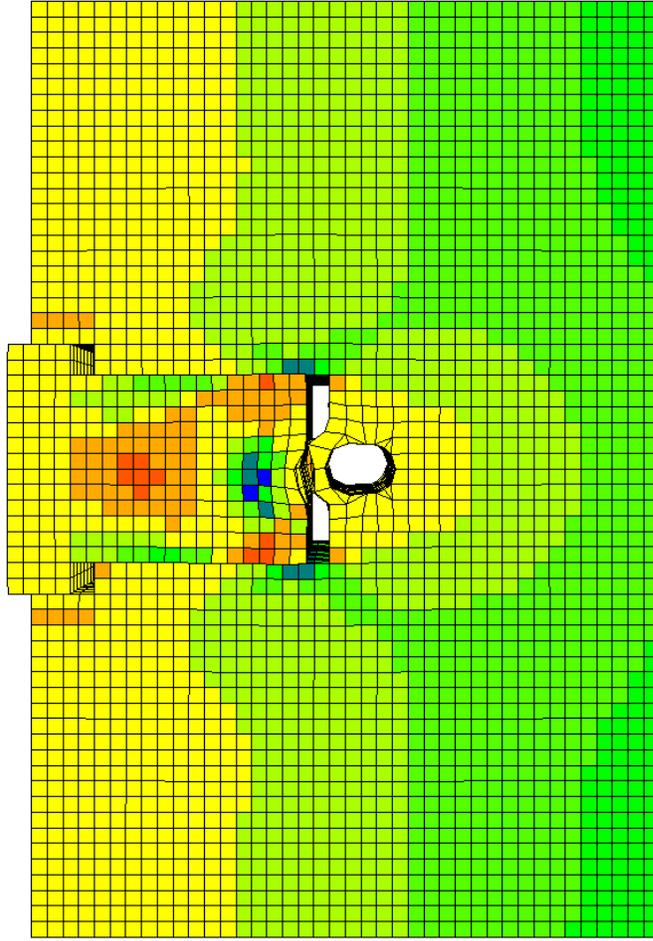
Figure 118. Vertical stress contours for Geofoam model with interfaces
