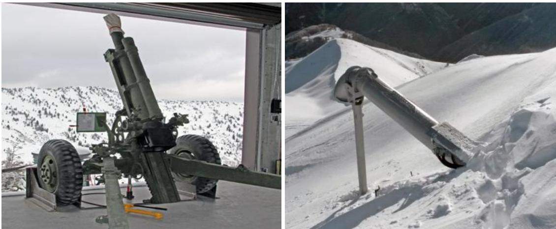
Figure 3 – Alta's Howitzer (left) and Gazex® Device (right)
