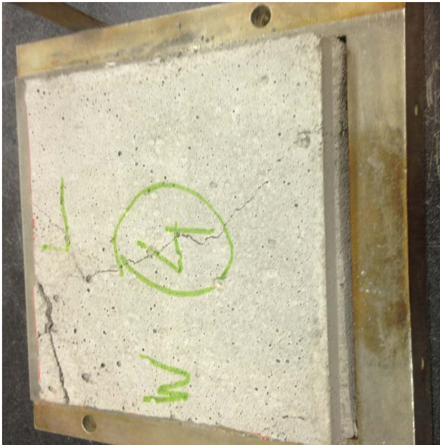
Figure 4: Close view of the sample after completion of direct shear test
