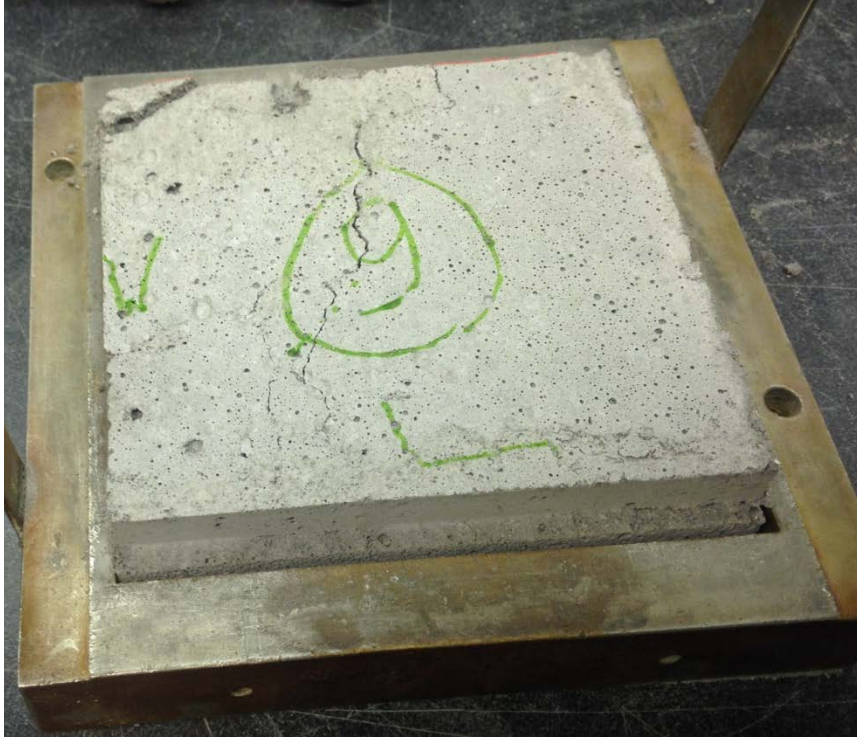
Figure 3: Sample after completion of direct shear test
