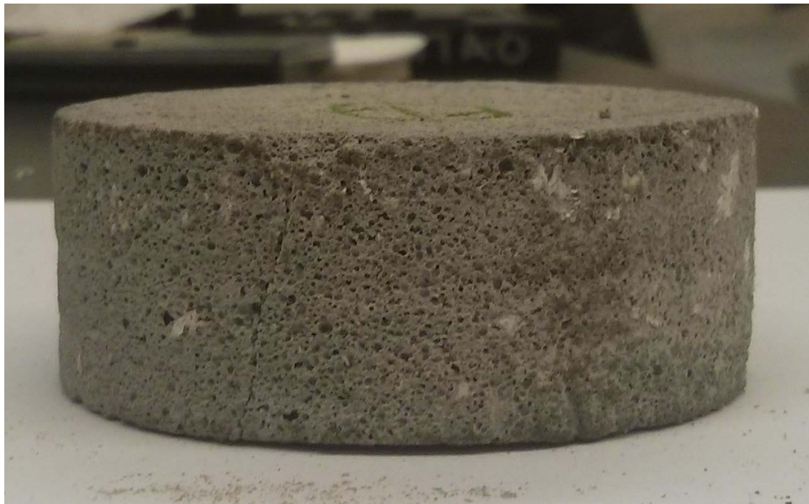
Figure 16: Photograph of a sample after cyclic simple shear test.
