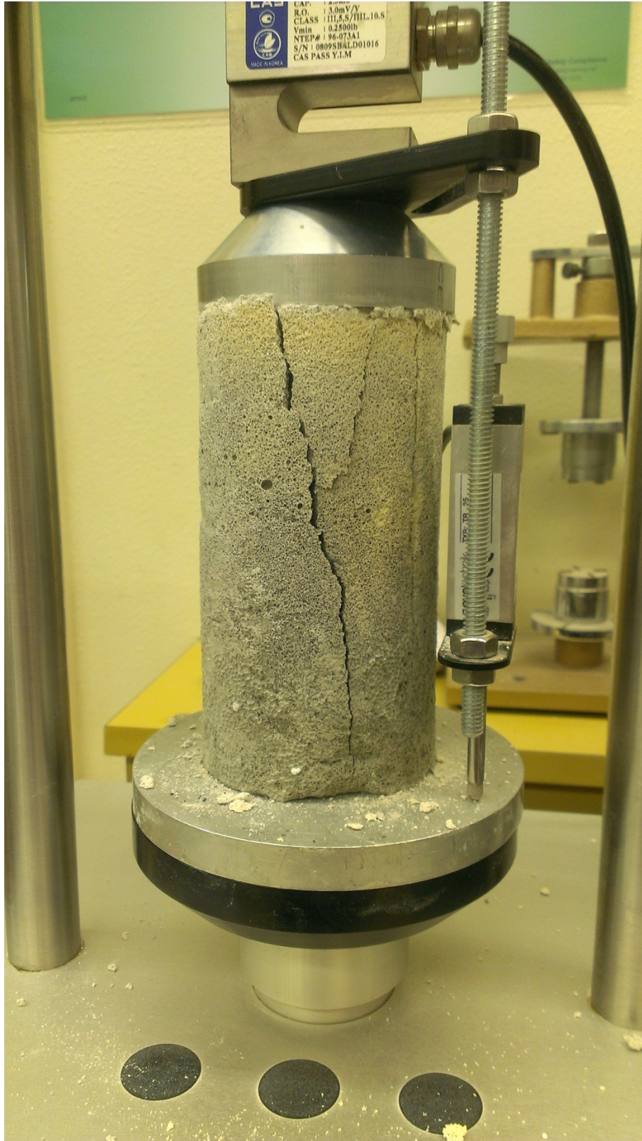
Figure 6: Cracking pattern observed during unconfined compression test
