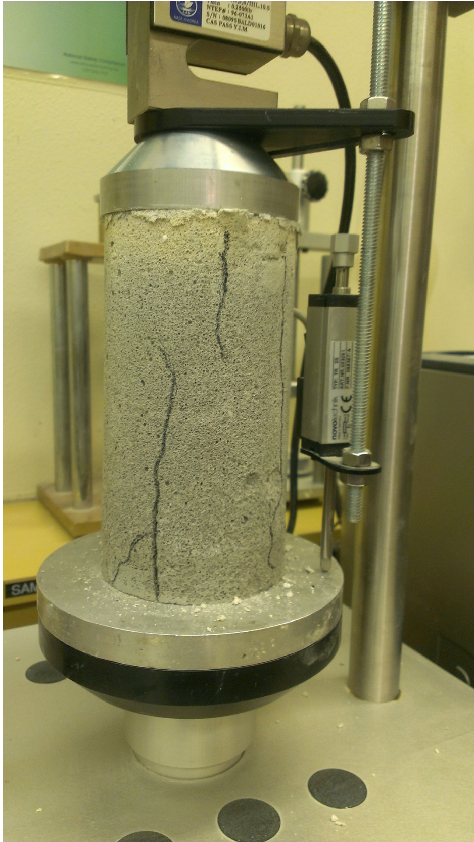
Figure 7: Cracking pattern observed during unconfined compression test
