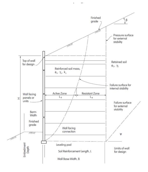
Figure 5.9.1-1 MSE Wall Element Dimensions Needed for Design.
