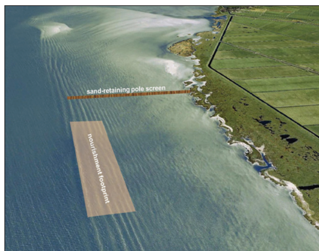
Figure 5. Workumerwaard shore nourishment design – 31 500 m 3 of dredged sediment was placed in a 600 m long, 100 m ridge around 600 m from the shore
