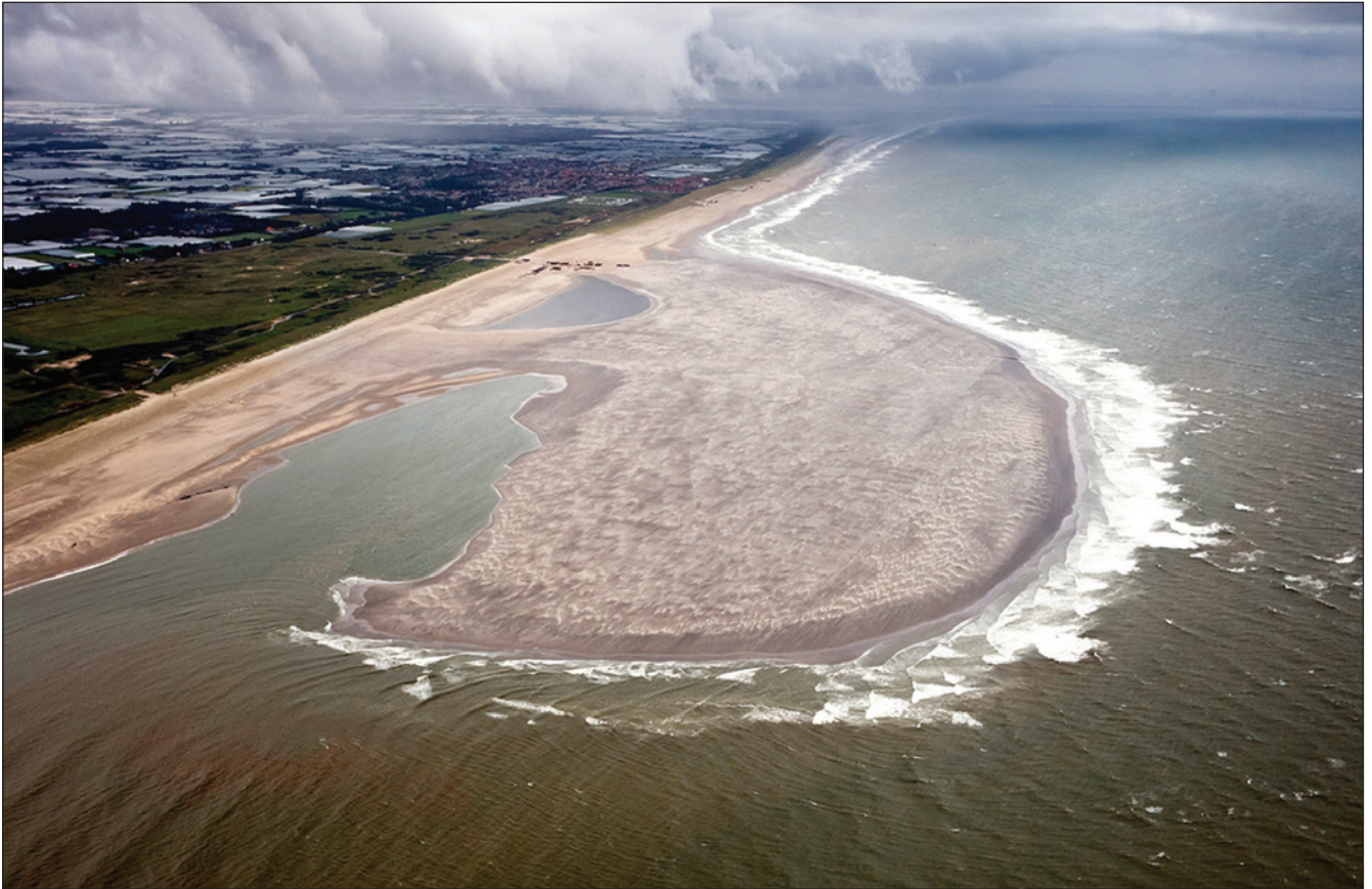
Figure 1. Delfland sand engine in July 2011, just after completion – a total of 20 million m 3 of sand was placed in front of the existing shore (https://beeldbank.rws.nl, Rijkswaterstaat / Joop van Houdt)
