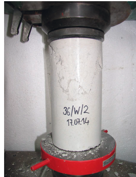
FIGURE 4: Typical failure pattern observed during compression tests with cylindrical specimens.
