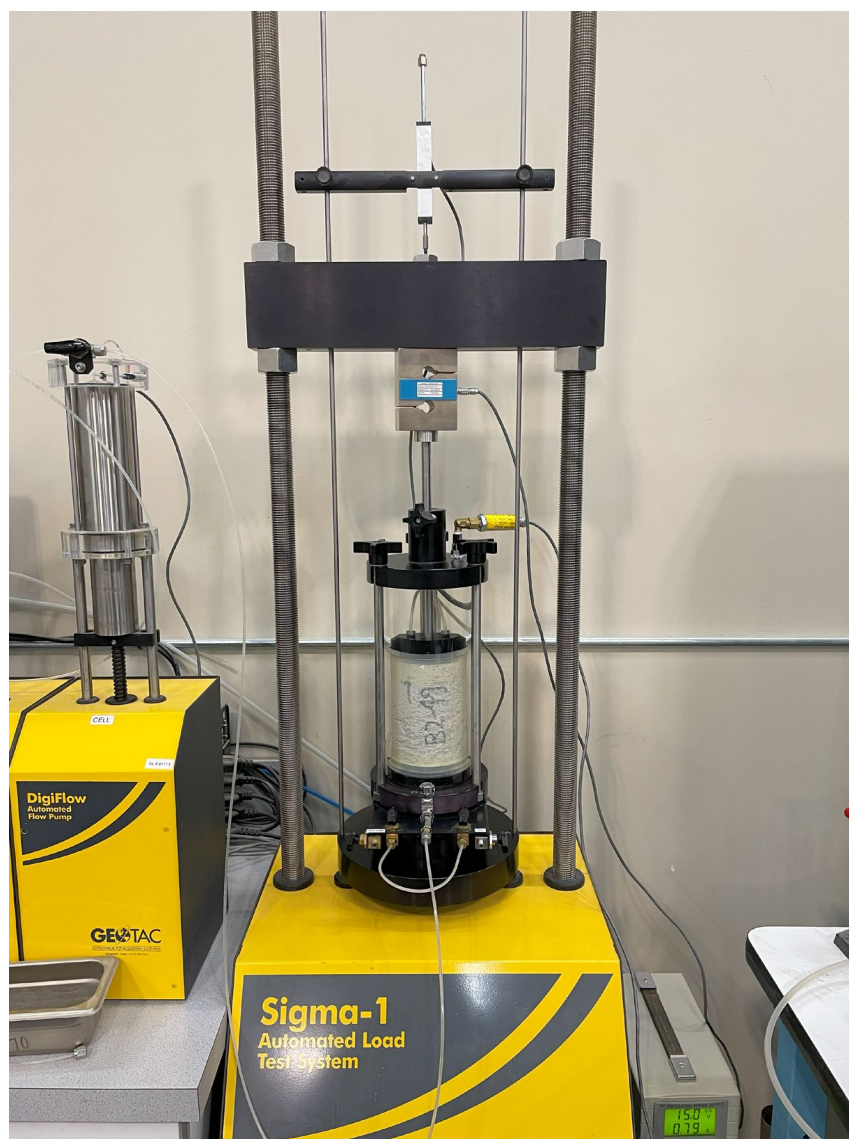
Figure 50. Photo of the triaxial testing apparatus with a test specimen in the triaxial cell.
