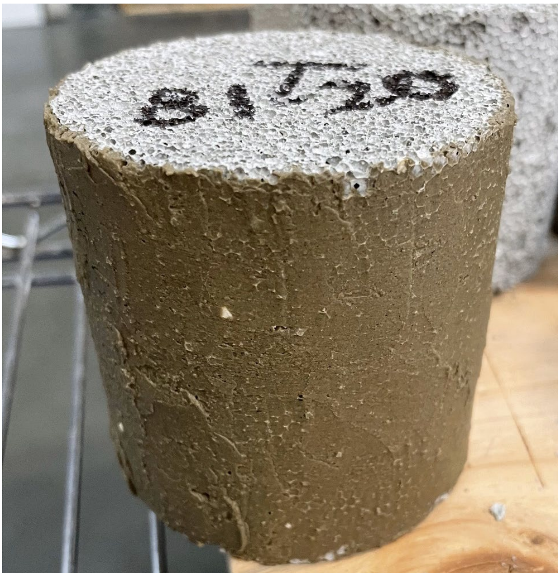
Figure 32. Photo of the LCC specimen with the bentonite gel sidewall treatment.
