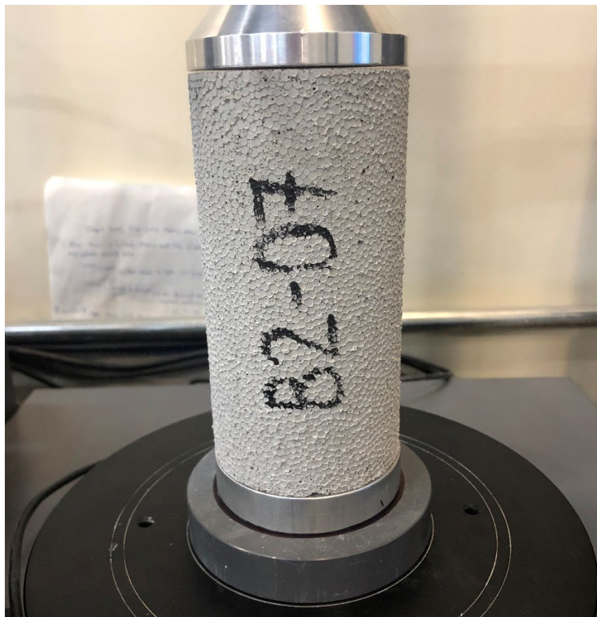
Figure 42. Photo of a specimen prepared for UCS testing in the load frame without padded end caps.
