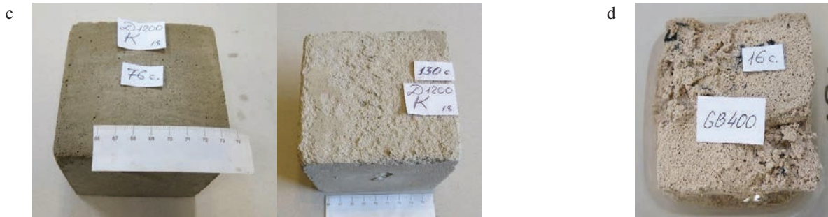
Fig. 3. (a) FC I-IV(3.6) produced in turbulence mixer after 40 cycles; (b) Gas silicate concrete after 10 cycles; (c) FC produced in turbulence mixer after 76 and 130 cycles; (d) Gas silicate concrete after 16 cycles.
