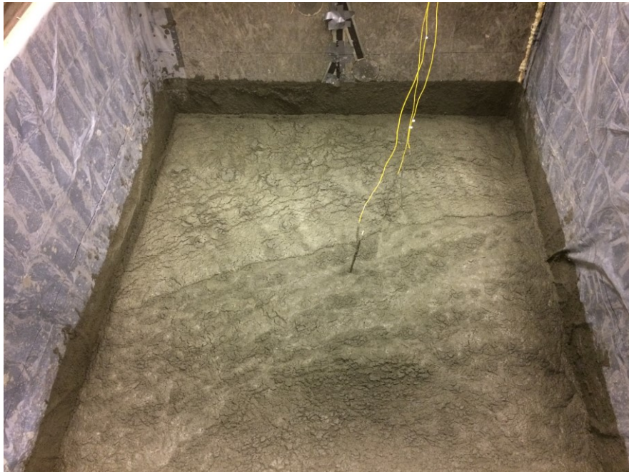
Figure 4-2: November 2019 LCC after full collapse
