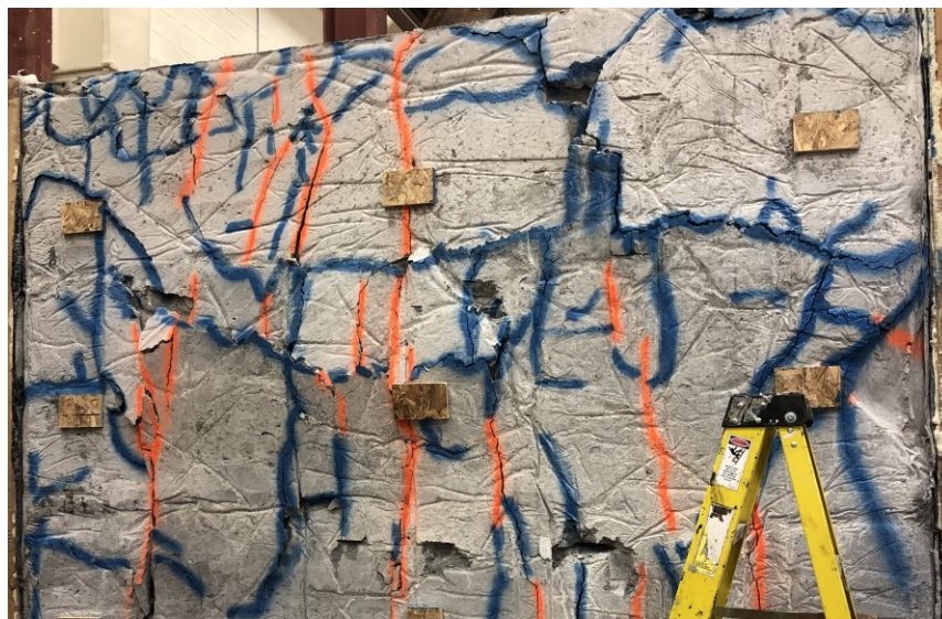
Figure 7-3: Cracking and bulging of the East face of the LCC block after the free-face test
