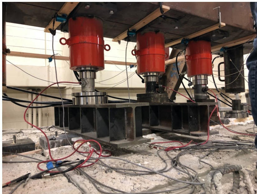
Figure 3-11: Hydraulic jacks, hemispherical platens, and load cells mounted to steel reaction beams and concrete surcharge beams.
