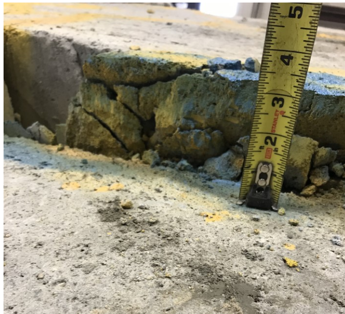
Figure 6-3: Measurement of the vertical displacement at the boundary of the surcharge beams at 6 ft behind the RCC wall
