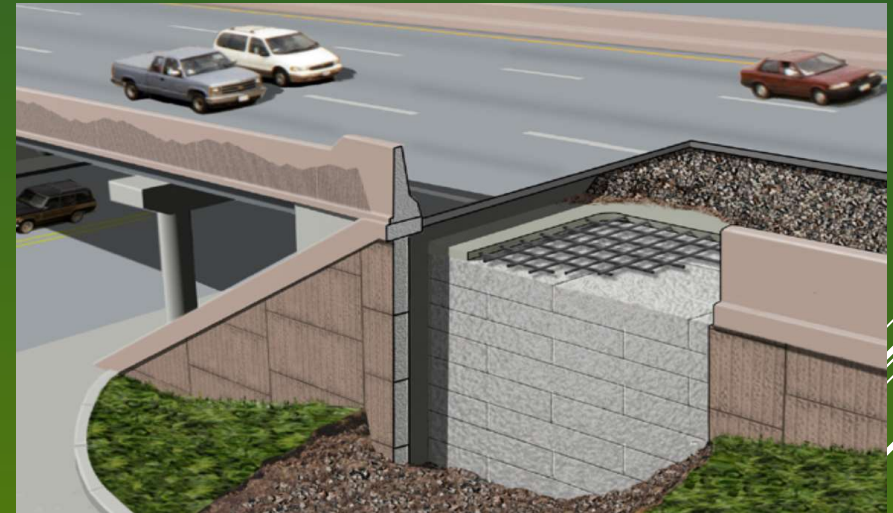
Method 2 – Vertical Embankment with concrete Load Slab and Precast Concrete Panels
