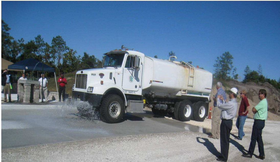
Figure 16 –Testing Drainability of Pervious concrete
