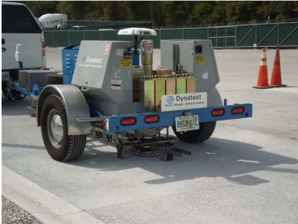
Figure 11 – FWD testing of the Pervious Test Sections
