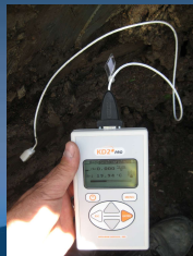
Conductivity/resistivity testing on soil (Bentham)
