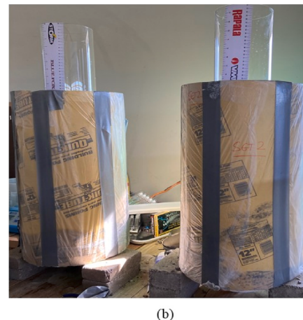
Fig. 4. Infiltration test: (a) schematic diagrams of the permeable paving with and without PLDCC; (b) the laboratory sections.
