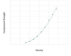
**Fig. 1.** correlation between compressive strength and the cast (wet) density of PLDCC
