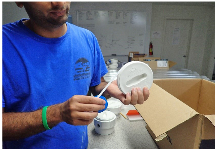
Figure 13. Teflon tape is added to the threaded PVC cap for the bottom of the siphon.
