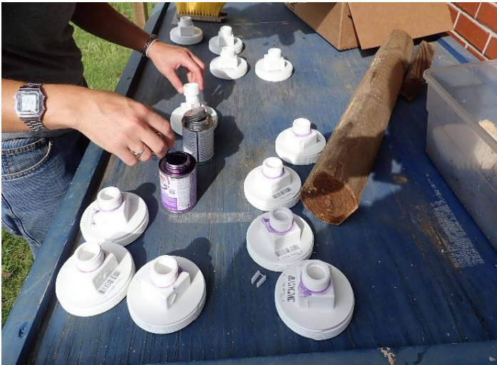
Figure 10. The repair coupling is glued to the threaded cap for the top section of the siphon.
