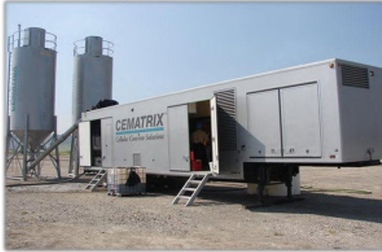
Figure 2-3: “Dry” Mix Equipment (Dolton et al., 2016)
