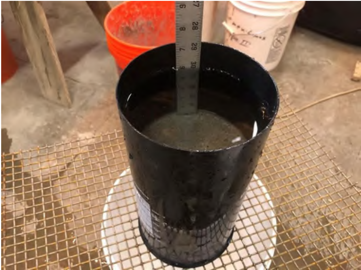
Figure15: Free draining sample. The time is recorded for the water surface to drop from the 5" mark to the 2" mark.
