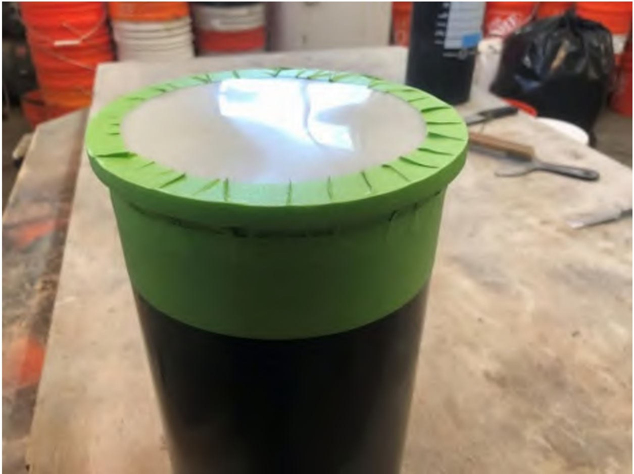
Figure 6: Mold lid taped and sealed.
