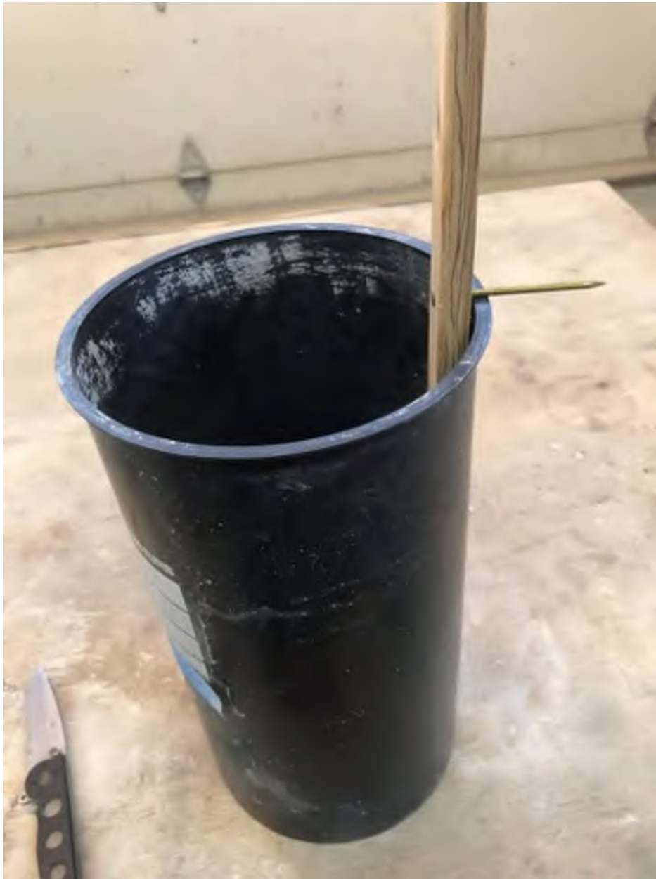
Figure 4: Scribe the line on the inside. Hold the tool against the cylinder wall, with the stop on the edge of the mold and rotate while pushing the screw against the wall.
