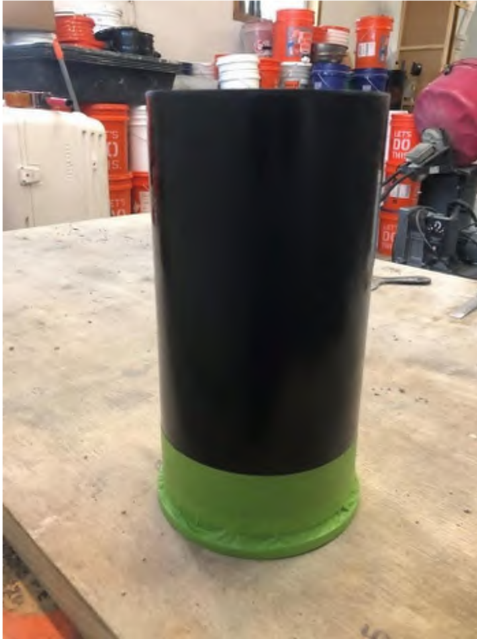
Figure 1: Modified 6x12 cylinder mold for falling head field permeability test.
