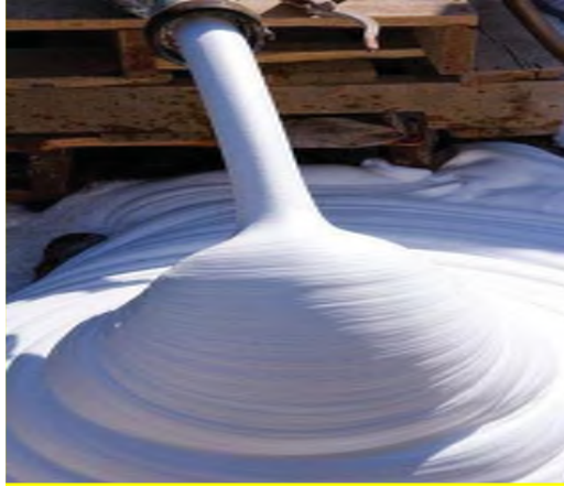
Figure 2-1: Texture of Wet LCC (Maher and Hagan, 2016)
