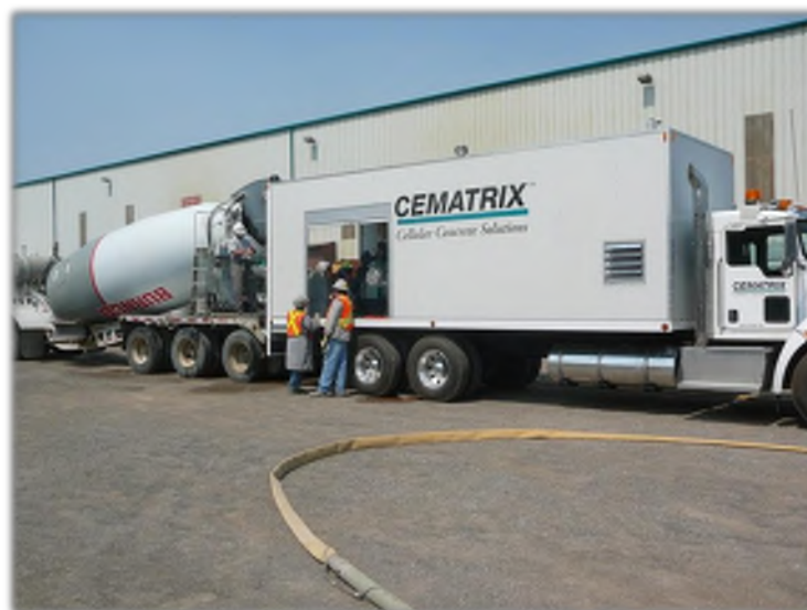
Figure 2-2: "Wet" Mix Equipment (Dolton et al., 2016)
