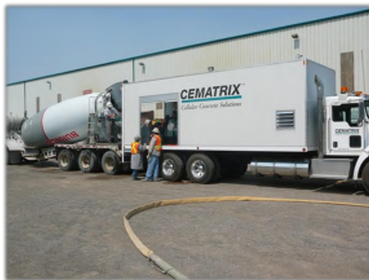
Figure 2-2: "Wet" Mix Equipment (Dolton et al., 2016)
