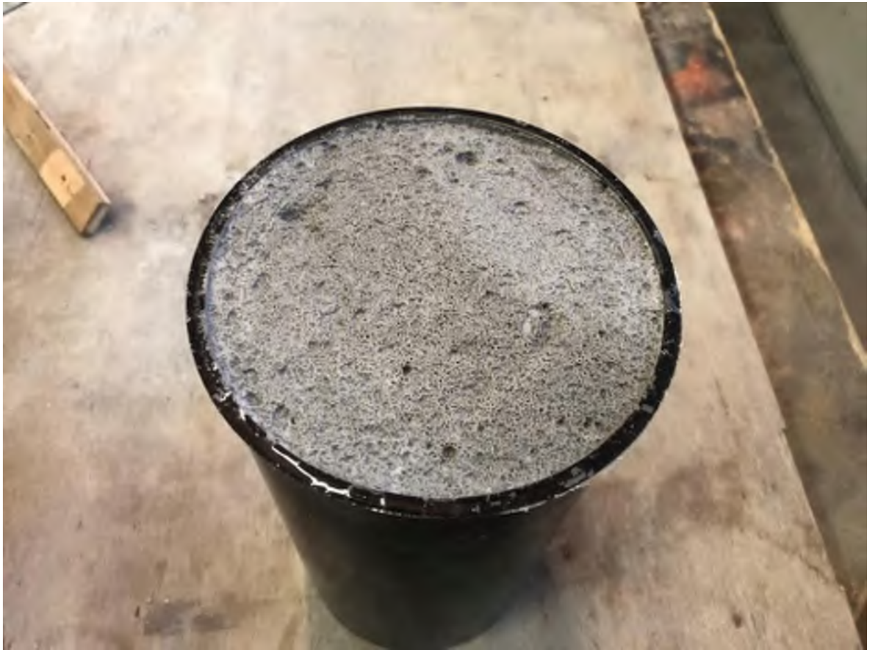
Figure 7: Lid removed, scarified bottom surface.
