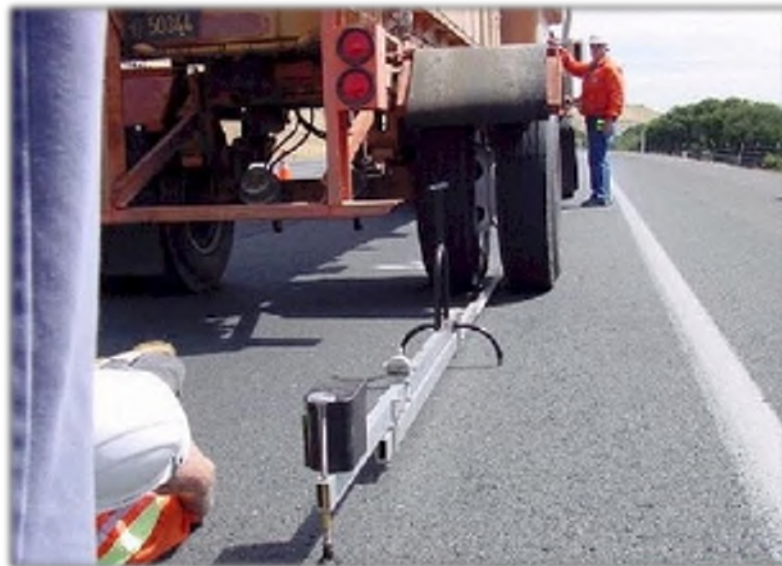
Figure 3-25: Benkelman Beam Deflection Testing
