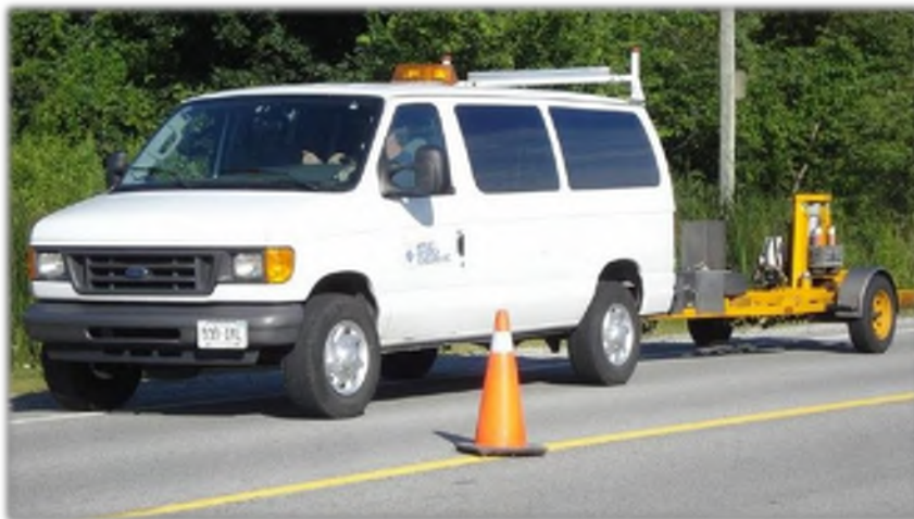
Figure 3-9: FWD Truck and Trailer (Griffiths and Popik, 2013)
