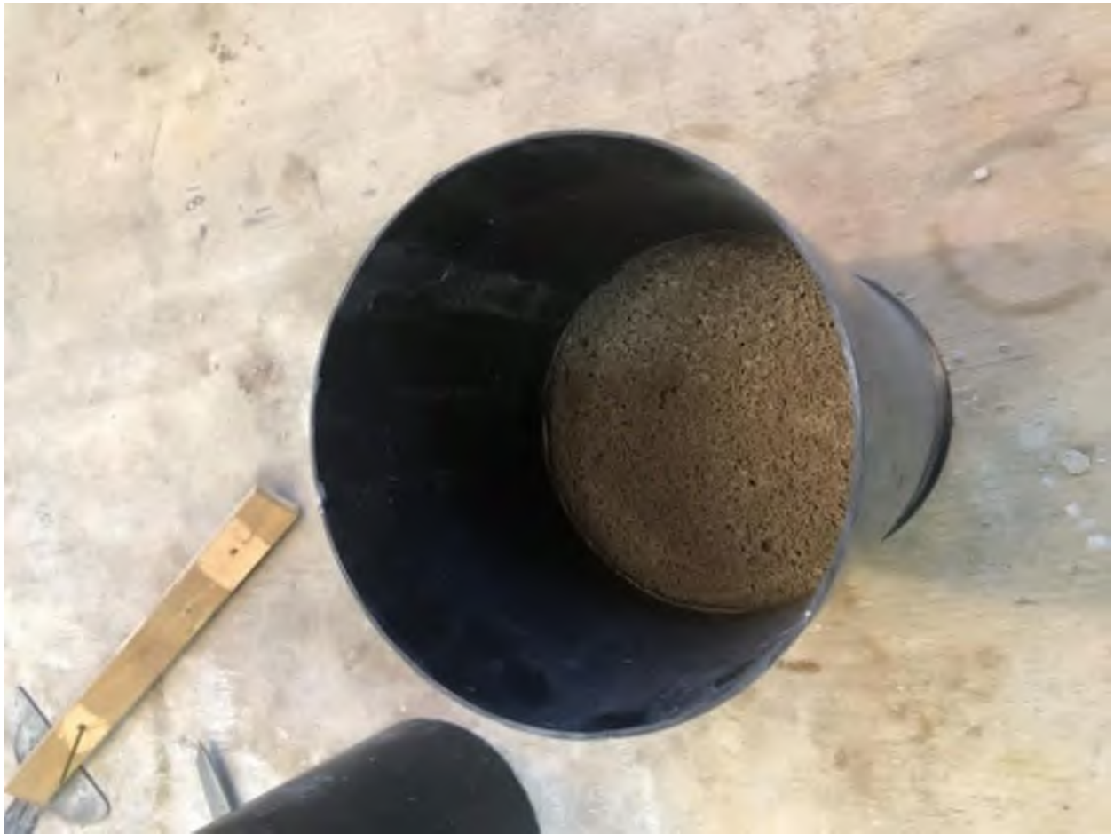
Figure 8: Scarified and cleaned top surface. Sample ready for testing.
