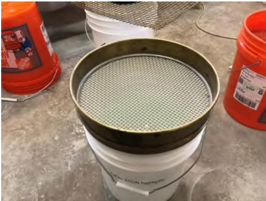
Figure 10: Empty bucket with heavy screen for draining sample, or 12" Brass Sieve Alternate
