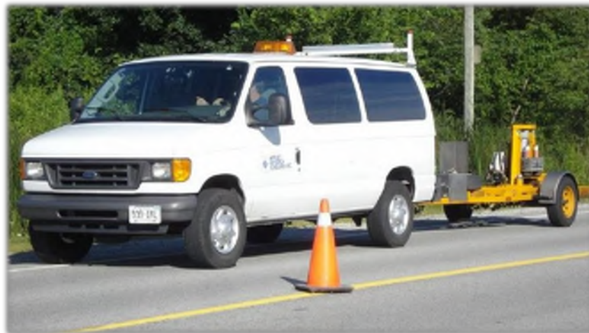
Figure 3-9: FWD Truck and Trailer (Griffiths and Popik, 2013)
