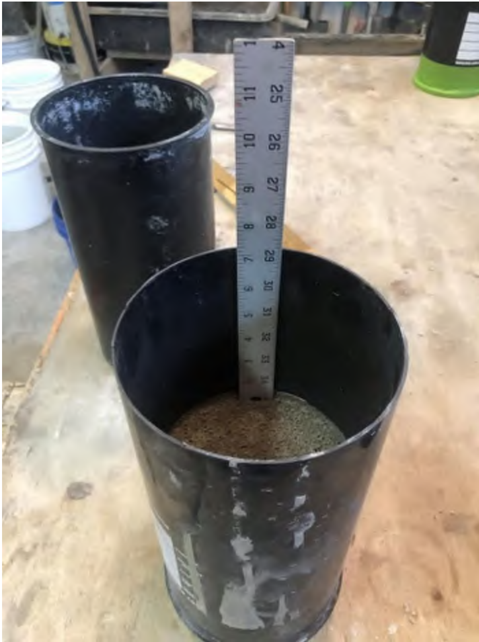
Figure 9: Ruler inserted into sample surface to a depth of one inch. The scale for the test.
