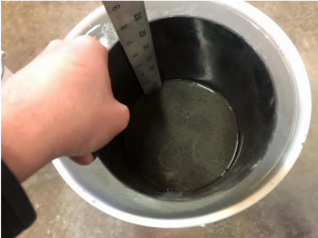
Figure 12: Water is covering the surface, now ready for total submersion.
