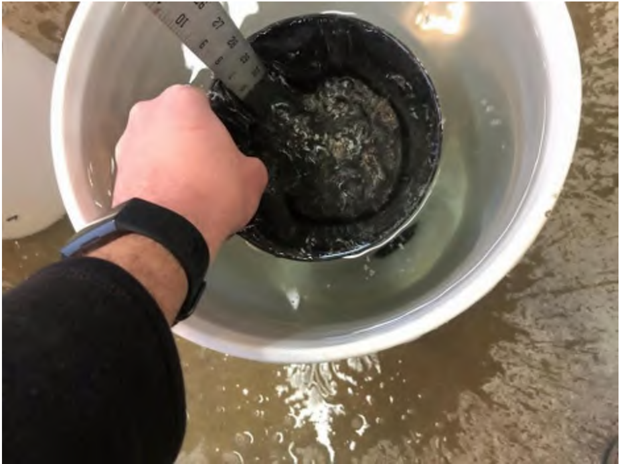
Figure13: Submerging the entire mold to full fill with water.
