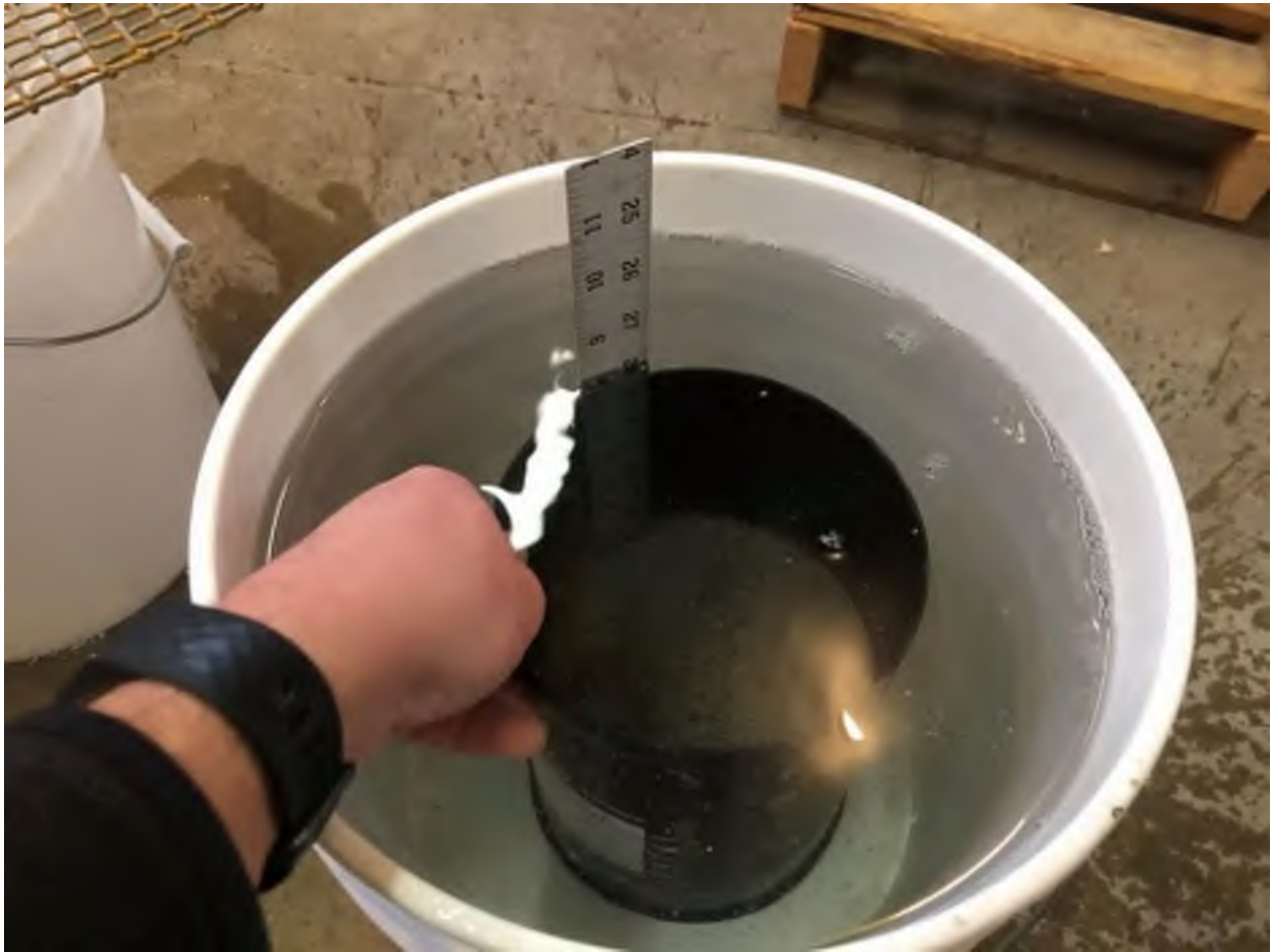
Figure14: Submerged sample, ready to be lifted out for draining and or testing.
