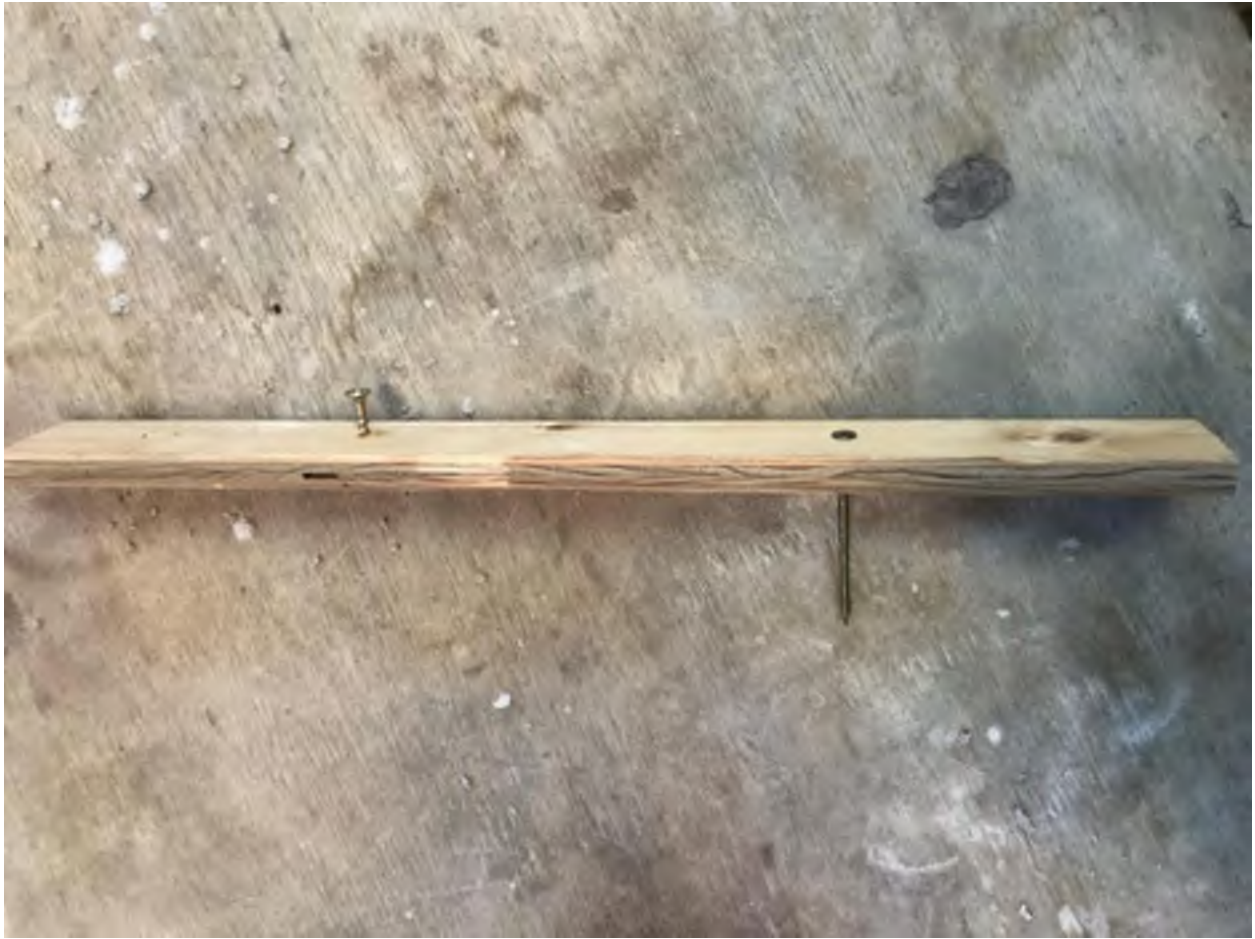
Figure 2: Scribing tool. The screw protrudes slightly through the wood and acts as the scribe. The nail acts as a stop on the cylinder rim. The distance between the center of the nail and the center of the screw is 6".
