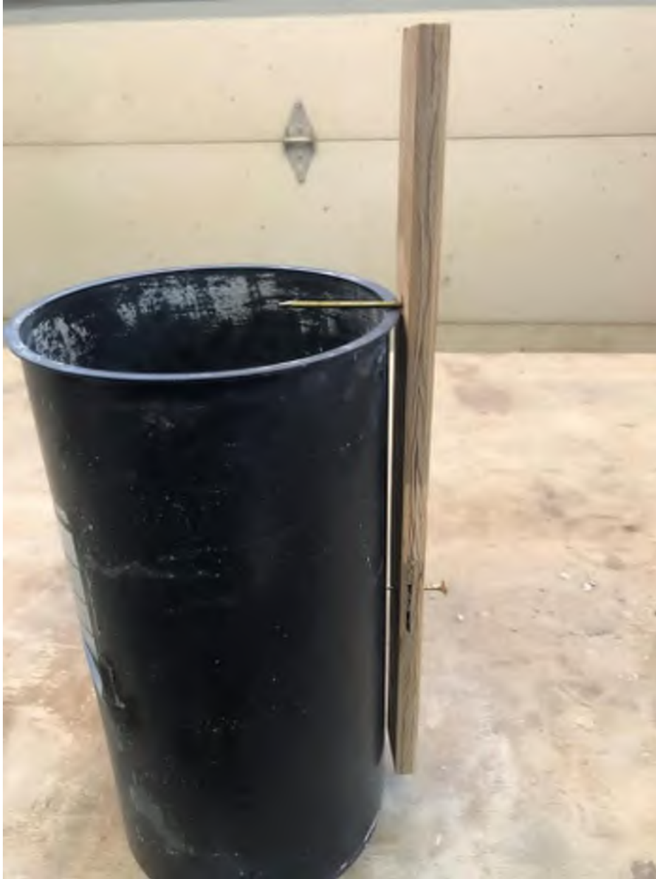
Figure 3: The nail is the stop that rides on the rim of the cylinder molds un-cut edge, the screw point scribes the line. Shown here on the outside of the cylinder for demonstration. Scribe the line on the inside.
