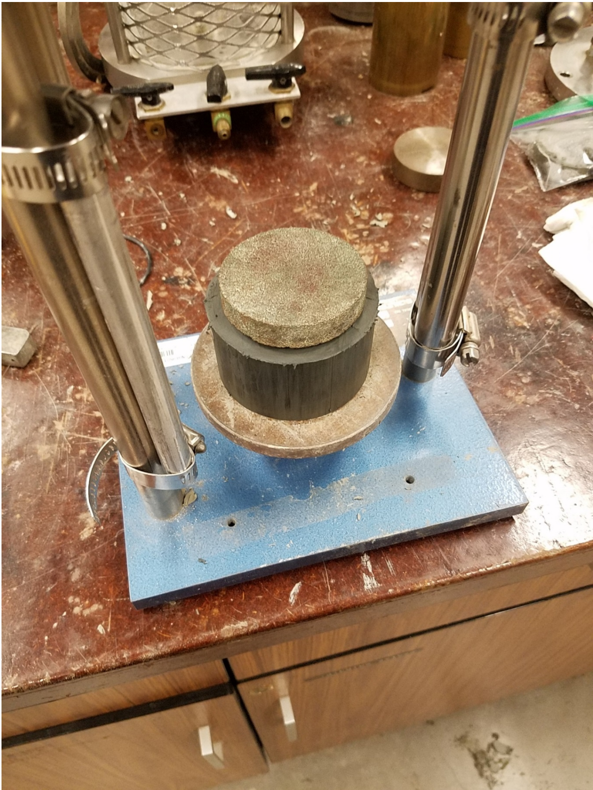
Figure 3: Portion of tube sample on the soil lathe, ready for trimming to proper diameter.
