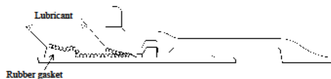
Figure 15 Application of lubricant
