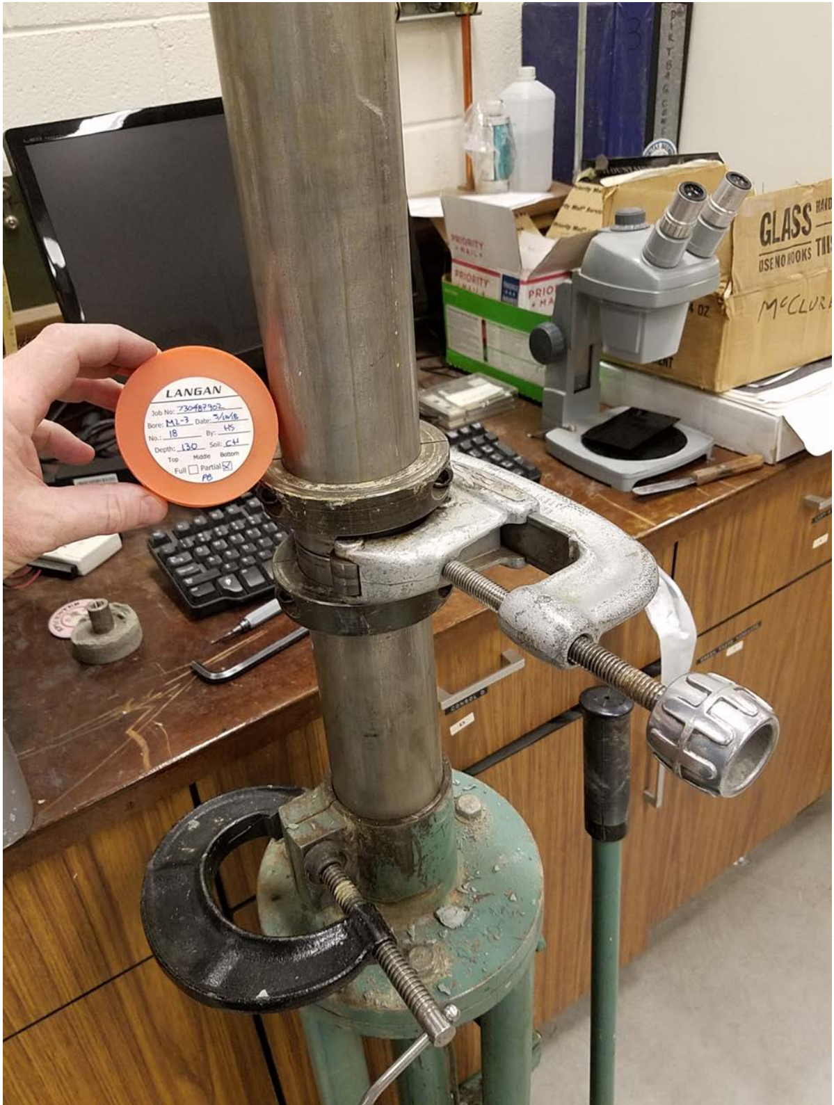
Figure 1: Cutting the sample tube using the pipe cutter and rigid stiffener rings (5M project)
