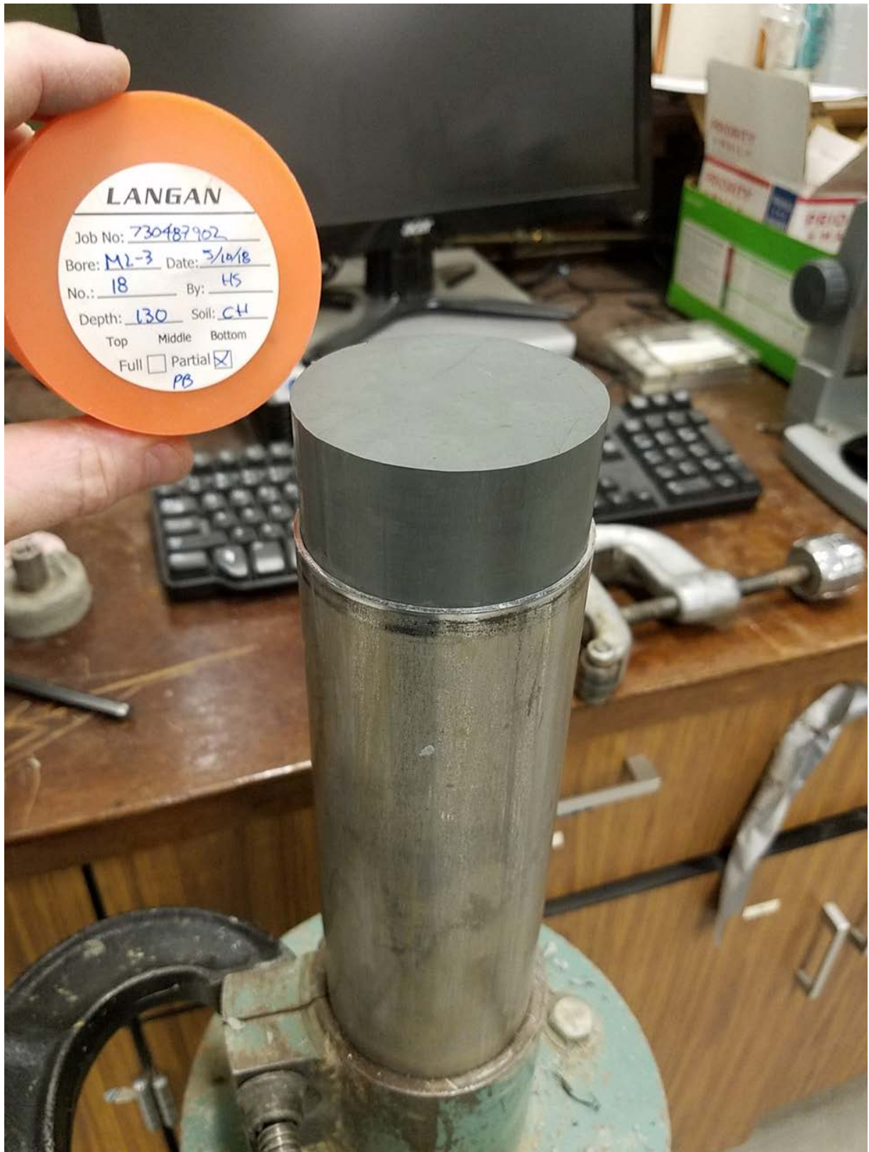
Figure 2: Extruding soil to slice and trim to prepare the consolidation specimen (5M project).
