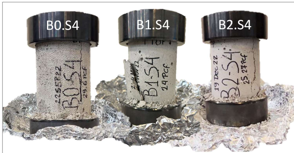
Figure 17. Samples of each batch immediately after the uniaxial compressive strength test.
