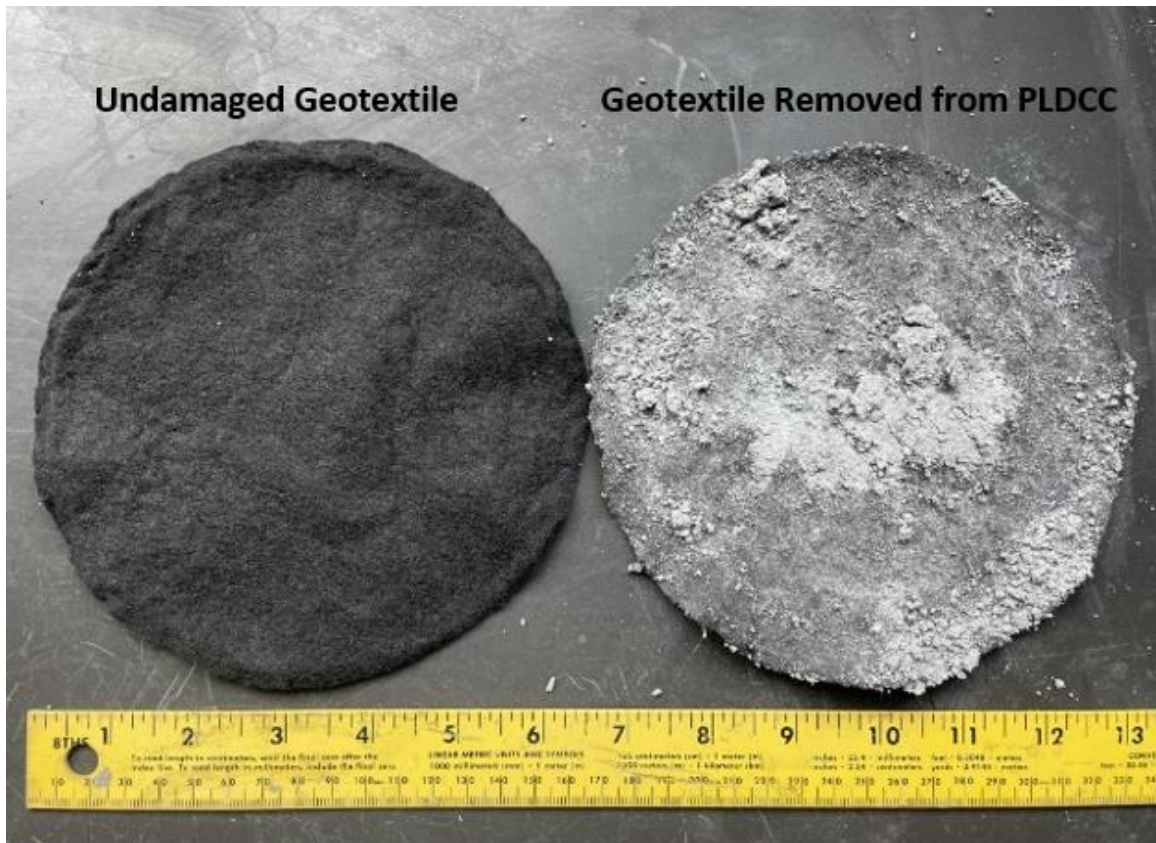
Figure 20. Undamaged Geotextile and Geotextile Removed from PLDCC.
