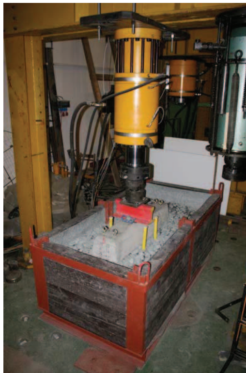
Fig. 2 Hydraulic load cylinder
