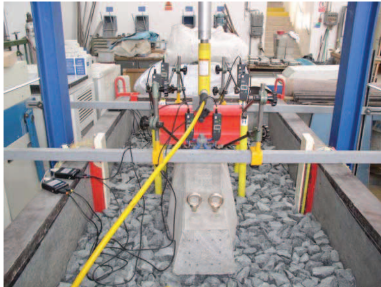
Fig. 3 Measurement of settlement under short-term loading
