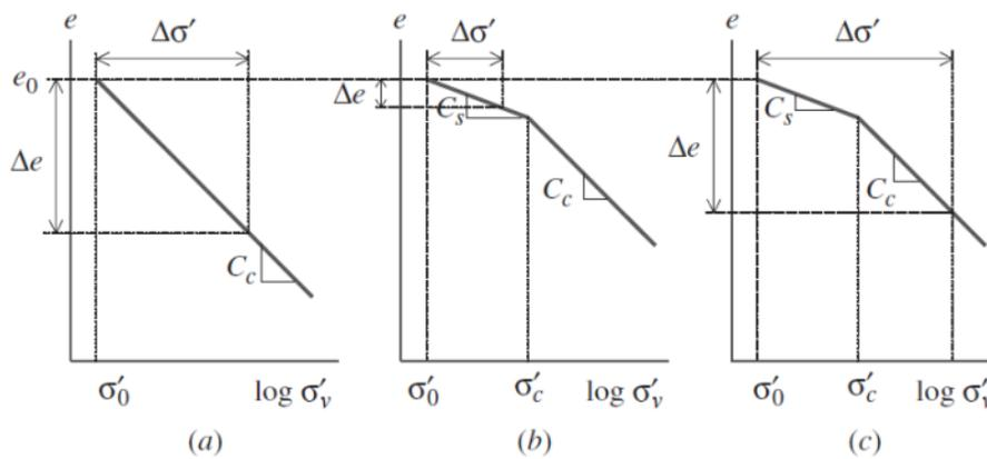
**FIGURE 4.7** Calculation of consolidation settlements: (a) NC clay; (b) OC clay with  $\Delta\sigma' + \sigma'_0 < \sigma'_c$ ; (c) OC clay with  $\Delta\sigma' + \sigma'_0 > \sigma'_c$ .
