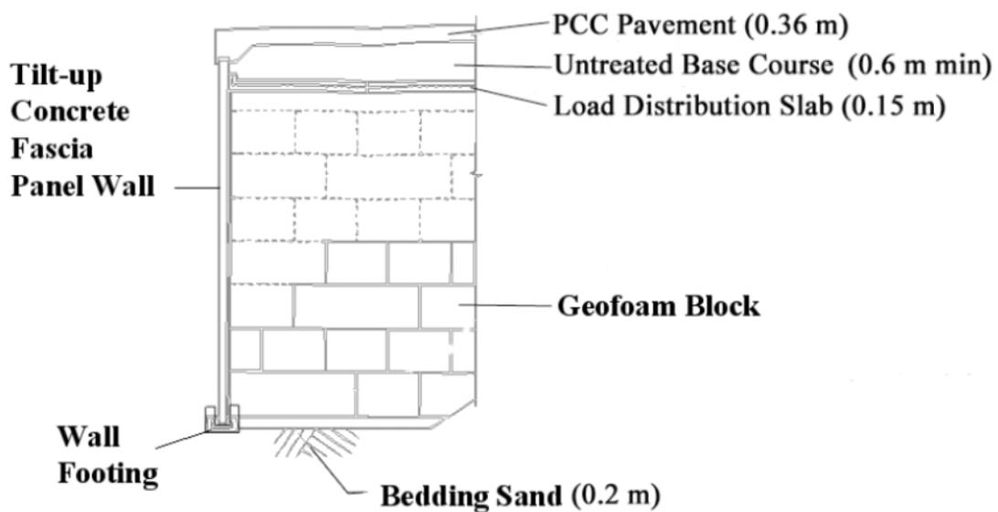
Figure 4. Typical geoforembankment cross-section used for the I-15 Reconstruction Project.
