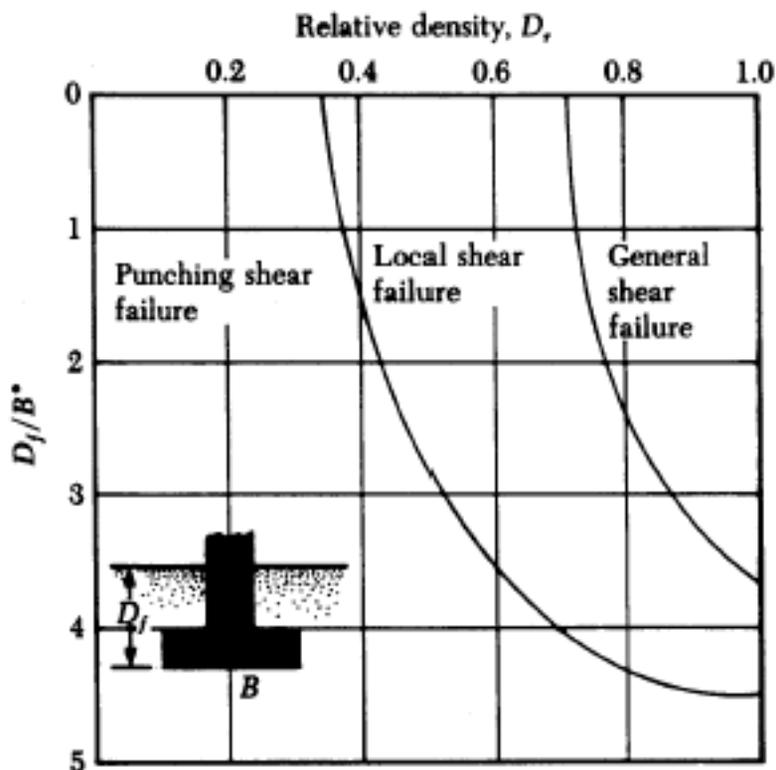
▼ FIGURE 3.3 Modes of foundation failure in sand (after Vesic, 1973)
