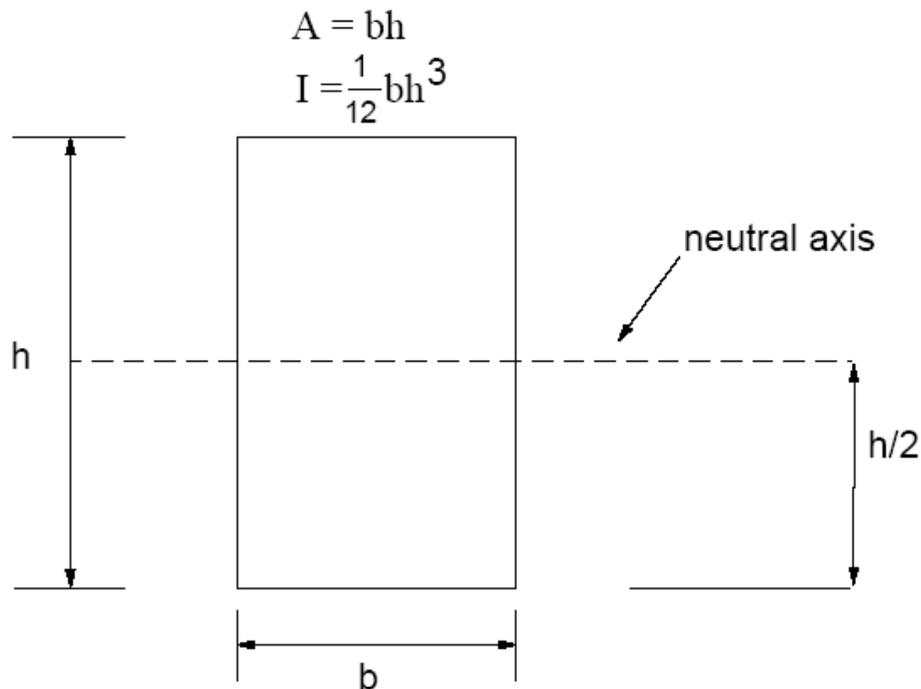
*Figure 1.3 Rectangular beam cross-section with second moment of area,  $I$ , and cross-sectional area,  $A$*
