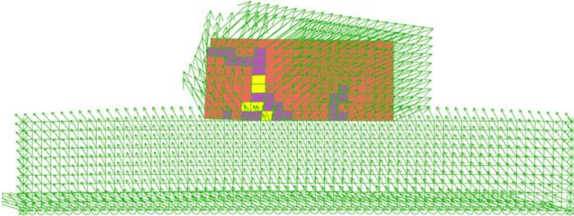
Rocking analysis of a geofram embankment undergoing earthquake excitation.
