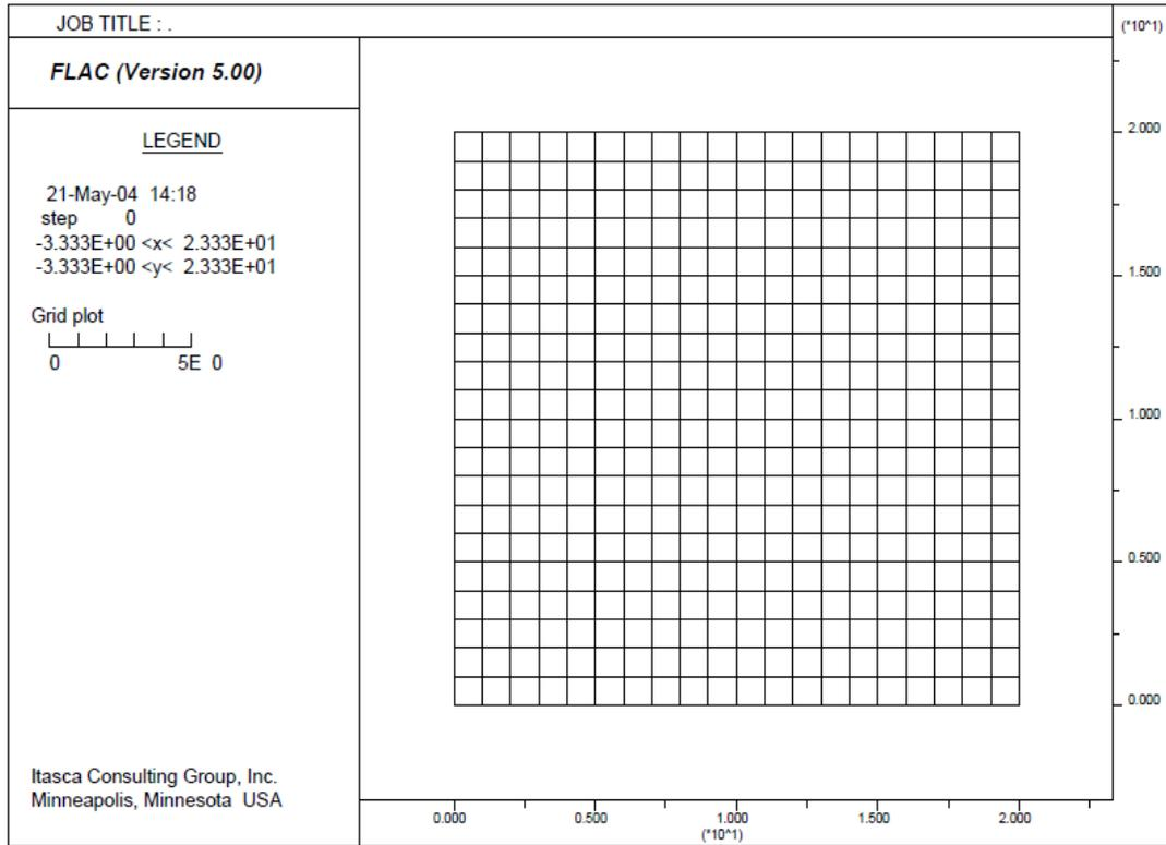
**Figure 2.37** Finite difference grid with 400 zones
