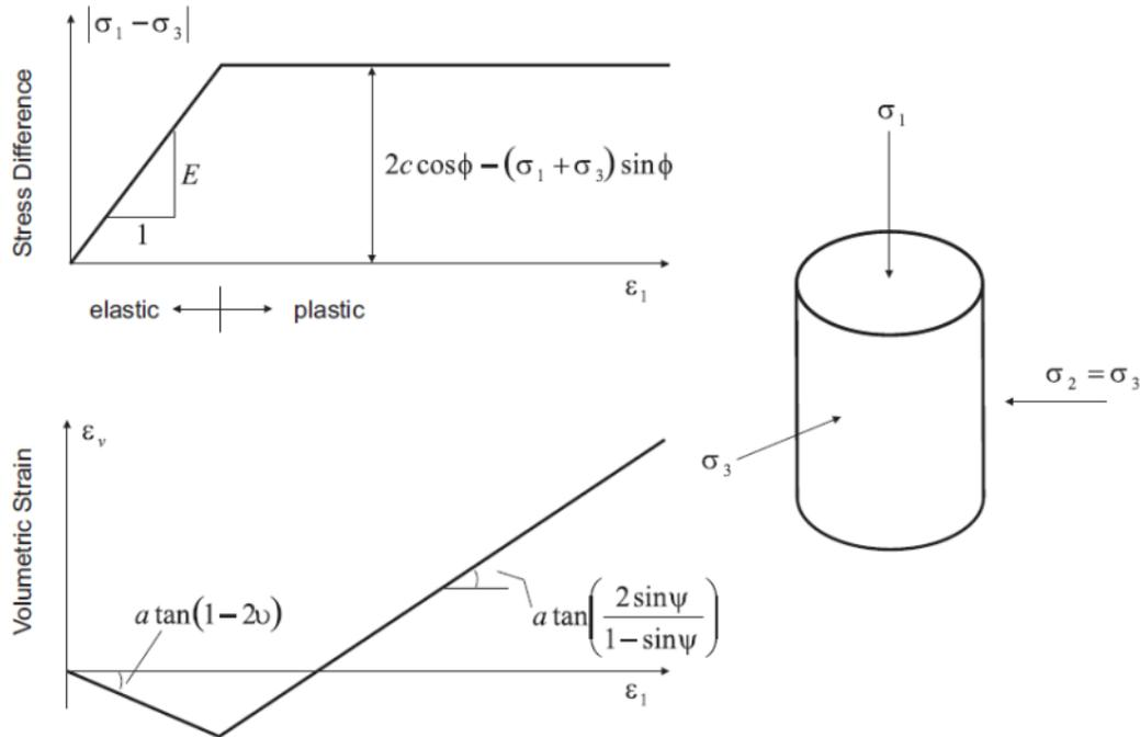
**Figure 3.58** Idealized relation for dilation angle,  $\psi$ , from triaxial test results [Vermeer and de Borst (1984)]
