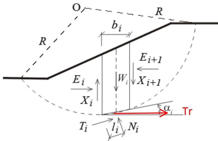
*The component of  $T_r$  that is parallel to  $N_i$  increases the normal force on the base of the slice and hence increases the frictional resistance.*
