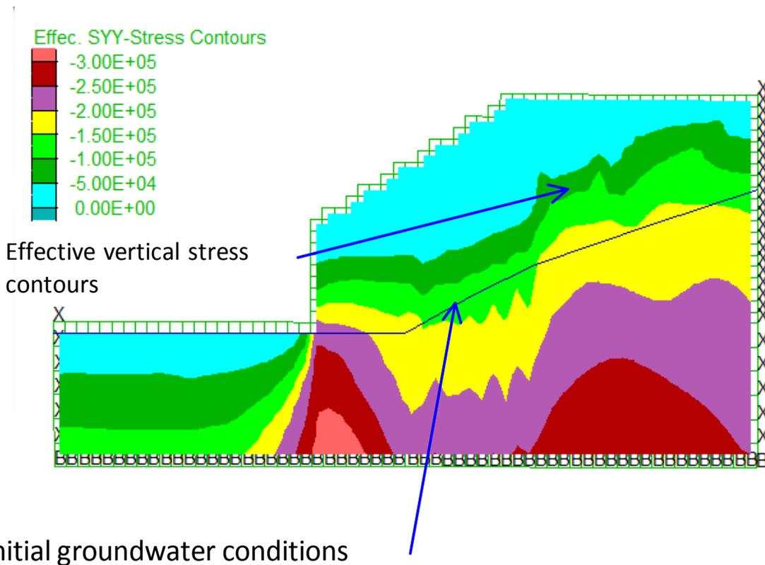
*Note that for this case, the initial effective vertical stresses were calculated by the computer model for the given boundary conditions, water table elevations and material properties.*
