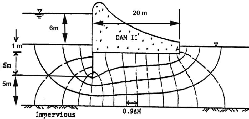
2. Use FLAC to develop a numerical model for a flow net similar to that shown above.
