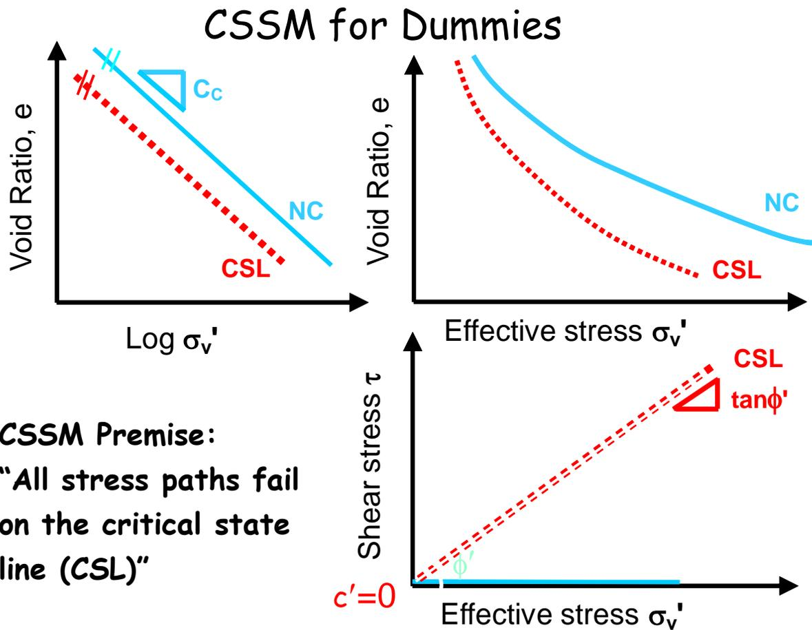
*The above statement means that the critical state line forms an envelope that defines the failure state of soil. This failure or critical state is a function of the state of stress (vertical or mean effective stress and shear stress) and the void ratio.*
