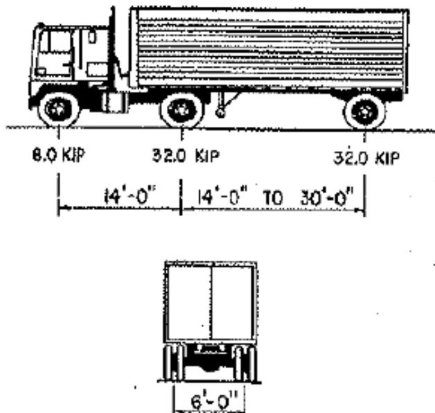
Figure 3.6.1.2.2-1 Characteristics of the Design Truck.
