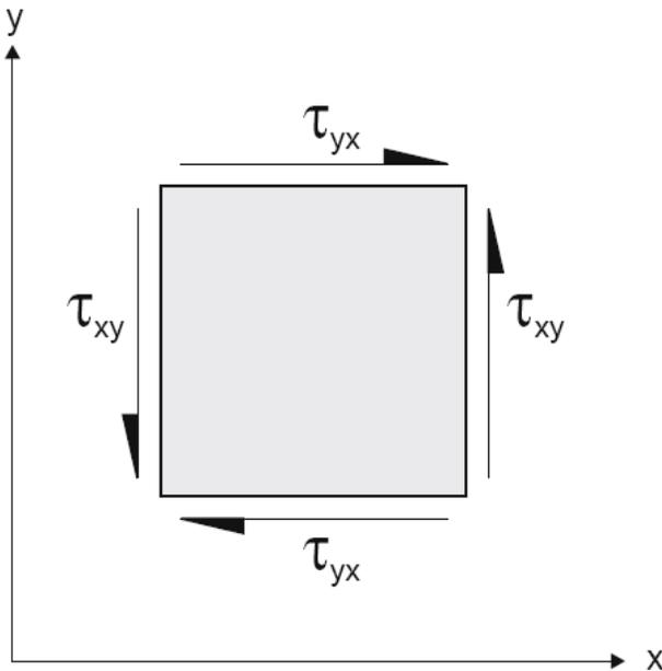
With reference to the above figure, a positive shear stress points in the positive direction of the coordinate axis of the second subscript if it acts on a surface with an outward normal in the positive direction. Conversely, if the outward normal of the surface is in the negative direction, then the positive shear stress points in the negative direction of the coordinate axis of the second subscript. The shear stresses shown in the above figure are all positive (from FLAC manual).
