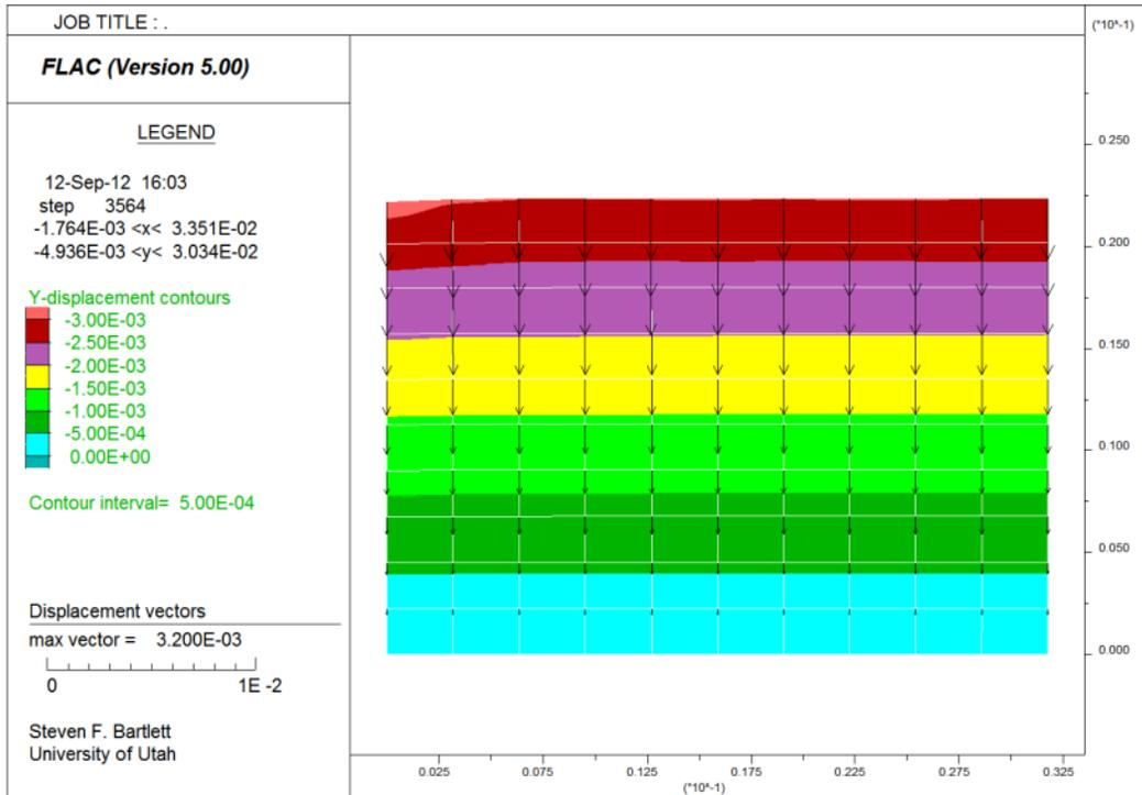
Vertical displacement vectors and displacement after applying 200 kPa, 4 tsf, stress at top of model.
