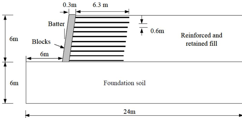
**Fig. 1. Model for limit equilibrium and numerical analyses**
