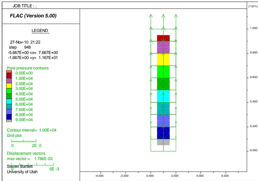
Displacement at top of model is  $1.78e^{-3}$  m.
