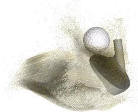
**Example of Lagrangian analysis of golf club head striking ball. Note that the tracking and movement of the sand with the striking of the ball requires a Lagrangian analysis. (from ANSYS)**
