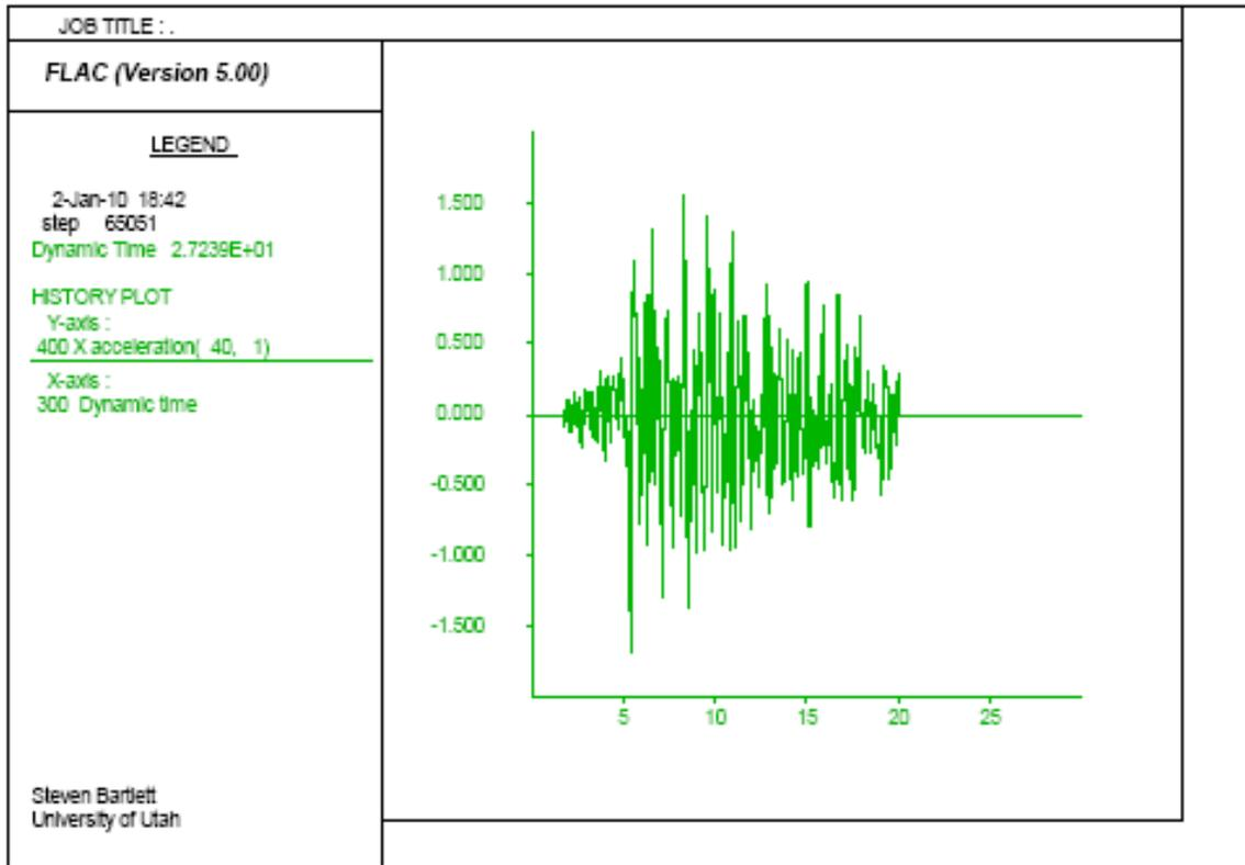
Input acceleration time history that is input into base of the model for dynamic modeling
