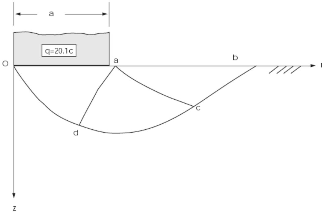
Figure 6.2 Cox slip-line net for a smooth circular footing  $\phi = 20^\circ$
