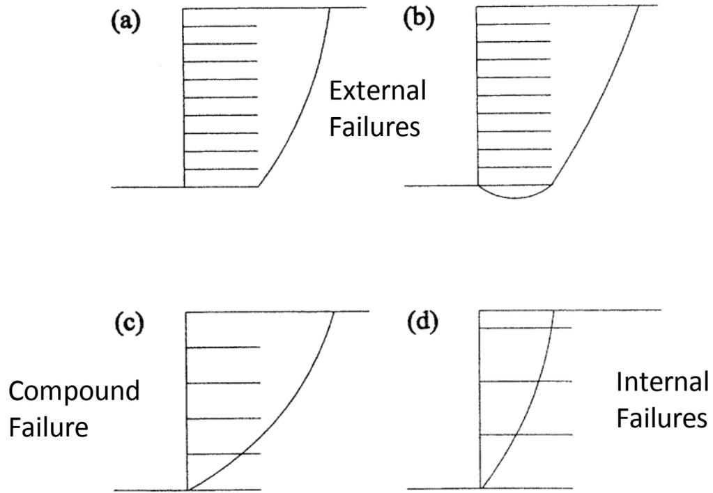
**Figure 4.3 Slip Surface Types: (a) External Slip Surface; (b) Deep-Seated Slip Surface; (c) Compound Slip Surface; (d) Internal Slip Surface.**
