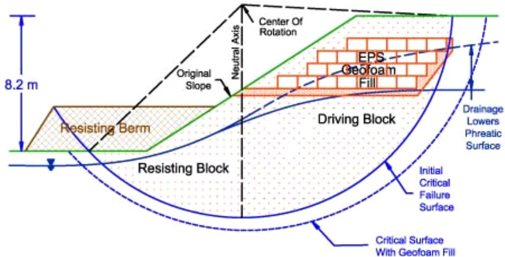
Design X-section for a landslide stabilization using EPS Geofoam
