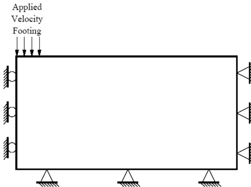
Figure 6.3 FLAC model boundary conditions
