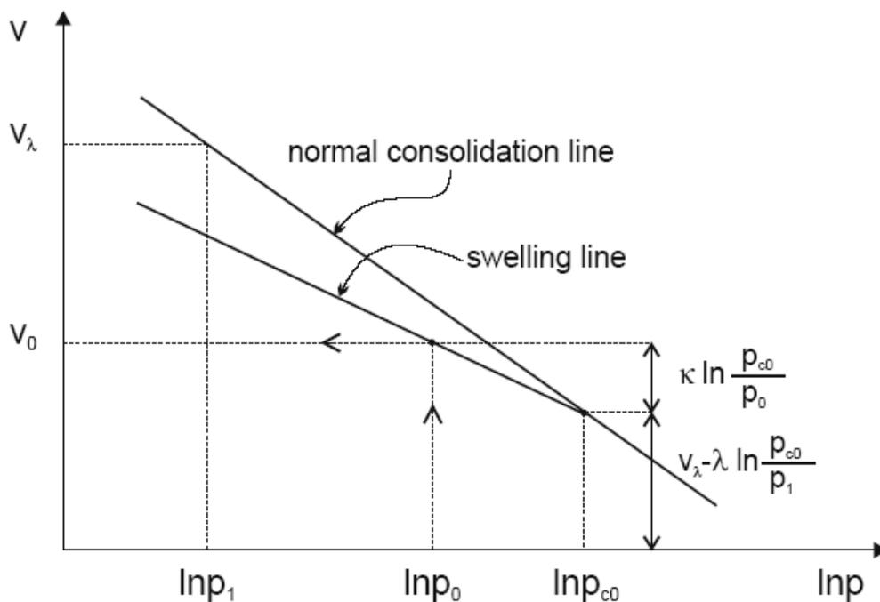
Figure 2.27 Determination of initial specific volume
