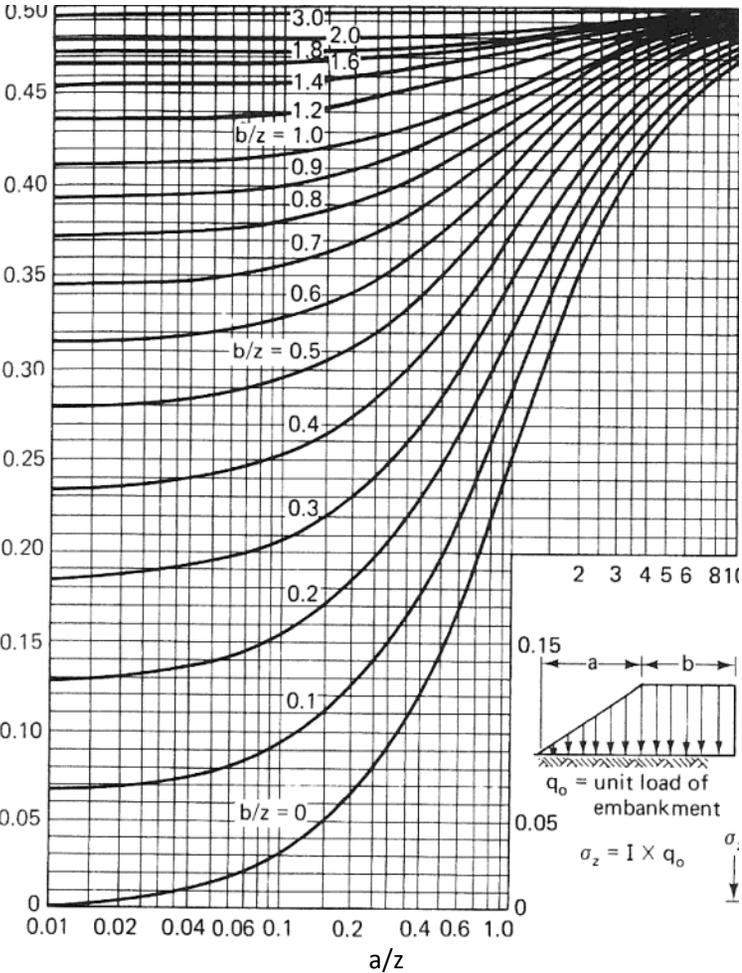
( $z =$  depth below ground surface (i.e., depth below base of embankment))
