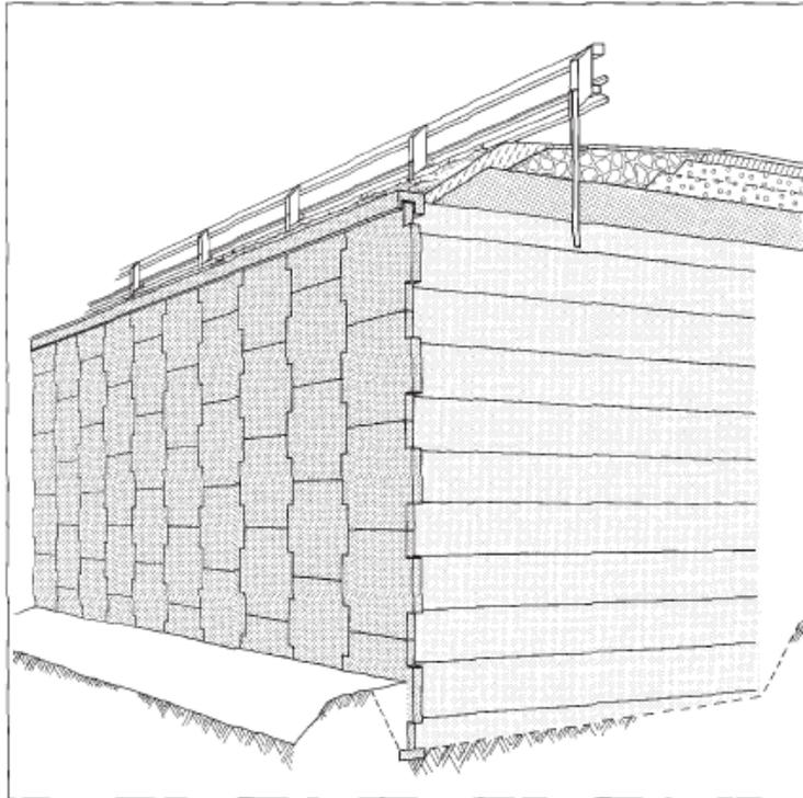
*Figure 1.75 Cut-away view of a typical reinforced earth retaining wall showing strip reinforcement*
