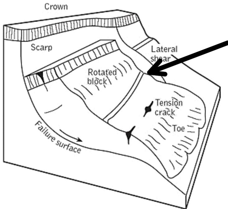
*Note that in the above drawing, the 2D plain strain condition would assume that the shear resistance on the back margin of the slide has little influence on the behavior of the landslide. If this is not true, then a 3D model would be required to capture this effect.*
