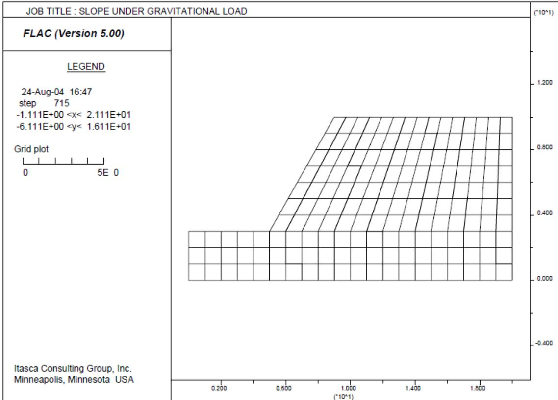
*Figure 1.1 Grid plot of initial slope*
