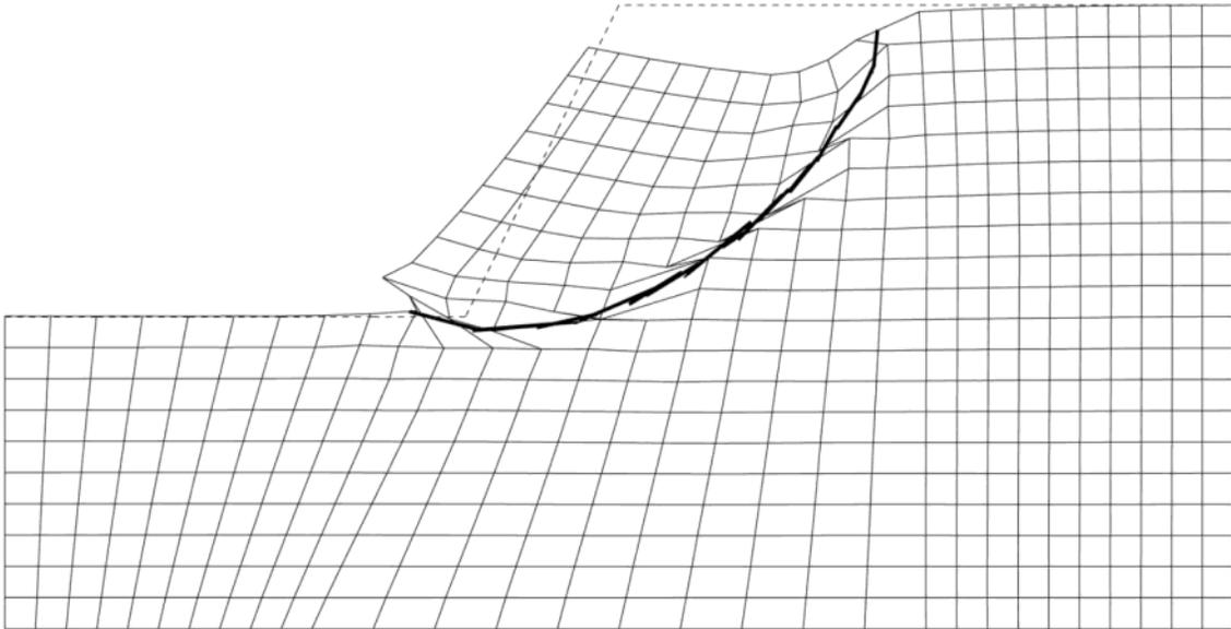
In deformation analysis we seek to estimate how much the slope will move or deform. This is much more of an involved process than simply calculating the factor of safety against failure from pseudo-static techniques.
