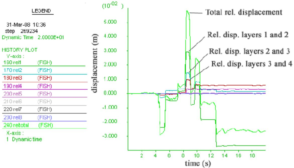
Figure 7. Relative sliding displacement plot for various geofoam layers for case 1a.
