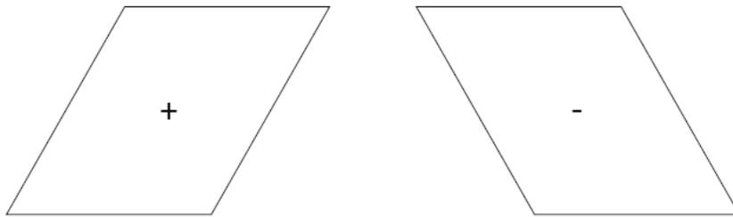
Figure 2.44 Distortion associated with positive and negative shear strain
