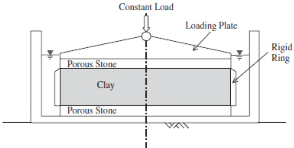
**FIGURE 4.3** One-dimensional consolidation test apparatus.
