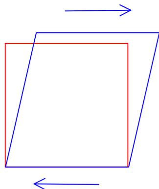
Dilatancy during shear. Note that the unit square has undergone distortion and volumetric strain (change in volume).
