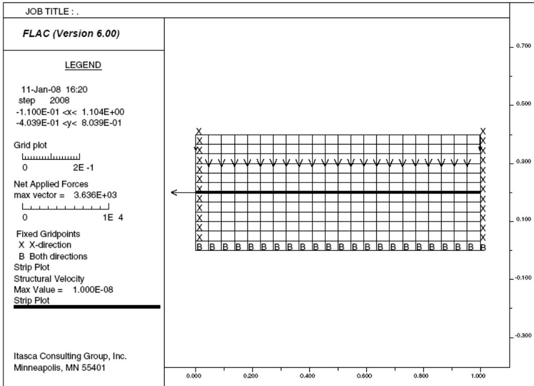
*Figure 1.81 Strip element in grid: vertical confining pressure and x-velocity applied at end node*
