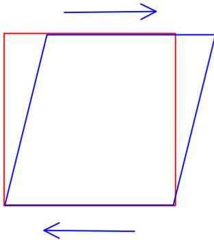
No dilatancy, dilatancy angle = 0. Note that the unit square has undergone distortion solely.
