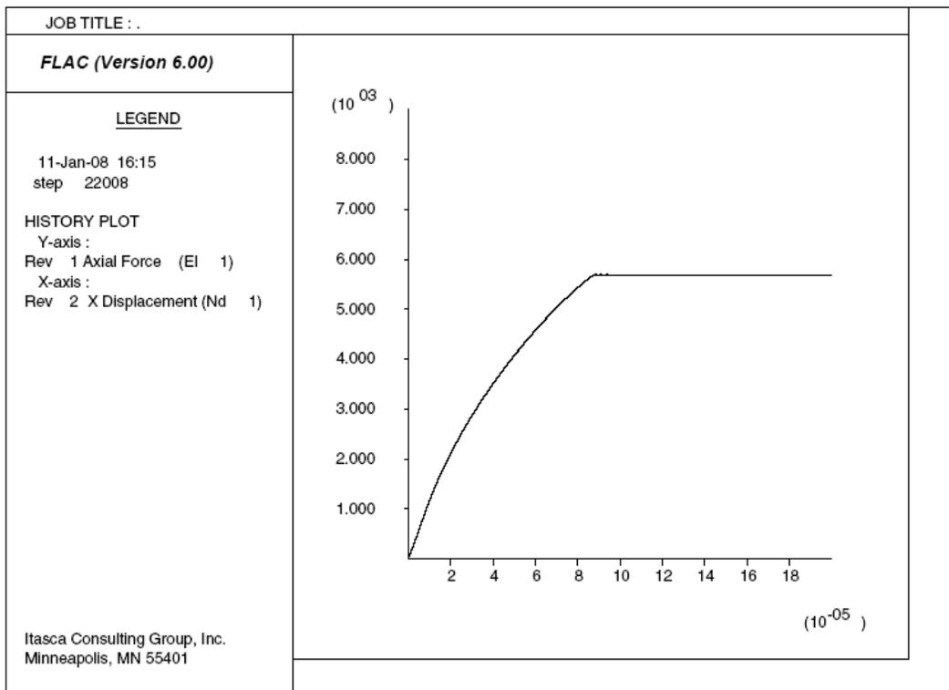
Figure 1.83 Strip axial force versus axial displacement – sigc0 = 70 kPa
