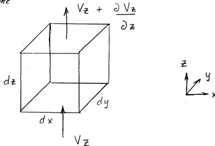
$v_z$  = velocity of fluid flow in  $z$  direction into unit volume
