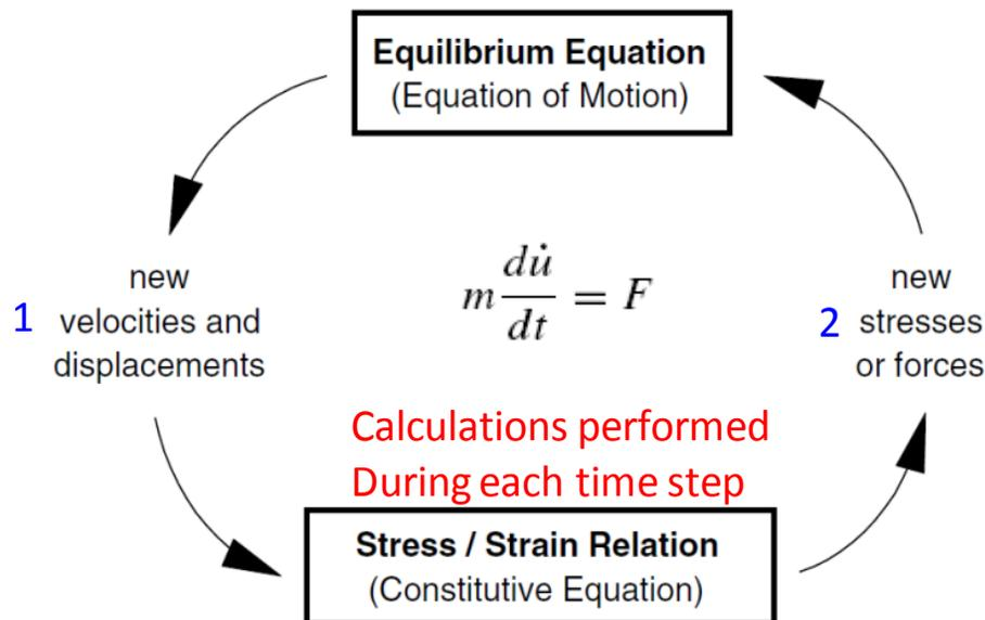
Figure 1.1 Basic explicit calculation cycle
