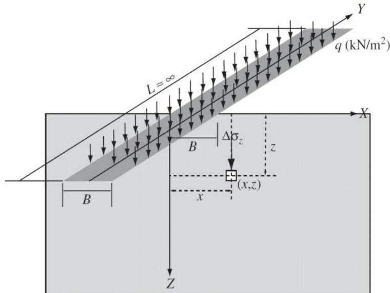
FIGURE 3.25 Stresses caused by a strip load.
