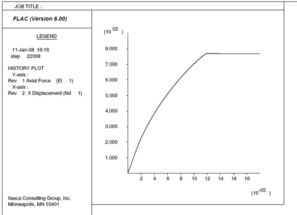
Figure 1.82 Strip axial force versus axial displacement – sigc0 = 120 kPa
