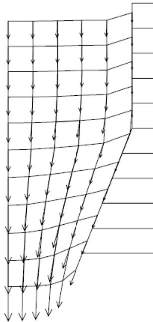
*Figure 4.11 Flow of frictional material in a “bin”*
