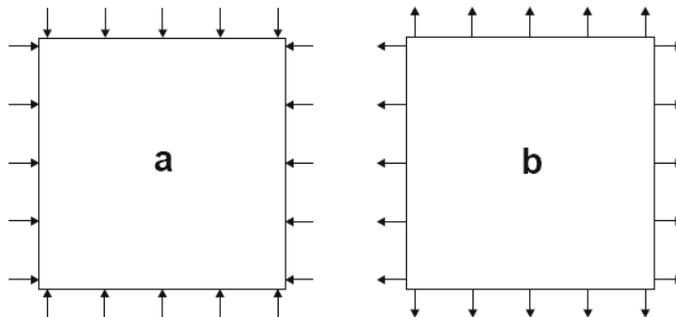
Figure 2.45 Mechanical pressure: (a) positive; (b) negative
