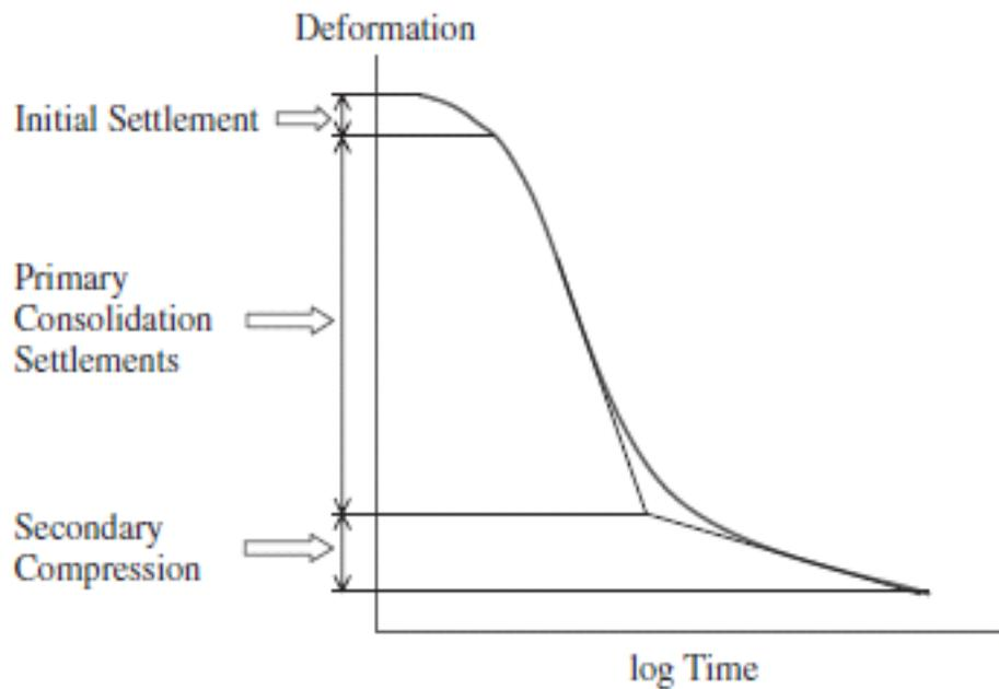
**FIGURE 4.4** Deformation versus time curve (semilog).
