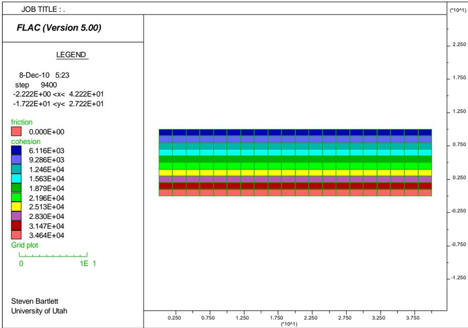
Note how the undrained cohesion varies with depth to account for changes in the mean effective stress.
