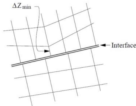
Figure 4.7 Zone dimension used in stiffness calculation
