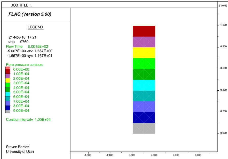
Pore pressure for saturated layer (Pa)
