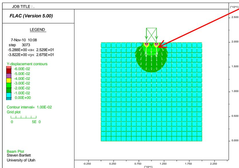
Note: High displacement occurs under walls of frame because of flexible floor. This shows soil-structure interaction in that the flexibility of the structure changes the stress distribution in the soil.
