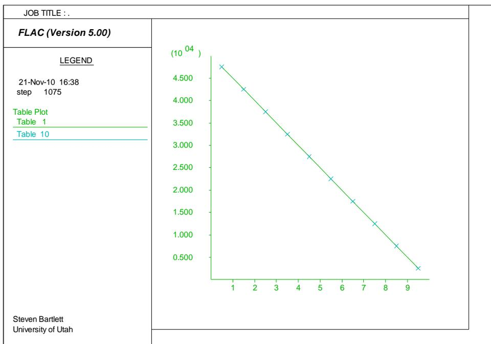
Vertical stress (Pa) versus elevation (m) for dry layer
