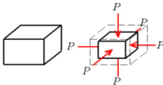
where  $P$  is [pressure](#),  $V$  is volume, and  $\partial P / \partial V$  denotes the [partial derivative](#) of pressure with respect to volume. The inverse of the bulk modulus gives a substance's [compressibility](#).
