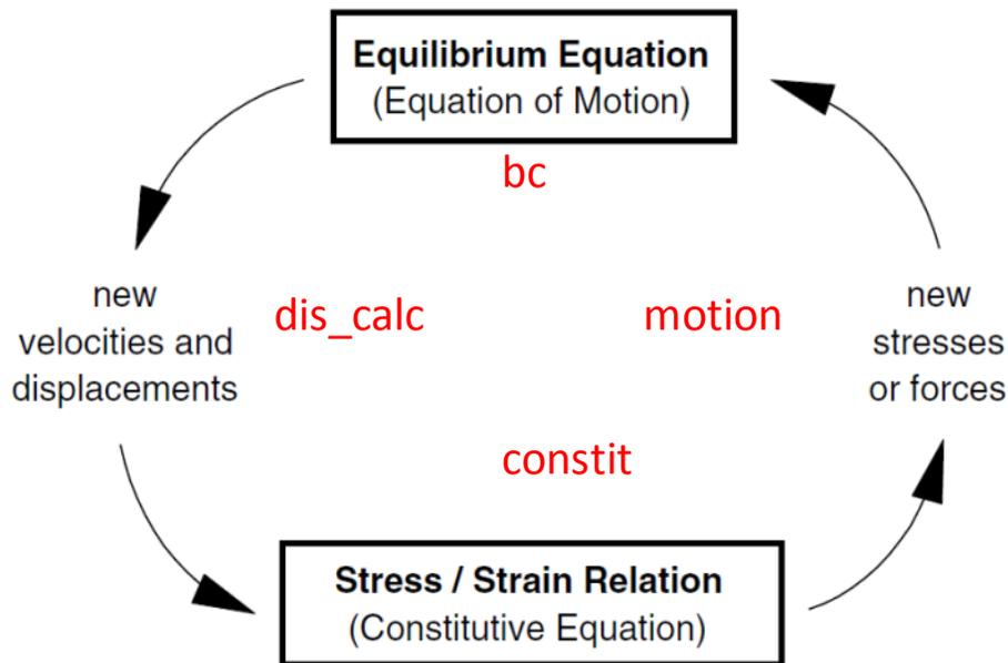
Figure 1.1 Basic explicit calculation cycle
