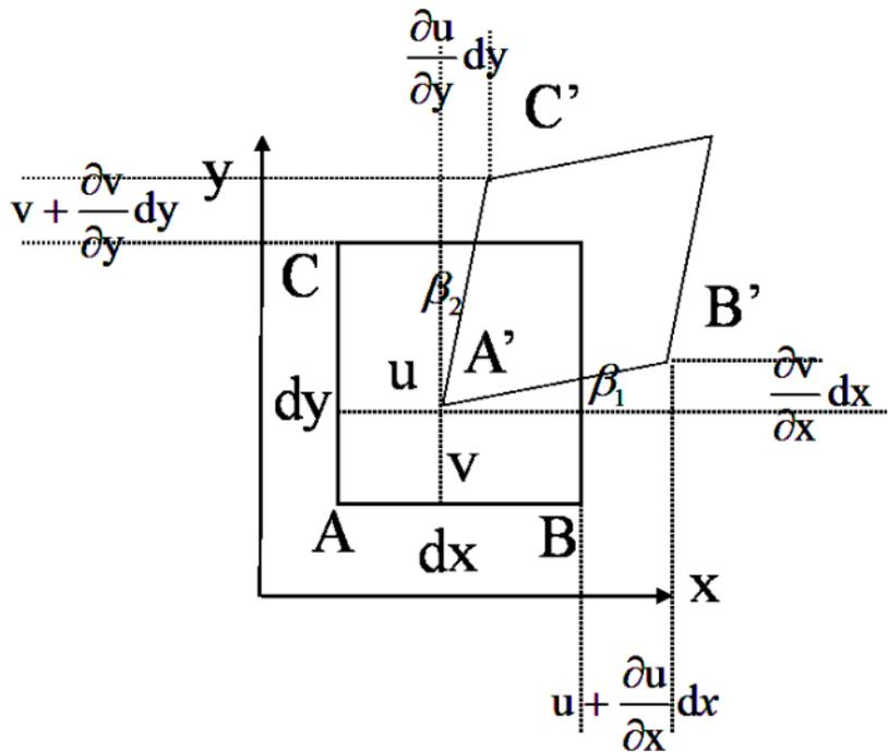
Note that the square shown below has undergone translation, deformation and distortion
