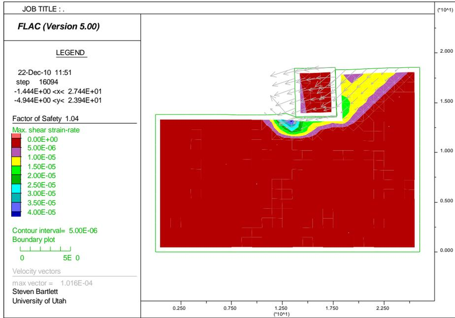
Factor of Safety for global stability = 1.04, friction angle = 20 deg.,
