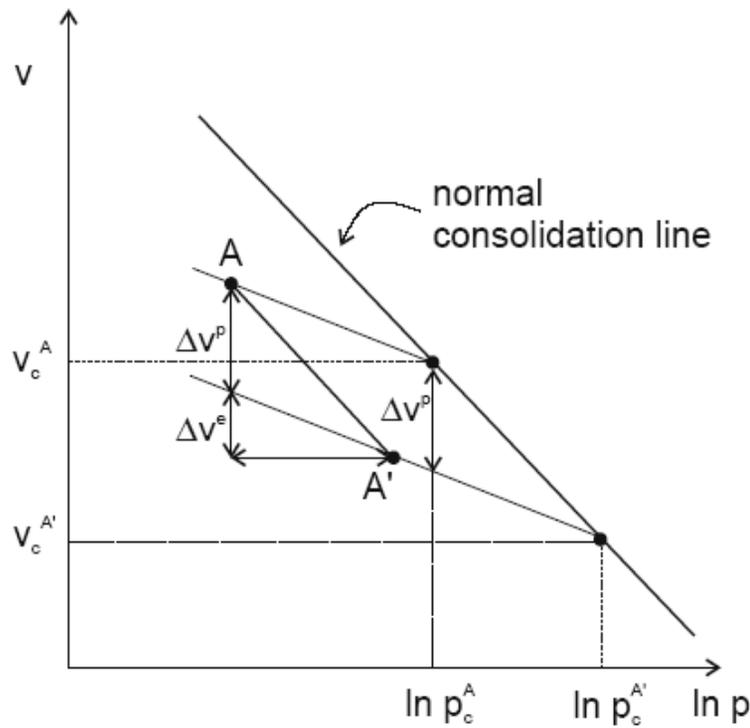
*Figure 2.25 Plastic volume change corresponding to an incremental consolidation pressure change*
