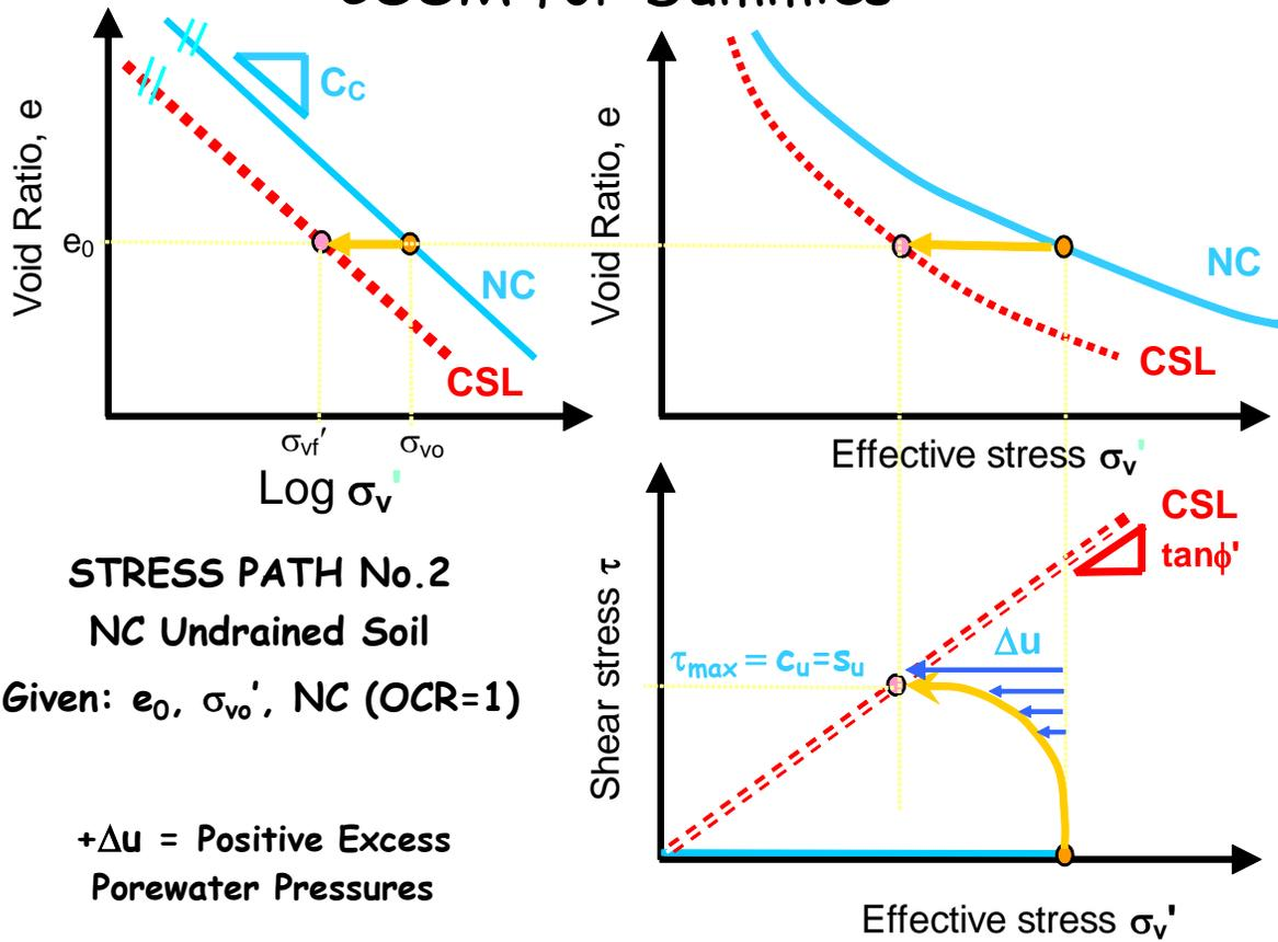
Note that there is no change in void ratio in the above consolidation plots because the *test is undrained*.
