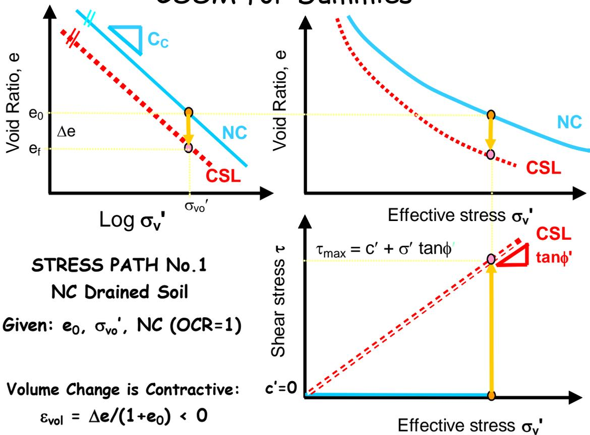
*The above stress path is straight because there is no excess pore pressure generated during shear because the **test is drained** and the applied vertical stress is not changing during the direct shear mode of failure.*
