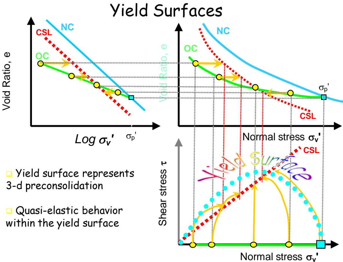
The behavior of the soil is elastic until the state of stress on the soil reaches the yield surface. After that, the soil behaves in a plastic manner and undergoes both elastic and plastic strains. The yield surface will expand as the soil dilates or strain hardens: it will contract as the soil contracts or strain softens until the critical state is reached. At this point, this yield surface no longer changes and is known as the yield surface at critical state.
