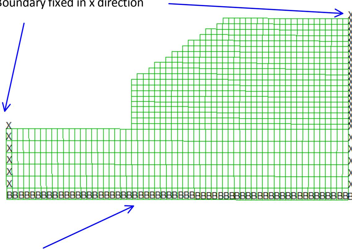
Boundary fixed in x and y direction (i.e., B is used to indicate boundary is fixed in both directions).
