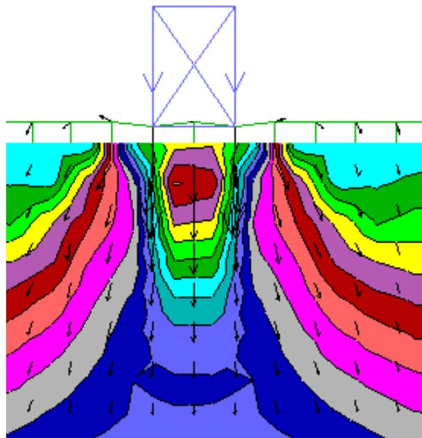
Vertical stress profile underneath structural frame with  $-7 \times 10^5$  N load on each wall.
