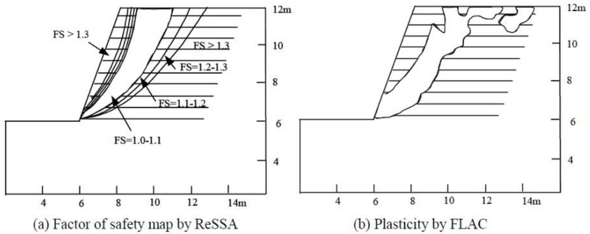
**Fig.3. Spatial distribution of factors of safety and plasticity (20° batter MSE wall)**
