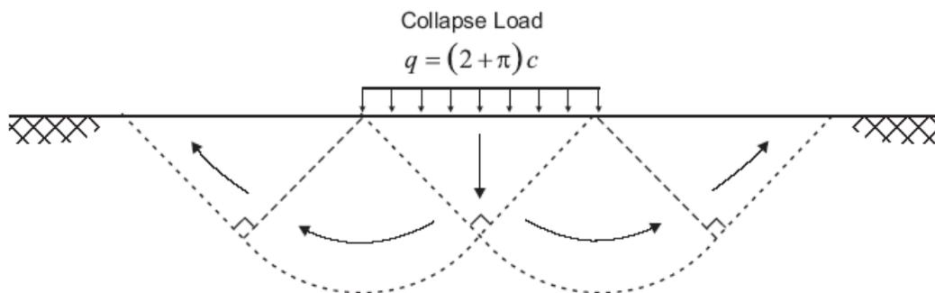
*Figure 6.1 Prandtl's wedge problem of a strip footing on a frictionless soil*
