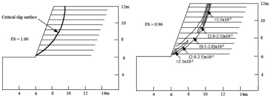
(a) Critical slip surface and FS by ReSSA      (b) Maximum shear strain rate and FS by FLAC
