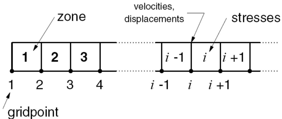
Numbering scheme for a 1-D body using FDM.
