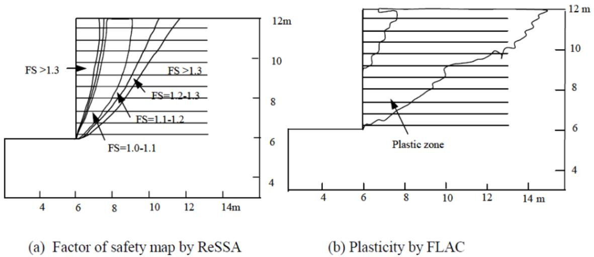
**Fig. 2. Spatial distribution of factors of safety and plasticity (vertical wall)**
