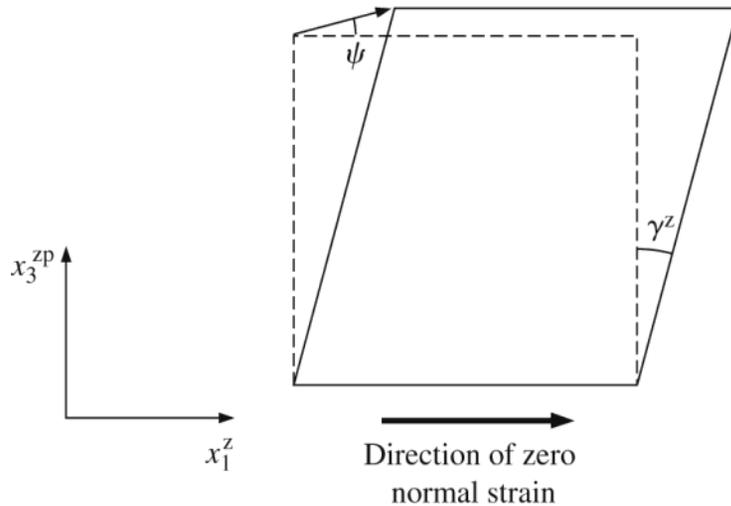
This element is dilating during shear. **This is plastic behavior.**
