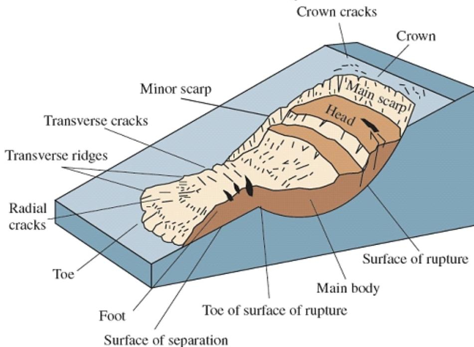
In the case of a rotational slump (above) the sides of the landslide have significant impact on the sliding resistance and this requires a 3D model.
