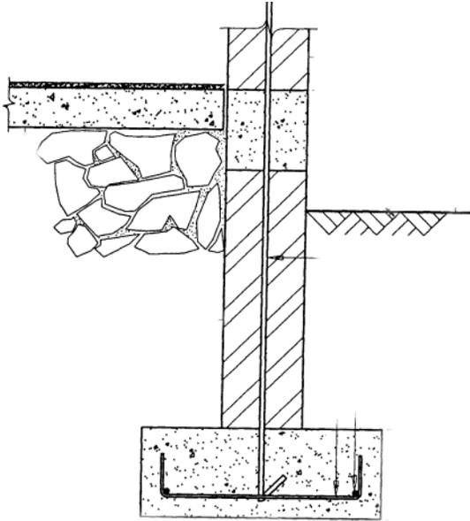
*Note: To be a plane strain condition, the loading to the footing must be uniform along its length and the footing must be relatively long.*
