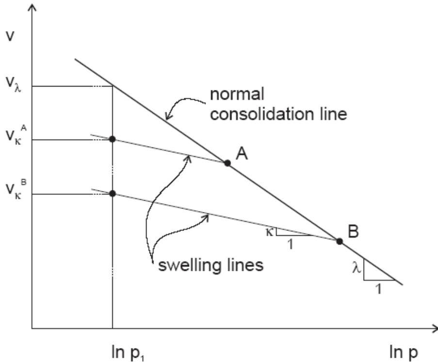
**Figure 2.24** Normal consolidation line and unloading-reloading (swelling) line for an isotropic compression test
