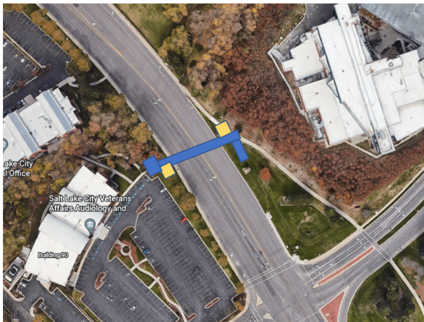
Figure 4.3 - Plan View of Single Span Bridge with Elevator and Stairs: Stairs are shown in blue while the elevators are in yellow [11].
