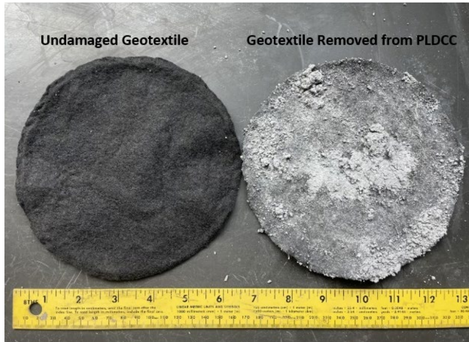
Figure 21. Undamaged Geotextile and Geotextile Removed from PLDCC
