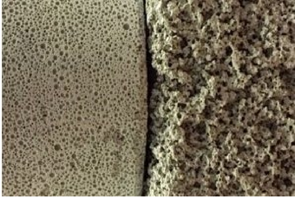
Figure 1. Comparison of the fabric and texture of LDCC (left) and PLDCC (right).
