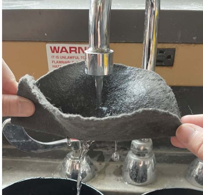
Figure 6. Water Infiltrating a Nonwoven Geotextile
