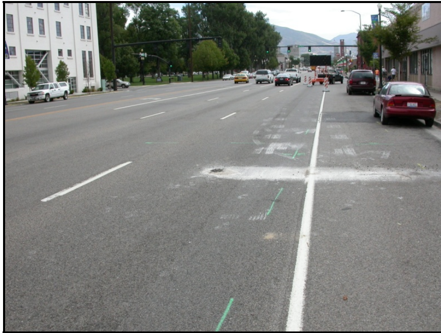
Figure 44- (CP-1) Demonstrates minimally invasive nature of the CPT
