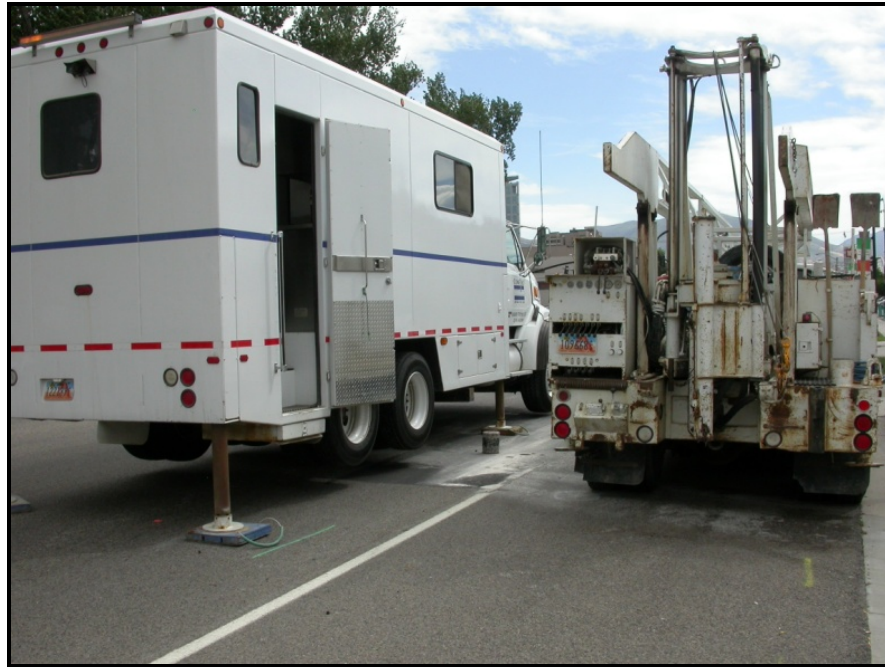
Figure 46 – (CP-7) 20-Ton CPT Rig and truck used to core asphalt and concrete
