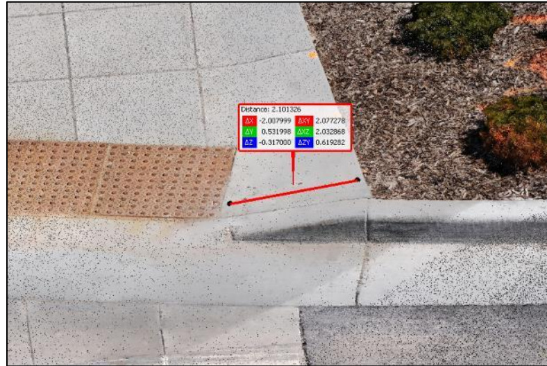
Figure 9 – Slope measurement of a flare component of a pedestrian access ramp. \Delta Z is the change in elevation, \Delta XY is the projected distance along the XY plane.
