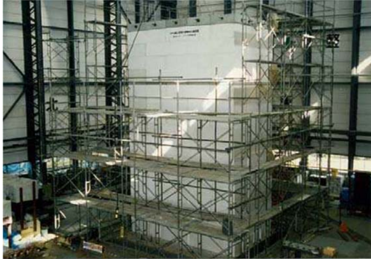
Fig. 25 Full scale seismic loading experiment on shaking table (EDO, Japan)
