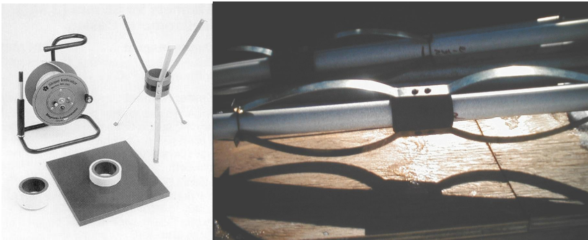
Figure F11. Magnet extensometer equipment. Tape reel (left). Spider magnet (right). Base plate magnet (left center middle).
